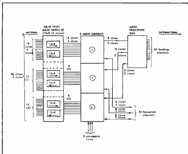
Block diagram of audio system at telephone (CIBA) center.
