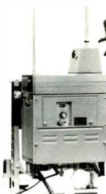
For microwave transmission from our HL-33 and HL-35 ENG cameras to a remote pickup point, we offer the Ikegami PF71 portable microwave relay system. This backpack unit transmits the video signal on the 13-GHz microwave band; audio and command signals on the 950-MHz uhf band. Maximum range is about 1800 feet with omni antenna, 3700 feet with 60-degree horn, two miles with a 20-degree horn.
