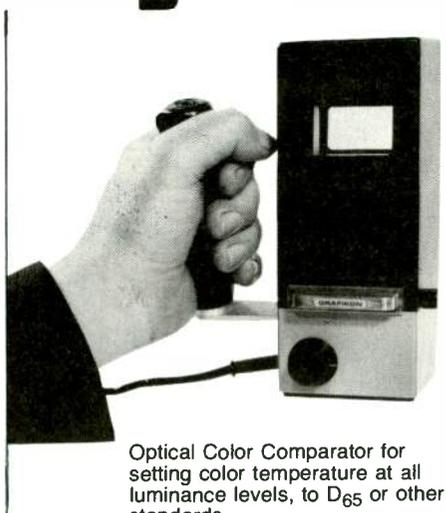
Optical Color Comparator for setting color temperature at all luminance levels, to D<sub>65</sub> or other standards.
