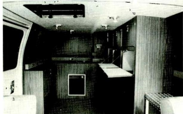
Another configuration for the interior reflects the intention to use the van as a production center. Wiremold is installed around the interior to provide a maximum number of power outlets since actual layout of equipment may change from day to day.
