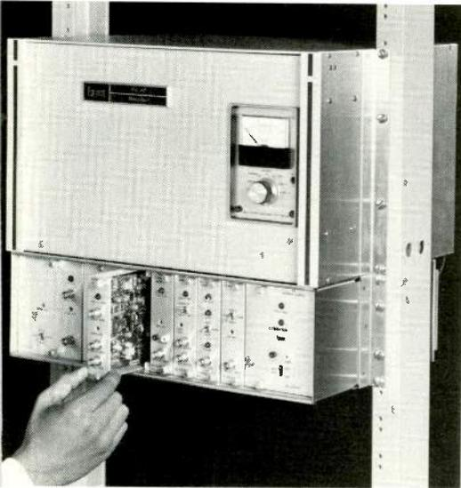
*FV4SR Terminal. System shown includes FV4F Receiver and FV45 Baseband Shelf.*
