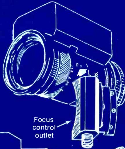
Accessory Focus Control outlet available to accept flexible cable for manual focus hand control.
