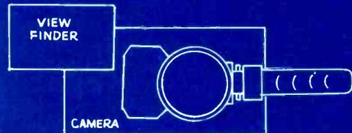
The camera can be placed on its side without interference from the lens.
