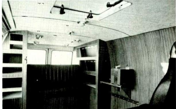
Interior of WGBH's field production van by Wolf Coach. This configuration reflects the intention of WGBH to use the van for remote recording. Because the van is used for remote production and not news, more room is provided for personnel.
