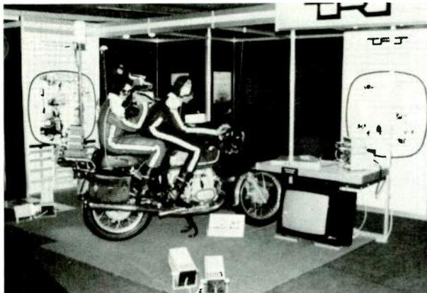
*This motorcycle, exhibited at Montreux, as part of the TRT display, is equipped with a 13GHz CP transmitter as well as camera equipment.*
