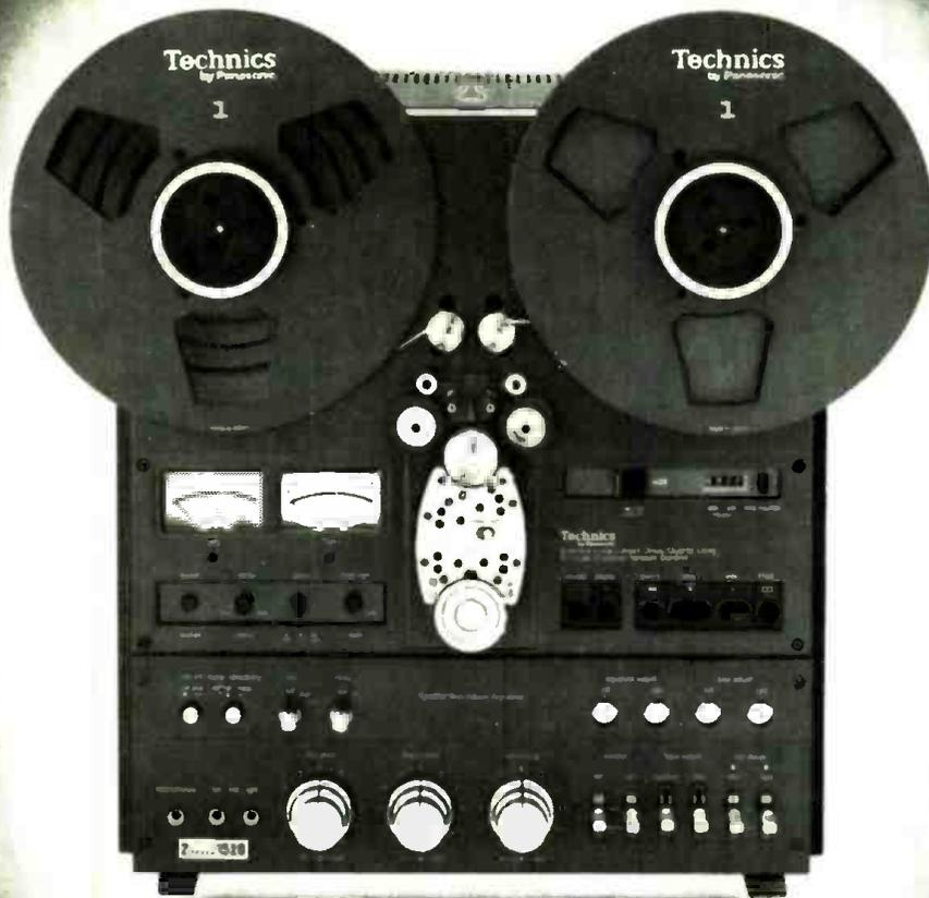
The RS-1520 has all the performance of the award-winning RS-1500 plus the features you need in a studio deck. Like bias and equalization fine adjustments for each channel to optimize any tape formula. A 1kHz/10kHz test-tone oscillator for accurate equipment checks. The precision of ASA standard VU meters with a +10dB sensitivity selector. A Cue/Edit switch for quick, safe edits. And balanced, low-impedance, XLR-type output connectors to match other widely used broadcast and studio equipment.
