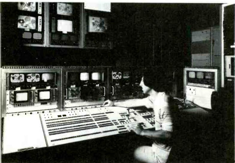
*TD at KCMO is truly "Mr. Video." Camera shading, quality control, switching, and master VTR machine control are all available at this console*
