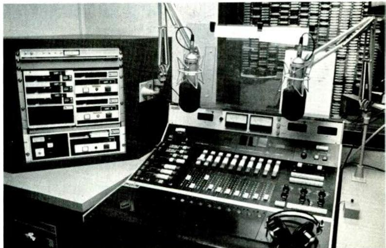
*WBEN's news control room, with master control visible through the window. News control is used to originate all newscasts and has its own cart and reel-to-reel decks, along with remote control to the AM automation sequencer*
