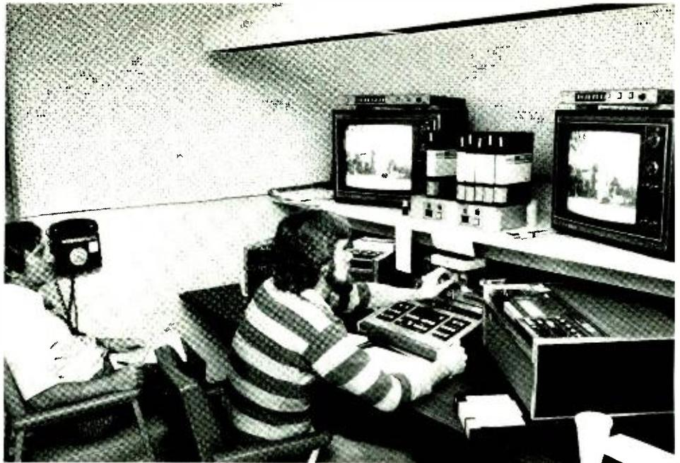
6:00 – 7:00 p.m., a half-hour from 11:00 – 11:30 p.m., and 10 minutes at 1:00 a.m. Four Convergence editors — two ECS-1s interfaced with Sony VO-2850s and two ECS-1Bs interfaced with Sony BVU-200s — handle the editing workload. One of the ECS-1B systems is assigned to the production area, but is frequently called into use for news starting around 4:00 in the afternoon when most of the tapes have arrived at the station. Each of the four editing systems gets at least five hours' use a day.
