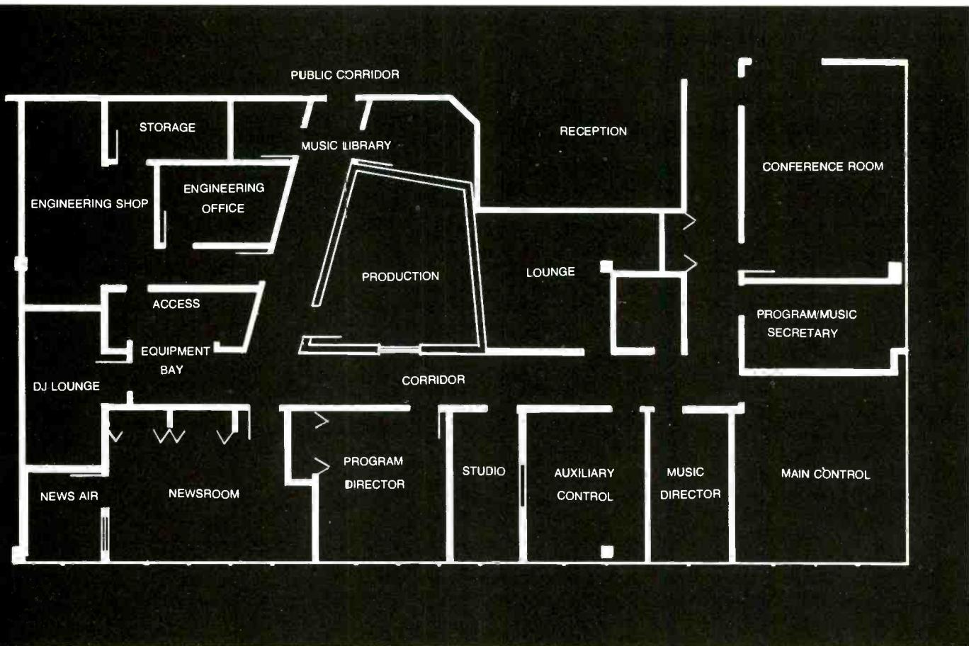
Floor plan of WDRQ. Four control positions are used
