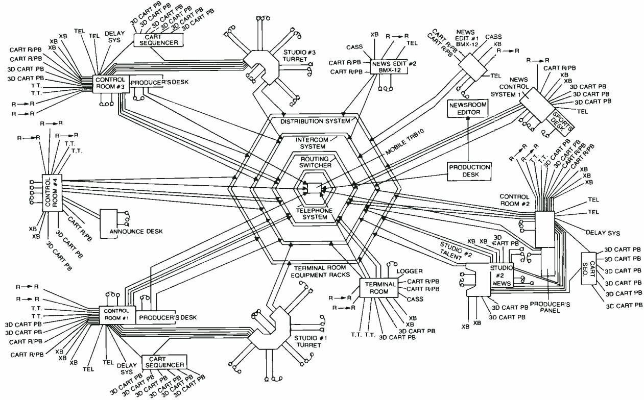
Interconnect plan (not a studio wiring diagram) shows every item of signal source and recording equipment connected to reach control position. Symbol XB is for the cross-bar switching system. Turntables are for music used on several "culture" programs, for interviews with music personalities, weekend music programs
