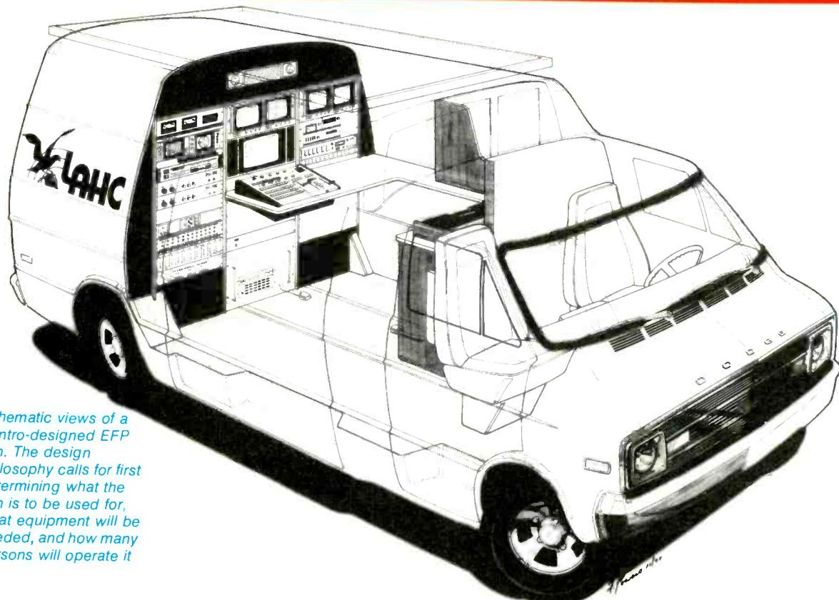
*Schematic views of a Centro-designed EFP van. The design philosophy calls for first determining what the van is to be used for, what equipment will be needed, and how many persons will operate it*
