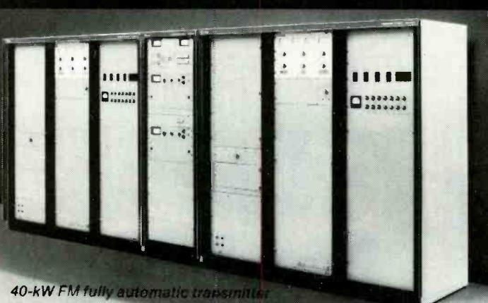
40-kW FM fully automatic transmitter
