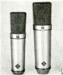
the others are hyper-cardioid (extra-narrow pickup angle at the expense of a small back lobe) and wide cardioid, described as "uni-directional." The U 89 has 10 transistors; sound pressure tolerance is up 12 dB from the U 87. There are two selectable low frequency roll-off curves, one at 80 Hz and one at 160 Hz. A 6 dB overload protection switch is also provided. GOTHAM AUDIO.
