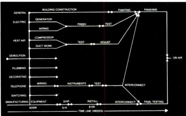
"PERT chart" is example of planning technique that allows different parts of complex job to be timed so that parts can be finished to allow others to start. Technique also allows detailed cost control and accurate scheduling of the job finish
