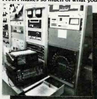
The Amber 4400A offers versatility and quality. Its features include sine, function, sweep, tone burst and noise generator; autoranging digital dBm meter and frequency counter; multimode filter; spectrum analyzer; frequency response and phase response plotter. High performance: low distortion and high output together with high measurement sensitivity and resolution.
