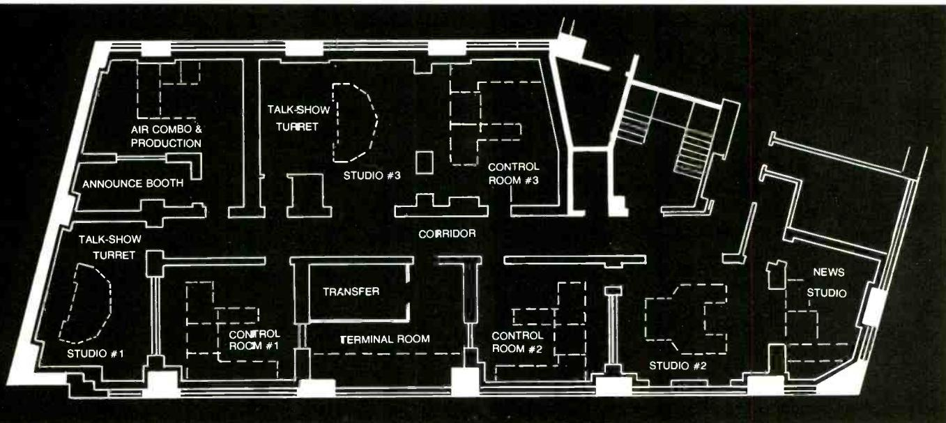
Floor plan shows how studios were laid out for mutual effectiveness. Studio 2, also in photo above, has adjoining room for control engineer when on-air talent requires one. Announce booth next to production room allows voice track to be added to commercials or other material
