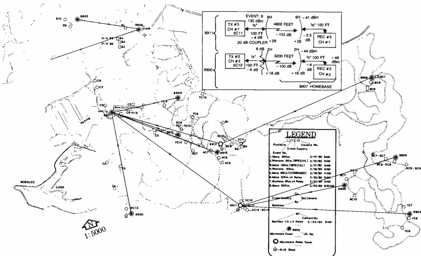
Coordination plan of extensive microwave relay system for cross-country and biathlon events at Mt. Van Hovenburg. Irregular terrain forced the use of 14 relay towers scattered throughout the courses, outfitted with a variety of H and V polarized dishes to enable channel agility on the 2 GHz band. Two snow cats, equipped with three cameras each multiplexed into a single feed, were moved about before the start of each race. Insert (top right) shows typical setup for cross-country event
