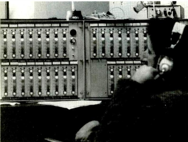
*Production coordination intercom system located in control room A. Operator-assisted, it linked 57 remote locations with six trunks handling up to 10 conversations per trunk*
