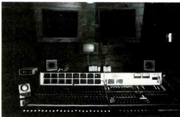
At the front of interior is the Ward-Beck console, which provides mixdown from up to 32 microphone inputs, or from the 16 tracks of Ampex recorder
