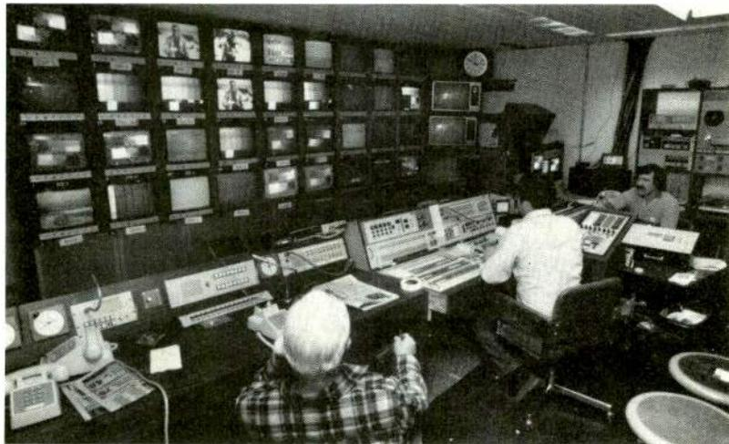
*Production control room B at broadcast center with Grass Valley 1600 7K switcher and Vital four-channel SqueeZoom. Audio position, identical to control room A, had Ampex reel-to-reel and ITC cart decks*
