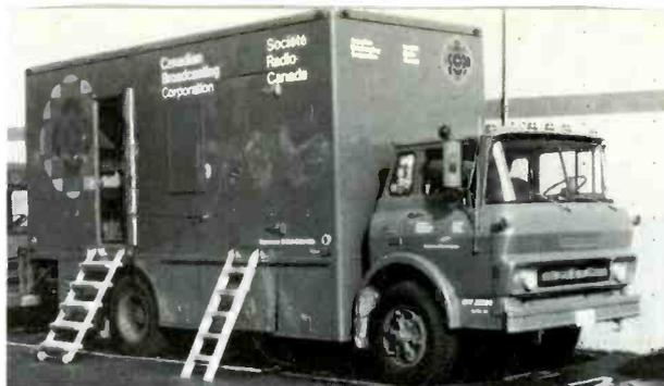
Close view of van shows entries and comparatively high ceiling, put to use in the acoustical design so that monitoring of mixdown balances will be proper
