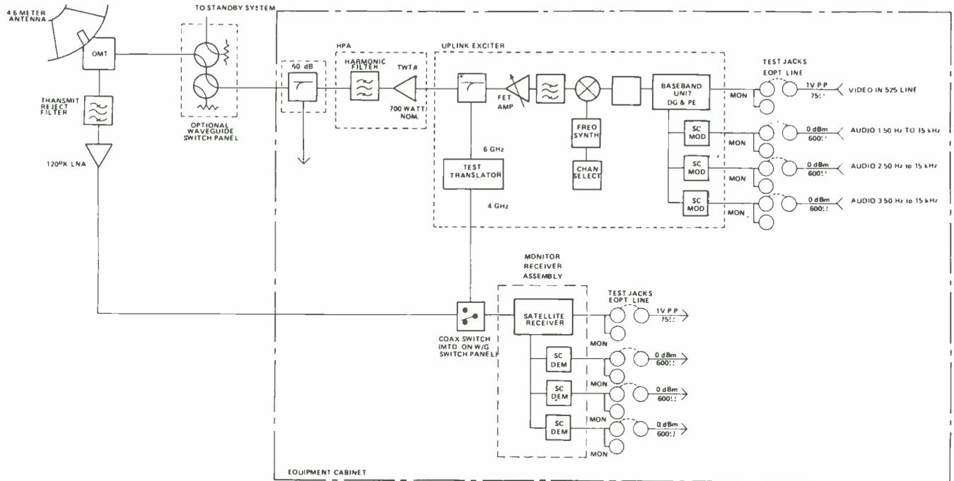
Schematic of Satellink's "Flying Saucer." Unit provides both transmit and receive capability in an unusually compact package for radio and television
