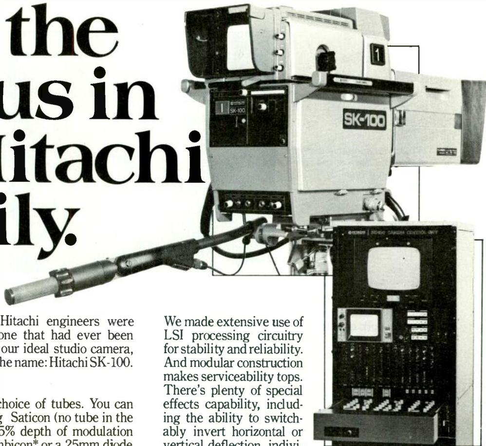
We made extensive use of LSI processing circuitry for stability and reliability. And modular construction makes serviceability tops. There's plenty of special effects capability, including the ability to switchably invert horizontal or vertical deflection, individually or together, and to invert the RGB signal polarity. The DCU/triax option allows you to remote control the SK-100 from up to a mile away.
