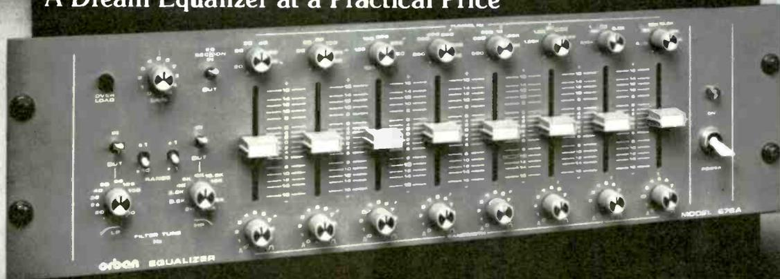
The 672A is a single-channel equalizer offering astonishing control and versatility. There are eight non-interacting parametric bands with reciprocal curves and the convenience of graphic-style controls. Highpass and lowpass filters with 12dB/octave slopes that tune continuously over a 100:1 frequency range. And, separate outputs that let you use the 672A as an eight-band parametric cascaded with an electronic crossover in reinforcement and monitor tuning applications.
