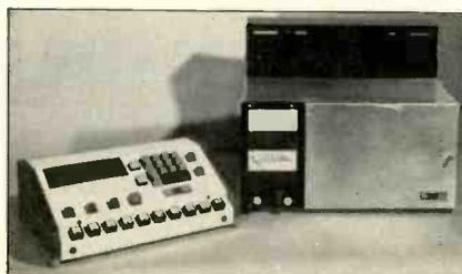
10 audio sources. The 10 source START buttons are lighted as long as that source is on the air. Other features include adjustable monitoring facilities, simple user installation via terminal strips for each channel connection, low-cost optional relay, and adjustable time delay silence sense action, which allows for automatic program advance if desired. Frequency response is  $\pm 1$  dB 50 Hz to 16 kHz; THD is under one percent at +8 dBm. \$3995. SONO-MAG CORP.
