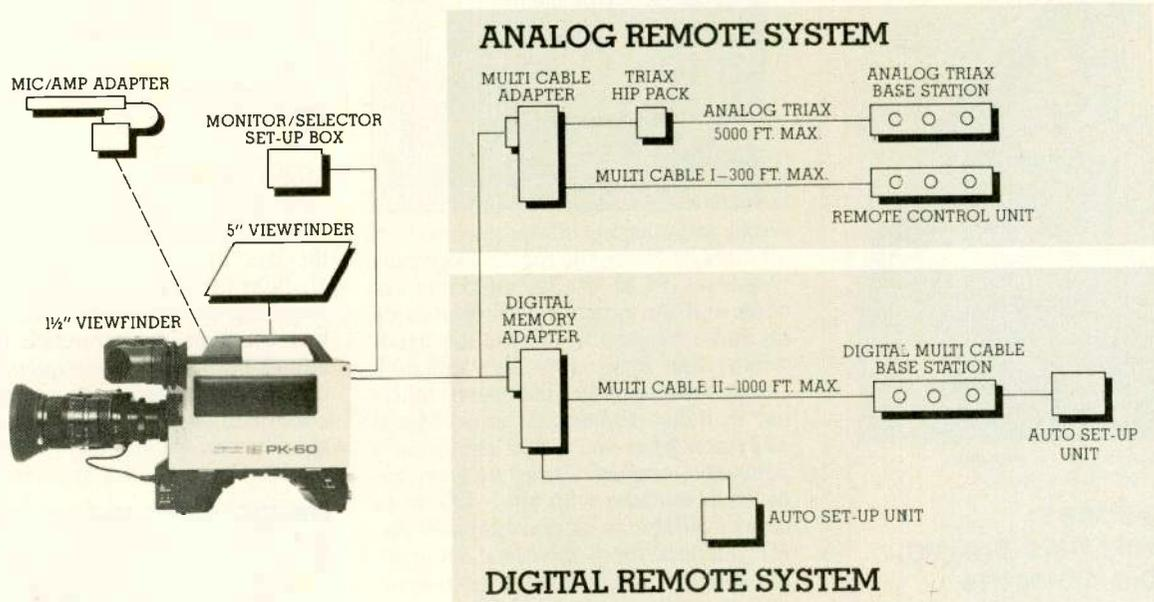
Introducing Toshiba's PK-60 ENG/EFP Color Camera. These drawings tell the story of the camera's digital and analog modularity. It features a separate digital memory with an internal microprocessor, an automatic setup unit with an 8-bit microprocessor, a digital base station and triax/wireless transmission with base station. The monitors also detail the PK-60's very modest dimensions.
