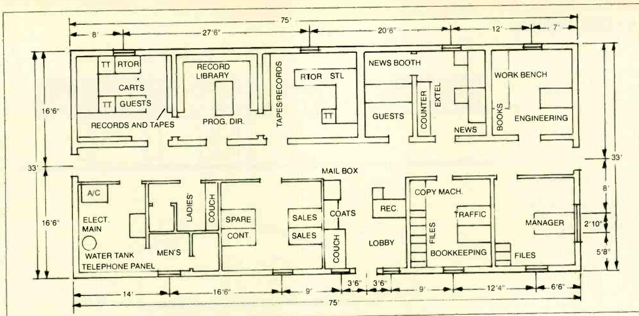
Standard floor plan is 75 feet by 33 feet, and provides space for all operational needs of a small to medium-sized radio station. The transmitter will be in an adjoining accessory building or at a remote location. The standard plan can be enlarged by adding length (see plan below) or by adding one or more wings. Interior, too, can be altered
