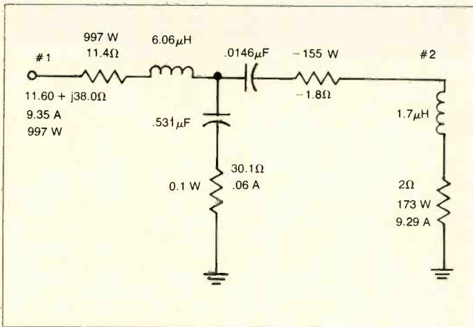
Fig. 5. Input power is 1015 W
