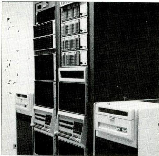
*The two switching computers for the CBS Radio Net, one a hot standby, are the two side-by-side units with piano-key controls in lower half of racks. Disc memories flank racks; interfaces to crosspoints are on cards high in right rack*
