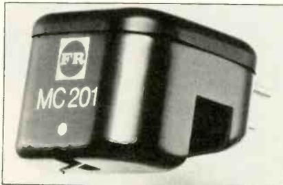
other MC cartridges. Specs include a 0.3 by two mil line contact solid diamond stylus, with a 0.16 mV rms at 5 cm/sec/1 kHz and 0.12 mV peak at 3.54 cm/sec/1 kHz output voltage. Coil impedance is 8 ohms  $\pm 1.3$  ohms at 1 kHz, load impedance is 10 ohms or higher, and total cartridge weight is 7.5 gm  $\pm 0.3$  gm. \$325. FIDELITY RESEARCH.
