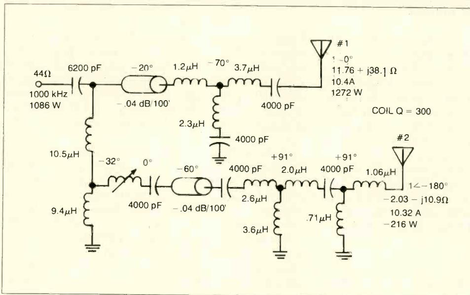
Fig. 2. The negative tower's coupler must present the negative of the operating base impedance to the tower
