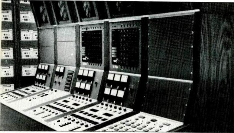
Manual control position for CBS switching system has CRT readouts (top) to show upcoming events; NetALERT transmitters above VU meters; and a full set of pushbuttons so operator can take over switching from computer, if necessary
