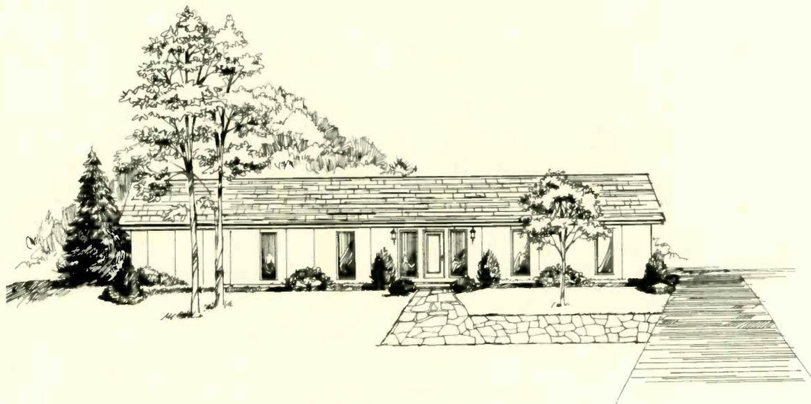
*One of exteriors available with standard Grinnan prefabricated broadcast station building is shown in the drawing above. The exterior walls can be lapped siding, brick veneer, brick, stucco, plywood panels, or others. The roof can be gabled (as shown) or flat, with one side of the roof covered with acrylic plastic if solar heating is chosen*
