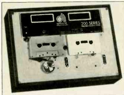
lows a cassette duplicator to precisely measure the master and make the duplicating blank tapes to the exact length required. A unique leader sensing element shuts the unit down before the leader runs out, permitting the rewriter to run tapes at very high speed. In the exerciser mode, the unit winds and re-
