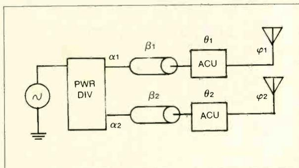
Fig. 1. Power flow is from the negative tower back to the power divider
