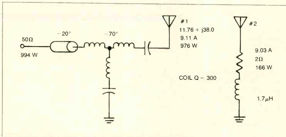
Fig. 3. In theory, the coupler could be replaced by a resistor and a coil
