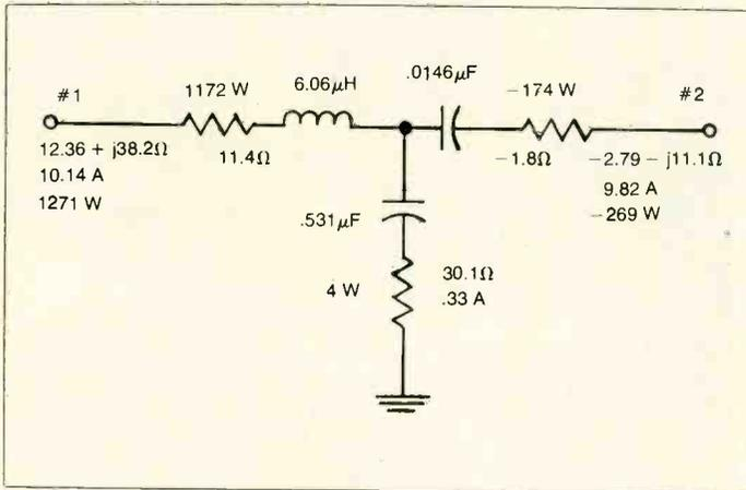
Fig. 4. Input power is 1002 W
