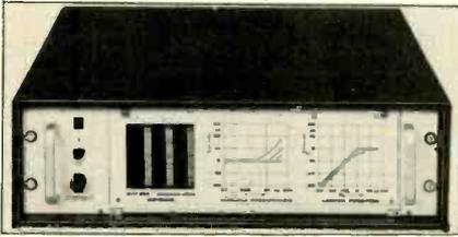
cuitry to calculate the gain reduction required for each transient before it arrives, eliminating transient overshoots. The unit's "adaptive preemphasis" circuit further processes this limited signal via a variable time constant filter to control high-frequency signals that would otherwise cause overmodulation. Rack-mountable, the limiter is intended for hands-off operation. GOTHAM AUDIO CORP.
