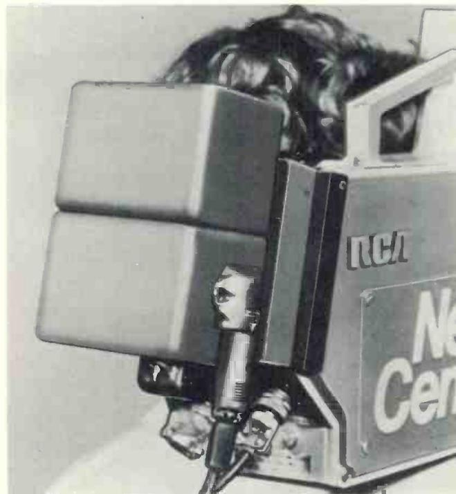
The on-board nicad by Alexander is hooked to an RCA video camera.
