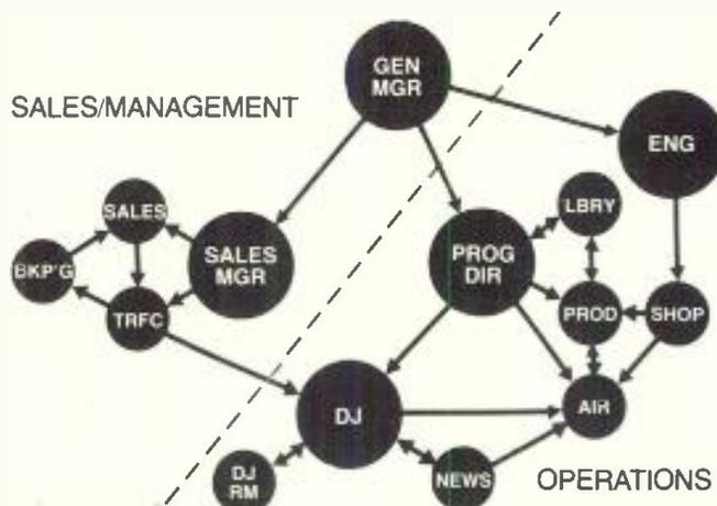
A flow chart of station functions used to define space allocations.
