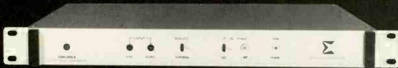
If SC/H Phase is critical to you, then be critical . . . Specify SIGMA SYNC GENERATORS. Both Models CSG-360A and CSG-365A lock horizontal directly to subcarrier so you can be sure it is in the proper place, all the time . . . even resets the phase on power up.
