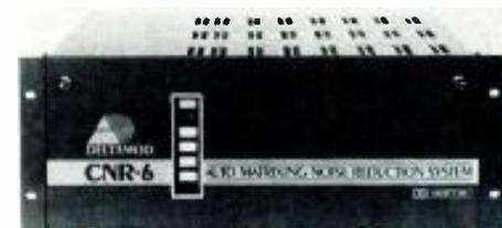
After initial calibration, the CNR-6 automatically switches matrix noise reduction in or out. Carts recorded with noise reduction are automatically cue-track encoded. If the noise reduction is switched off, there is no encoding and no cue tones of cart machines are sacrificed. The unit accepts up to six stereo encode or decode modules with additional space for a bypass card. This noise reduction unit is also suitable for video recorders.
