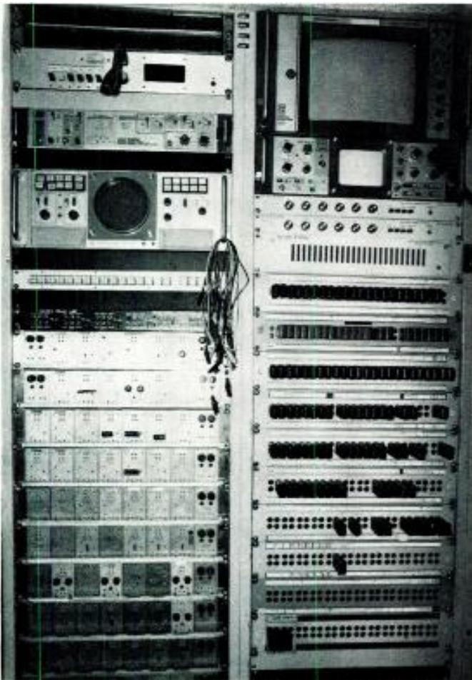
*Sync rack in NEP's SuperShooter II truck holds Tektronix 850 matrix monitor, 149A NTSC test signal generator, Type 520 NTSC vectorscope, and 1480R waveform monitor; Microtime delay line; and Fernseh TVP-1000 video proc amp and RC-1000 processor remote control units.*
