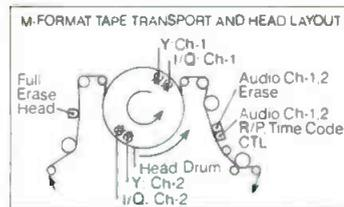
dubbing or insert and assembly editing. At the same time, two rotary erase heads and vertical head switching make for clean, accurate edits.
