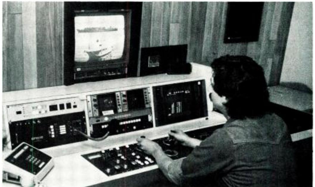
Mark III, the FDL-60A also uses a capstan drive and transfers images from the film while it is in continuous motion. The capstan drive has completely dispelled early fears about potential original film damage.
