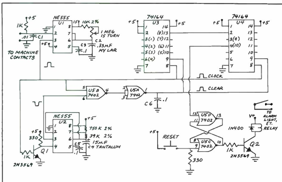
U2. Since U2 goes low when reset, U5B prevents it from resetting U3 and U4. U5A is used as an inverter.
