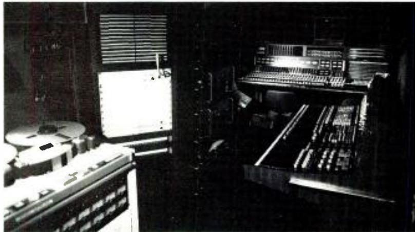
The control room of WGBH's Unit 4 audio control facility features a custom 40x24 API mixing system that provides simultaneous 24-track, stereo, and mono mixes. Outboard equipment includes eight dbx 903 compressor/limiters, dbx 162 stereo program compressor, Lexicon 224 digital reverb system, and two Lexicon PCM 41 DDL effects units. Otari MTR-90 24-track recorder is seen in foreground.
