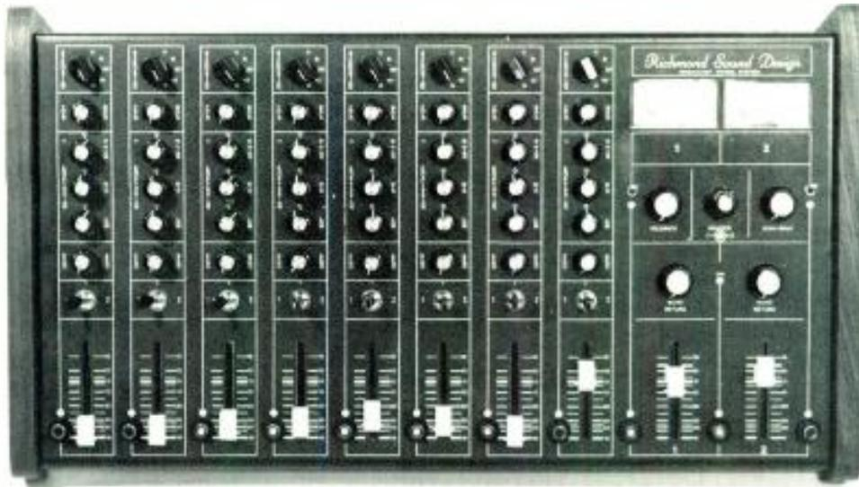
Richmond Sound Design's Model M82B broadcast audio control console features production and on-air capabilities with transformerless inputs, equalization, and complete monitoring facilities. A calibrated attenuation switch is offered, selecting mic input on 0, 10, and 20; line inputs are on A and B positions respectively. Three-band equalization is included with a wide adjustment range, continuously variable boost/cut, and active filter design.
