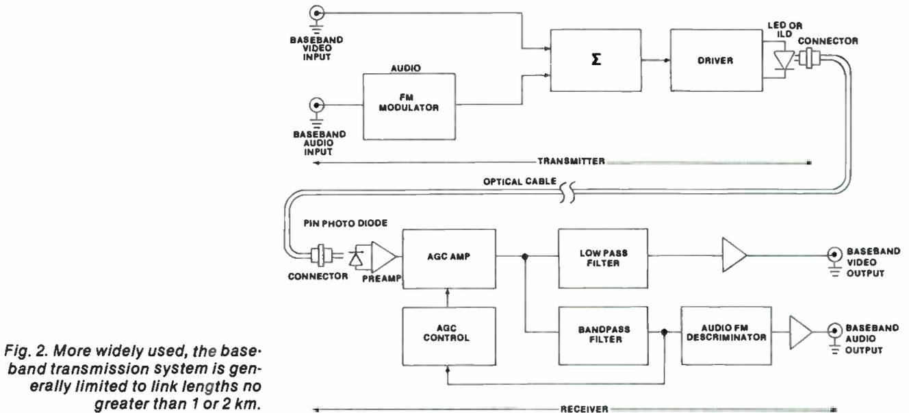
Fig. 2. More widely used, the baseband transmission system is generally limited to link lengths no greater than 1 or 2 km.
