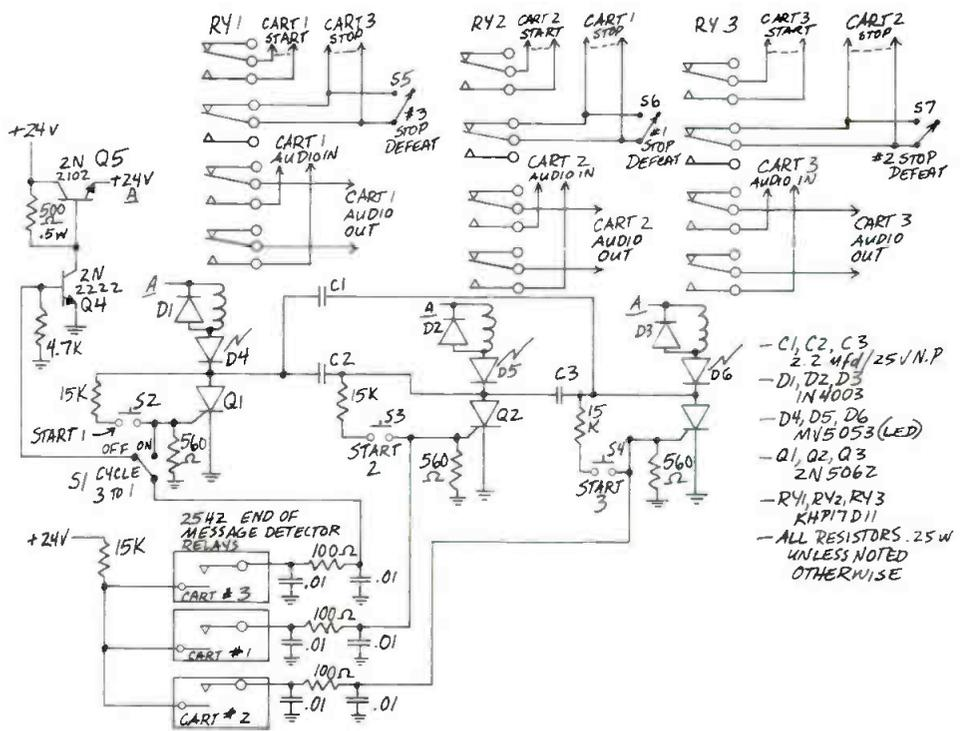
using one pair of relay contacts to switch the audio line, the machine with the cartridge recuing can be muted.
