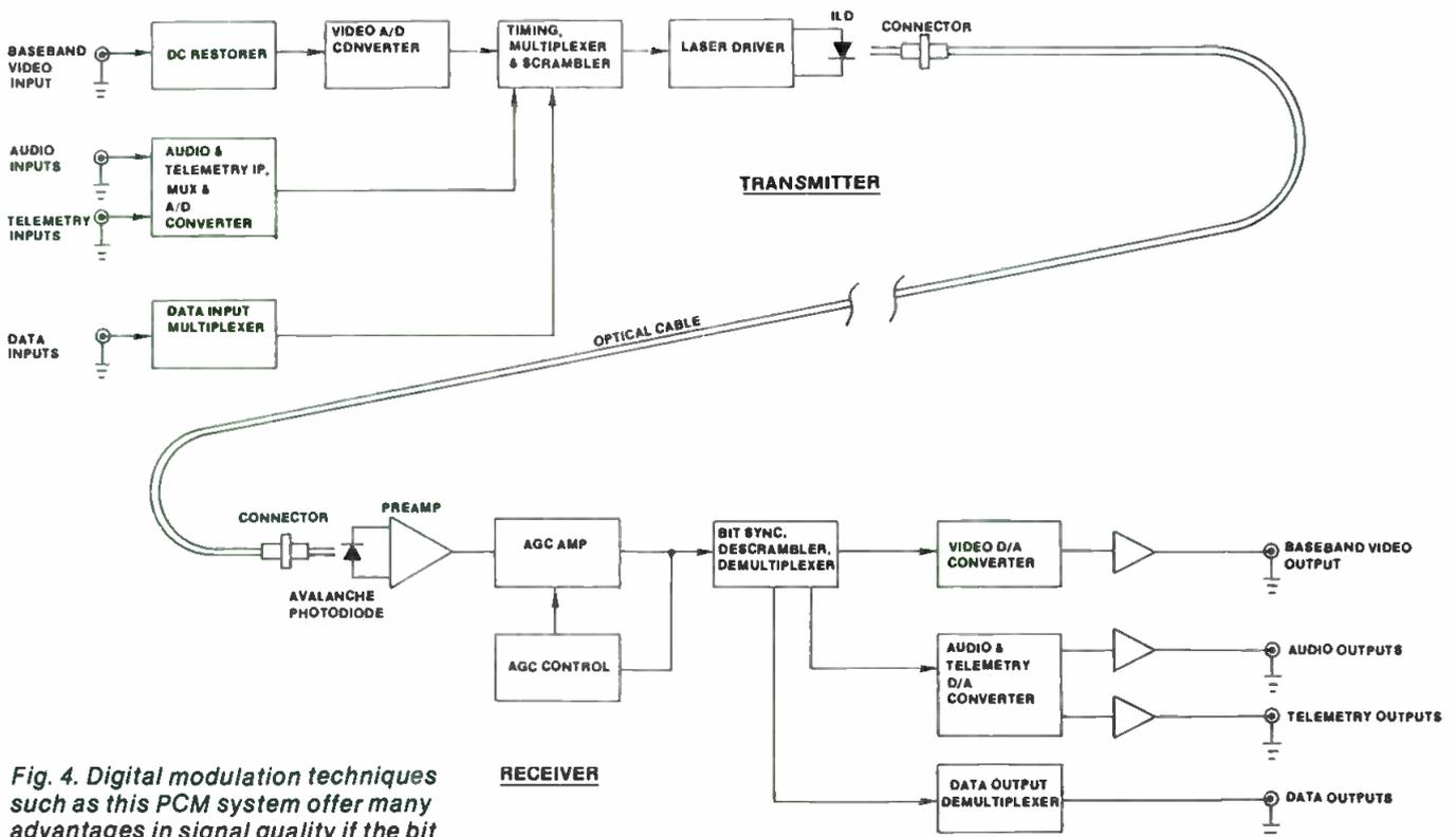
Fig. 4. Digital modulation techniques such as this PCM system offer many advantages in signal quality if the bit rate is reduced and coding used.
