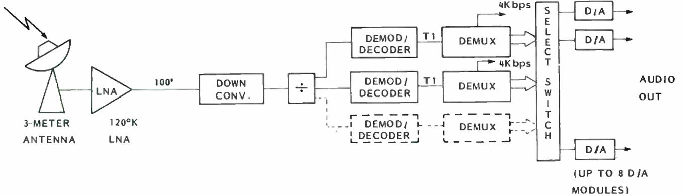
Receive-only earth station block diagram.
