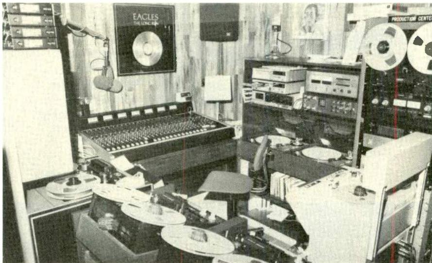
Hubbard's small but well-equipped production room in San Ramon, CA, has an Audio Arts console and Otari ATRs. Sony CD players are visible just above the turntables.
