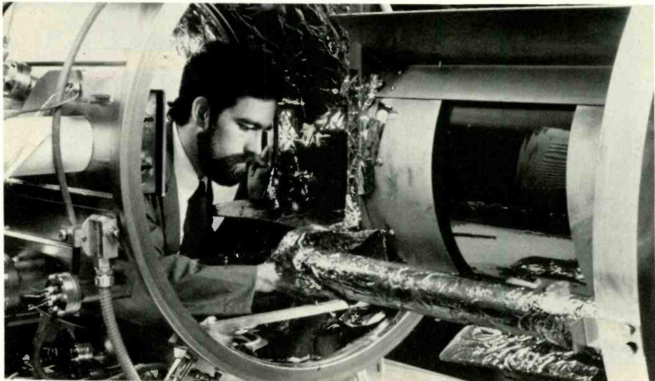
Vacuum chamber used to produce thin film coatings is readied by a 3M physicist.
