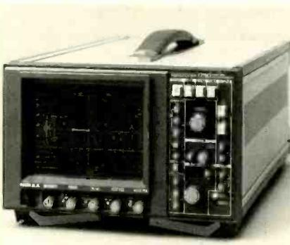
*The Tektronix 1750 waveform monitor/vectorscope.*
