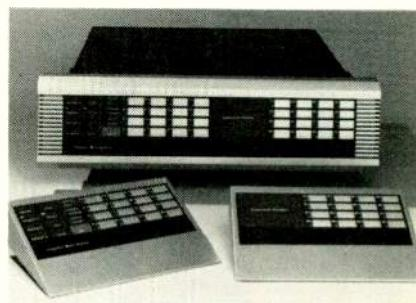
The Model 200 Smart Switcher is a new audio routing/mixing system from Integrated Media Systems. It is configurable in matrixes of eight, such as 32×8, 8×32, 16×16, and so forth, in one 5.25-inch frame including power supply. The matrix configuration can contain up to 256 crosspoints per frame, and it can be expanded up to 128×128, with up to 32 control stations.
