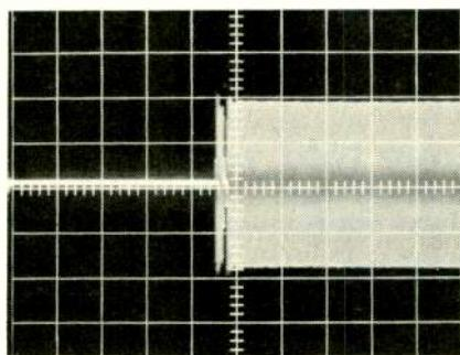
Fig. 2 Cue output with air dashpot set for 90 ms. start delay (Sweep = 20 ms./div.)
