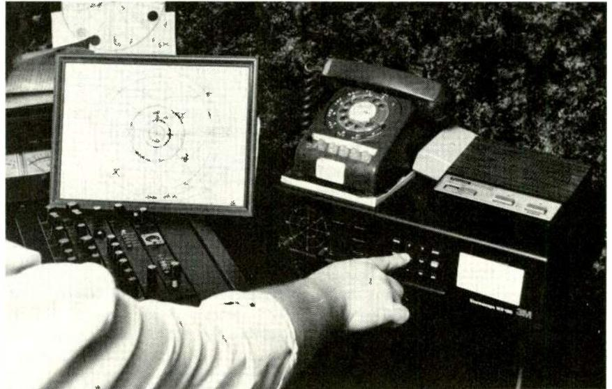
*The thunderstorm-tracking instrument superimposes a weather mapping grid, which corresponds to a grid on the Stormscope CRT, over a local highway map.*
