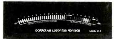
LEDs at the two maximum points allow the operator to adjust levels up. Equal loudness is achieved by riding maximum gain to these points of reference as the program dictates.
