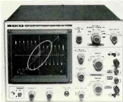
A stereoscope like that above can be used to check channels switched together before a stereo program is put on the air. A pattern like the oval seen indicates a phase difference that must be analyzed and corrected.
