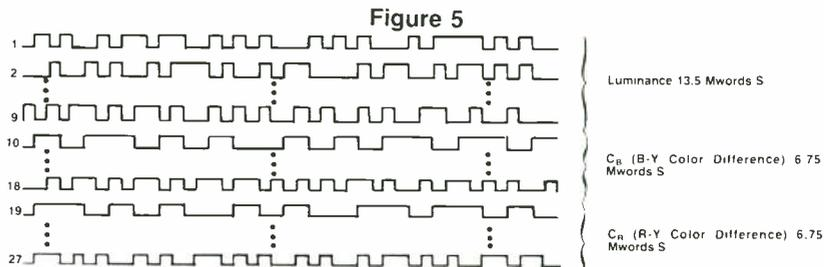
Figure 5 results from digitizing the signals from Figure 2 and sending them down eight pairs for each signal—a total of 24 pairs carrying signal data. Each group includes a ninth pair for a reference and timing signal. All 24 bits are sent in parallel, while words representing sample locations are sent serially through the 27 total pairs. The data rates are 13.5 Mwords/s for the luminance group and 6.75 Mwords/s for each color difference group.
