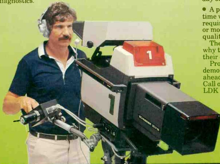
The LDK 6 total computer control system, one bus architecture allows physically locating the small master control panel at the camera head or CPU. This permits one technician vs two to maintain the system.
