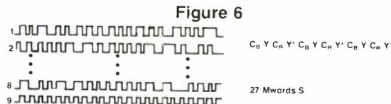
Figure 6 results from multiplexing of the data from Figure 5 by alternating between luminance and color difference data. Nine pairs are required: eight for data, which now include the timing signals in the data stream, and the ninth for a clock signal. The order of transmission of data is shown, with the Y\* representing luminance samples with no corresponding color difference samples. The other luminance and the two color difference samples are all co-sited.
