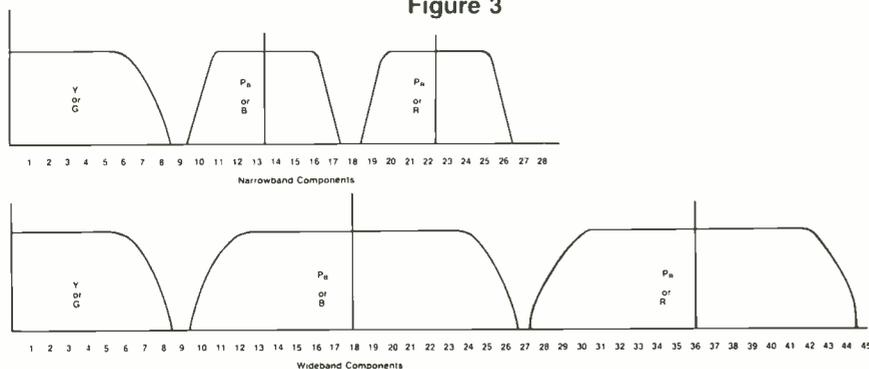
Figure 3. Spectra of frequency division multiplex (FDM) schemes in both narrowband and wideband forms. Luminance or green is carried in baseband. The other components are modulated on carriers. Amplitude modulation is shown because it minimizes bandwidth. Frequency modulation would yield better performance and would be preferable, but it would increase the bandwidth.
