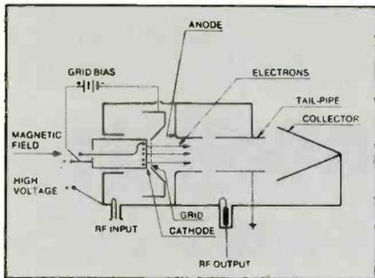
Figure 2 shows the structure of the Klystrode, which combines the features of a klystron and a tetrode.
