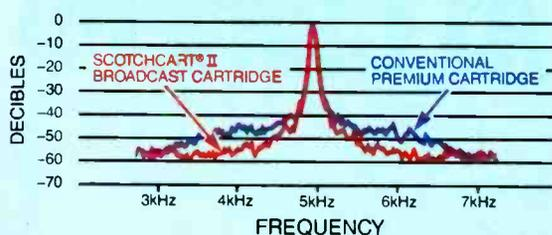
The Revolutionary ScotchCart® II broadcast cartridge design eliminates the excessive audio sideband noise which results from the rubbing effects of pressure pads and the mechanical irregularities of rotating hubs found in conventional cartridge designs.
