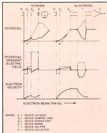
Figure 1 shows the potential, potential gradient and electron velocity vs. beam distance, for a tetrode and a Klystrode. In the top two drawings, the solid line indicates the tube characteristics at minimum conduction and the broken line shows the tube at maximum conduction.
