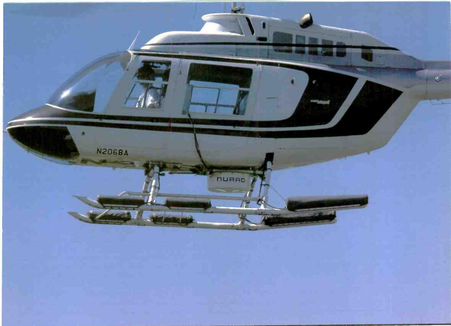
**SUPER POD™** (sōō' pər pod) *noun* 1. A microwave transmit/relay system used with ENG helicopters: enhances and extends the coverage capabilities of television news departments. 2. Nurad's advanced airborne ENG system featuring an automatically rotated transmit antenna; incorporates a sophisticated Loran C control system.
