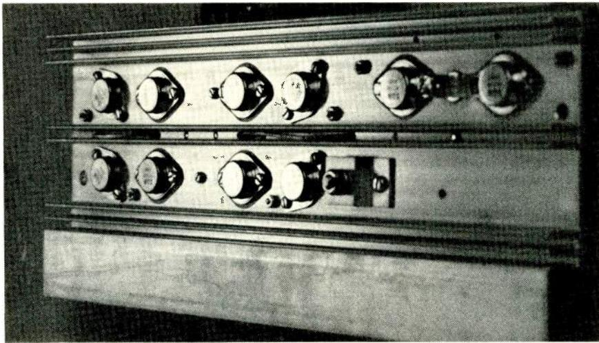
Metal Oxide Semi-Conductor Field Effect Transistors, or MOSFETS, have made solid-state AM transmission up to 50 kW possible.
