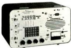
The RG-4 combines high level output (10 VRMS) capacity with a sensitive receiver (5 micro V) and more than 120 dB receiver/generator isolation.
