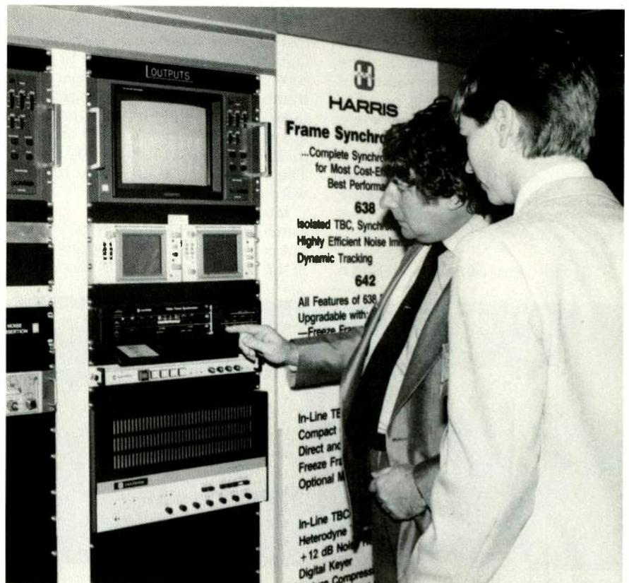
The new Harris model 642f frame synchronizer/time base corrector features up to 12 dB of Smart Noise Reduction that is automatically applied to the amount of noise measured in the video.
