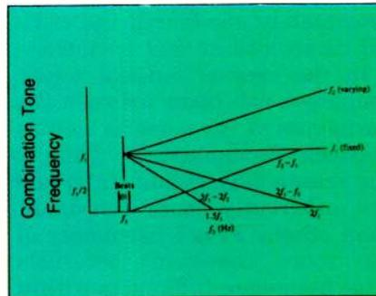
**Figure 3:** Most influential combination tones for a two-tone presentation consisting of one fixed frequency  $f_1$  and one of variable frequency  $f_2$ .
