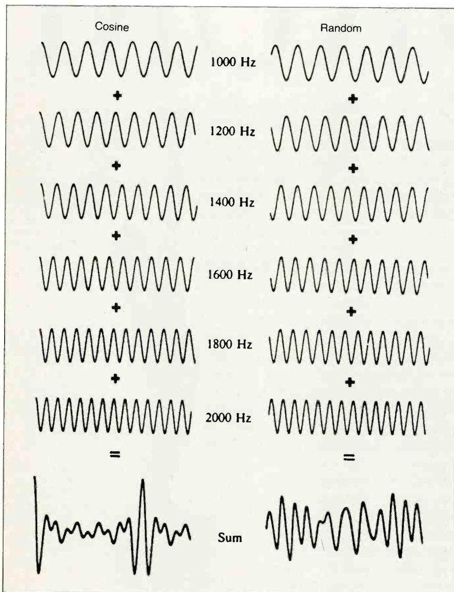
**Figure 6:** Changes in relative phases of components can change the waveform itself.
