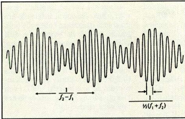
**Figure 1:** Waveform with beats due to pure tones with frequencies  $f_1$  and  $f_2 = f_1 + df$ .
