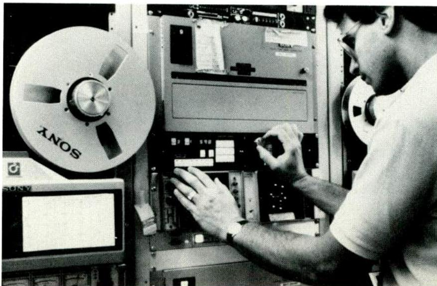
The Zaxcom multiple time base corrector remote control system installed at New York's Broadway Video includes control panels in the machine room (seen here) and in the edit suites.
