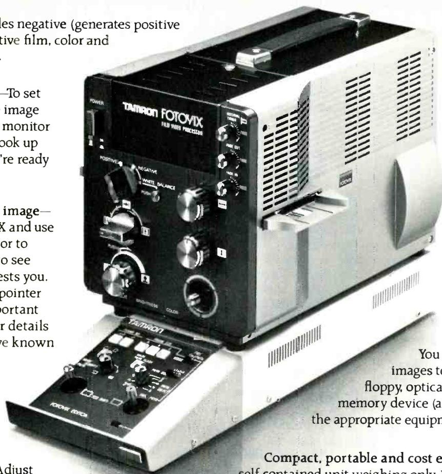
**Genlock**—Fotovix Pro's Genlock capability lets you integrate and review multiple images on a single monitor by use of an SEG (Special Effect Generator) or a switcher.
