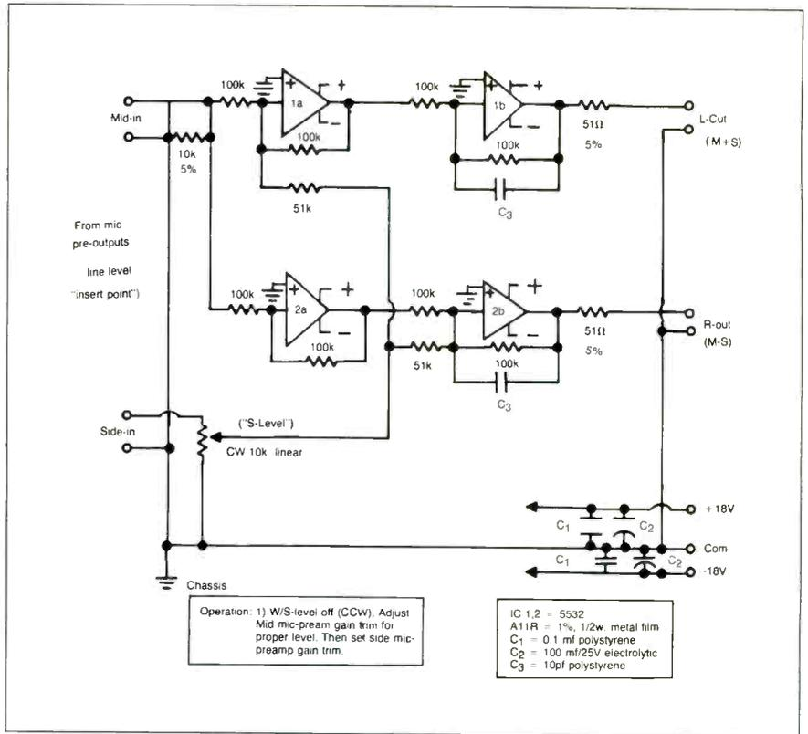
Figure 2: Active, line-level M-S matrix (unbalanced).
