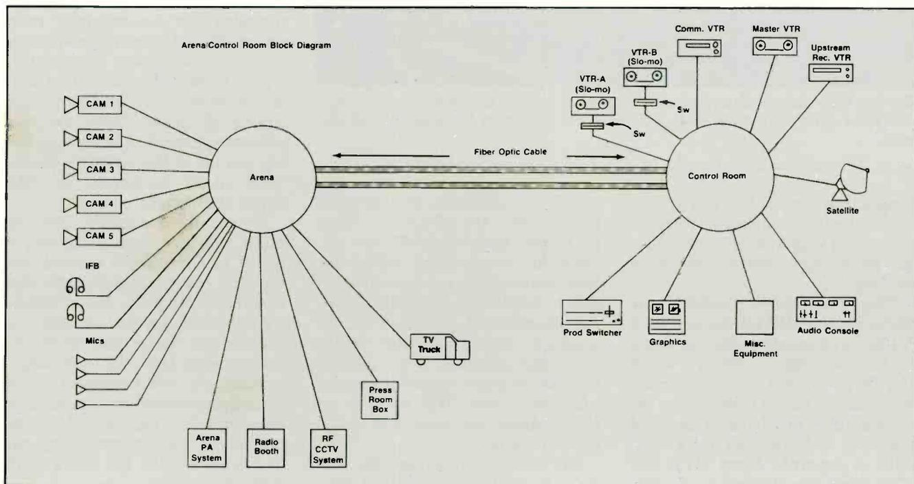
Figure 2: Full arena-to-control room block diagram.
