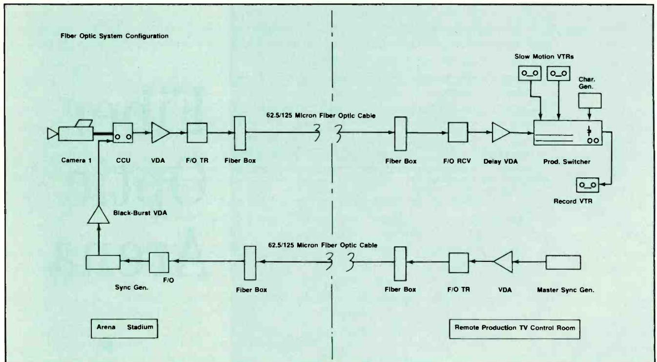
Figure 1: Simplified arena-to-control room design scheme.
