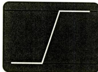
Figure 2: To create wipe patterns in a switcher, a waveform generator produces the control signal. Here a simple vertical split screen with soft edge is created by providing a ramp with a short risetime. Edge softness is adjusted by increasing or decreasing the risetime of the ramp signal. For a soft-bordered wipe, two ramps, offset in time, would create transitions from A to matte and from matte to B.
