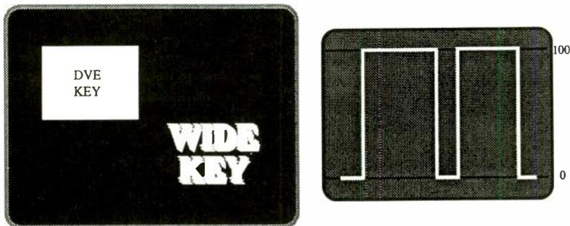
Figure 4: When "all" of a picture must be inserted into another picture, as is the case with a digital effects system or a character generator that produces its own edge enhancements, the external device must tell the video mixer where to insert the video. These devices typically have a "TTL" level key signal (either 0 or 100 with very fast risetimes). This type of key signal only produces sharp edges.
