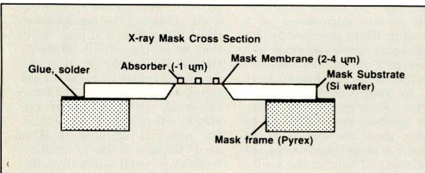
*Schematic cross-section through an x-ray mask.*
