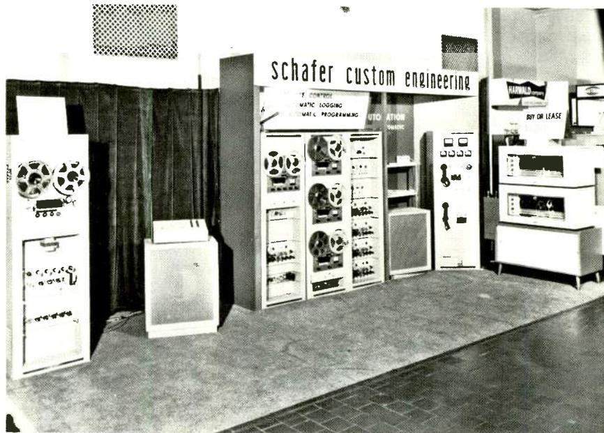
*The original Schafer Automation System, the Model 60, known as the "blue wire job," on display at the 1959 NAB convention. Concert One reel-to-reel decks were wired to two Seeburg juke boxes that played 45 rpm records. Also, the first spotter machine, with an Ampex deck, which ran re-wind and fast forward to locate commercials. Schafer: "It took at least 100 clip leads to make it work at the convention."*
