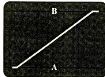
Figure 1: The video mixer is a proportional device that blends two pictures together based on the level of the control signal. If the control signal is at 0, only source A is allowed through to the output; a 100, only source B is output. At any value in between, a proportional mix of the two sources is output. The ramp signal changes from 0 to 100 at horizontal line rate (a rise time of 63.55  $\mu$ s).
