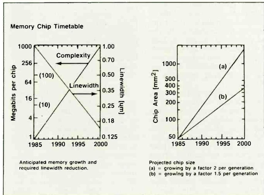
Timetable for memory chip production. (All diagrams developed by A. Heuberger, Fraunhofer-Institut für Mikrostrukturtechnik, Berlin, Germany and Technische Universität Berlin, Germany.)
