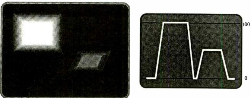
Figure 6: When a digital effects system goes the extra mile and provides a linear key output, a number of exciting effects are possible: The edges of the compressed images can be softened, or soft color borders can be added; and shadows can be cast on the background. The important factor to remember for any linear key is that the control signal should be softened or antialiased, but the video fill must not be similarly processed; it must extend just past the edge of the softened effect.
