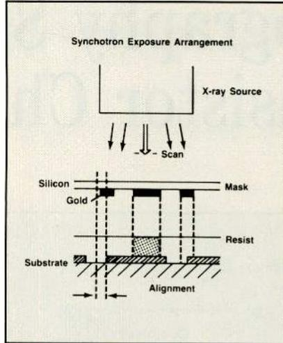
*Exposure arrangement for x-ray lithography using synchrotron radiation.*
