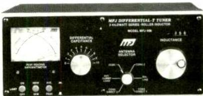
of two variable capacitors. The new MFJ-986 covers 1.8 to 30 MHz continuously, including MARS and all the WARC bands. The differential capacitor makes tuning easy and fool-proof because minimum SWR can occur at only one setting. Roller induction allows a very low SWR. A lighted two-color peak and average reading cross-needle SWR/Wattmeter indicates forward and reflected power and SWR. Comes with one-year guarantee and sells for \$239.95. **Reader Service #213**
