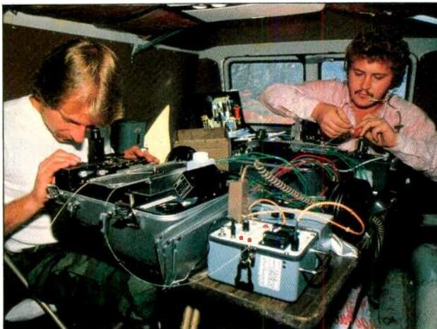
Technicians at the Corning Glass Works using an arc-fusion splicer to join heterogeneous single-mode fibers without excessive signal loss. A single universal setting is used for all fiber optic splices.
