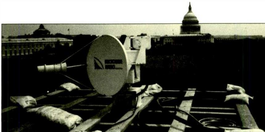
*Nurad's Silhouette microwave antennas are widely used for ENG applications (opposite). Microwave Radio's 2/7/13 GHz central receive system.*
