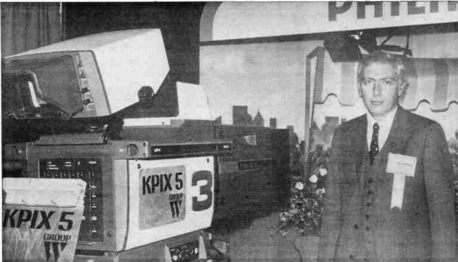
L. Merle Thomas of Group W's WJZ-TV, Baltimore, and SMPTE's vice president for television affairs, stands with a Philips LDK-6 microcomputer-controlled camera now owned by sister station KPIX-TV in San Francisco. Group W bought eight of the cameras for the two sister stations.
