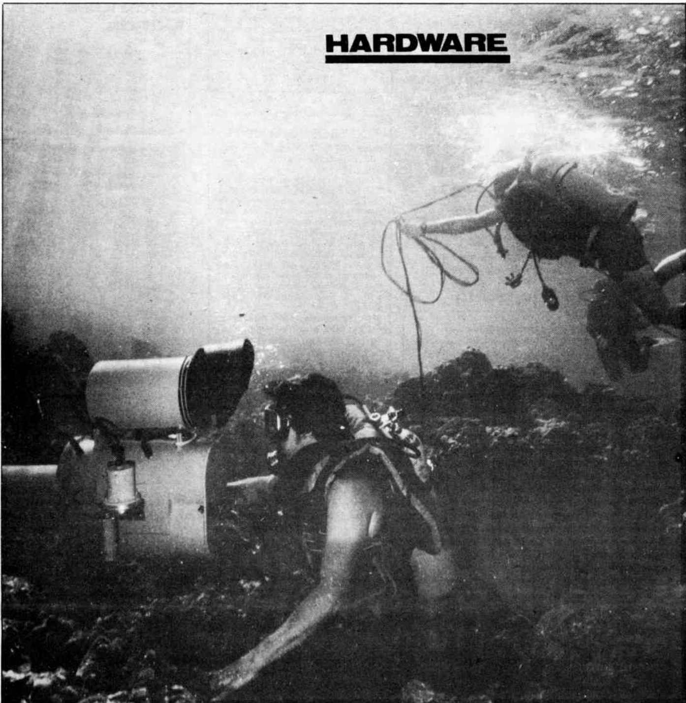
Sony's new underwater videotape housing is designed for its BVP-330 color camera and BVF-5 viewfinder.
