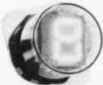
The RCA end view NUMITRON is a 7 segment incandescent readout tube, with a character height of 5/8". It requires a 9 pin Novar socket, which we furnish with each tube. The tube operates at a nominal voltage of 4.5v, and draws 24 ma. per segment. It can be filtered to any color. With data.
