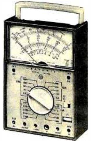
c. A multimeter. This all around useful test instrument can be built from a kit and later used to measure miscellaneous voltages, current and resistance when diagnosing or using the hardware of a computer and its interfaces.
