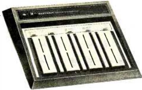
a. A prototyping breadboard. In computer applications, such a breadboard can be used to temporarily try out a circuit before committing it to permanent form using wires, sockets, Vectorboard and solder or wire wrap. Power supplies at standard logic (+5 V) and typical analog ( $\pm 12$  V) levels aid prototyping with this unit.
