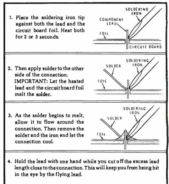
**Be sure the solder made a good electrical connection.** When both the lead and the circuit board foil are heated at the same time, the solder will flow onto the lead and the foil evenly. See illustration A. The solder will then make a good electrical connection between the lead and the foil.
