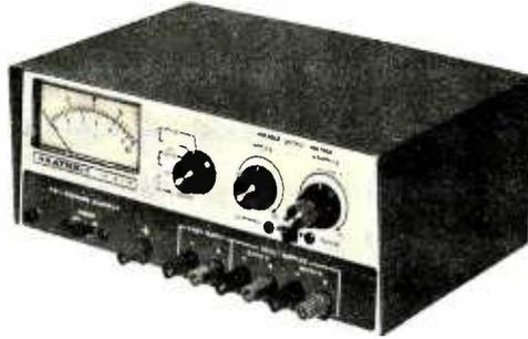
b. A laboratory bench power supply. Once built, this instrument is used to simultaneously power logic (+5 V) and provide variable metered analog levels from  $\pm 0$  to  $\pm 20$  V.
