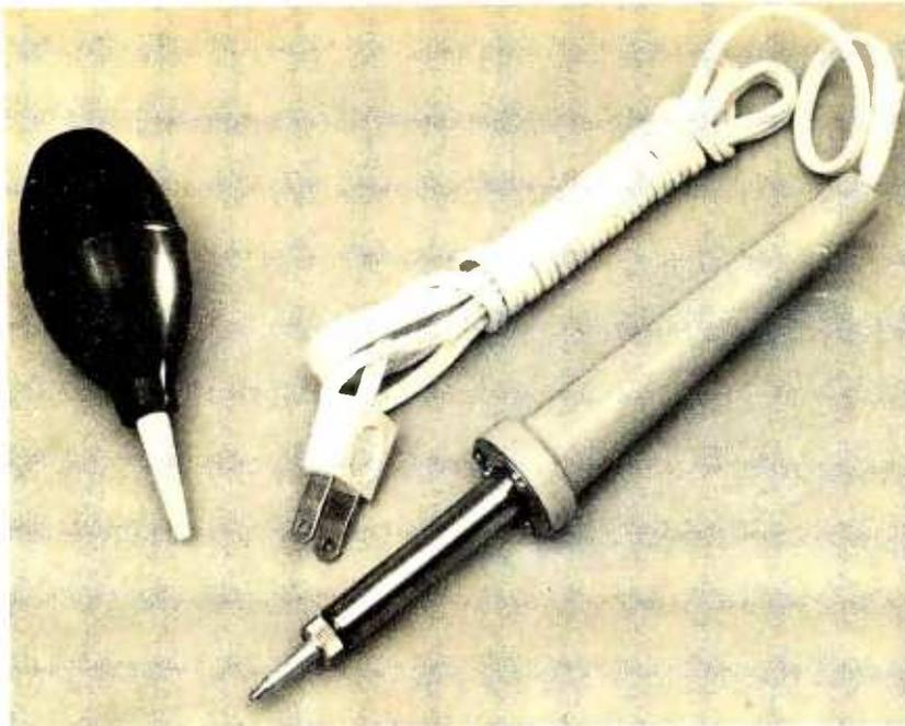
*Key 1: A low wattage soldering iron is a must for building computer kits (or any kit with delicate printed circuit runs). Here is a typical low wattage iron with a small tip, along with a suction bulb device which can be used to remove solder if necessary.*
