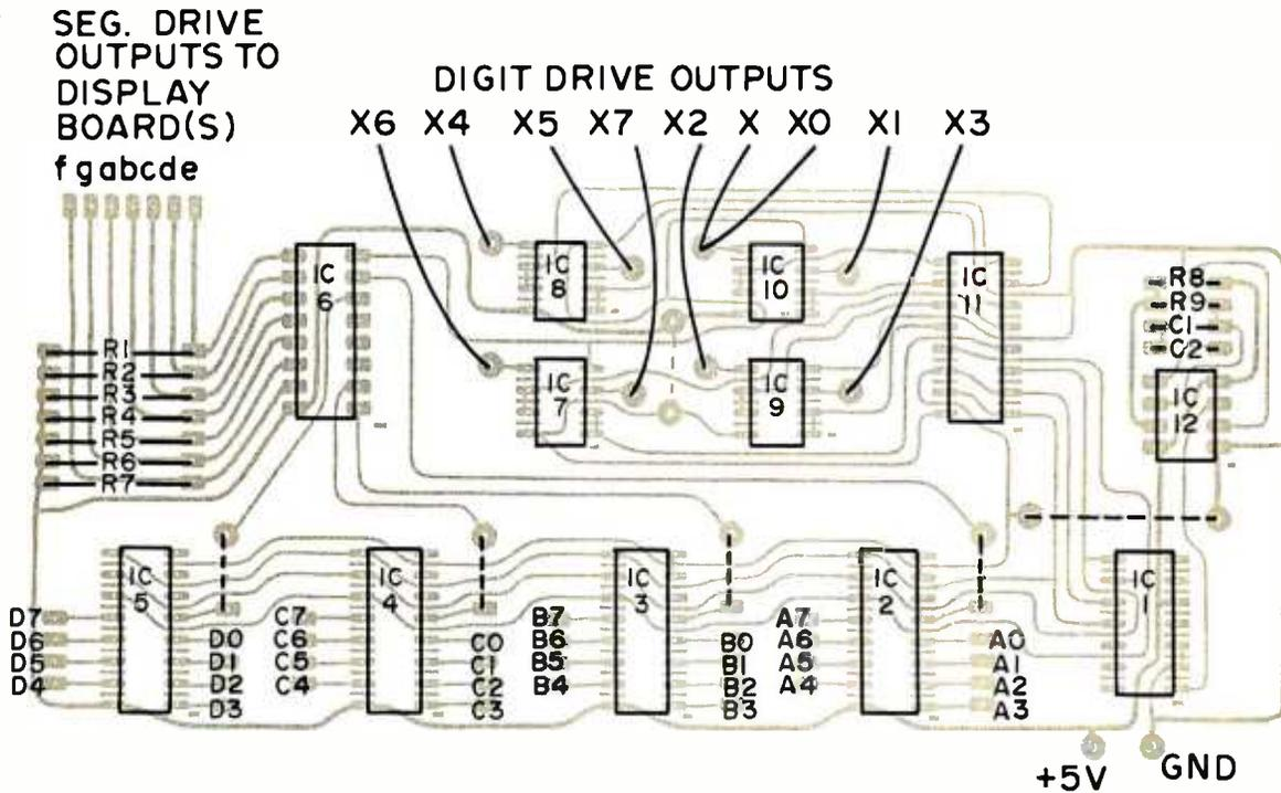
the counter will be disabled and the address on the counter inputs will appear at the outputs addressing the memory. IC2 provides a 60 ns delay, then a 60 ns pulse which writes the data at the memory data inputs into the memory location addressed. When the clock line returns to the high state, the counter will resume counting. The counter sequentially addresses the BCD data stored in the memory while it selects and enables the appropriate digit in the display.
