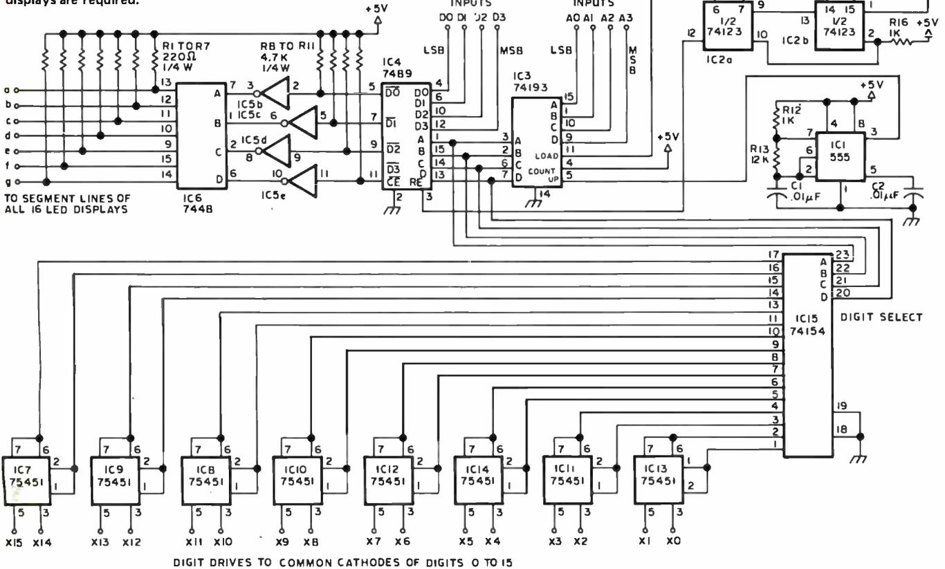
Figure 2: Circuit diagram of a digit-serial multiplexed 16 digit display with memory. The printed circuit layout of this version is depicted in figure 4. Figure 5 shows the printed circuit (two copies required) used to mount the displays.
