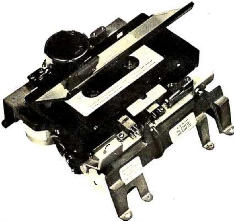
*Photo 2: The Phi-Deck Super Deck model manufactured by the Economy Company. This model allows varying tape speeds by varying the voltage to the capstan motor. The frame of the cassette transport is die cast, reducing alignment problems and making it quite rigid.*
