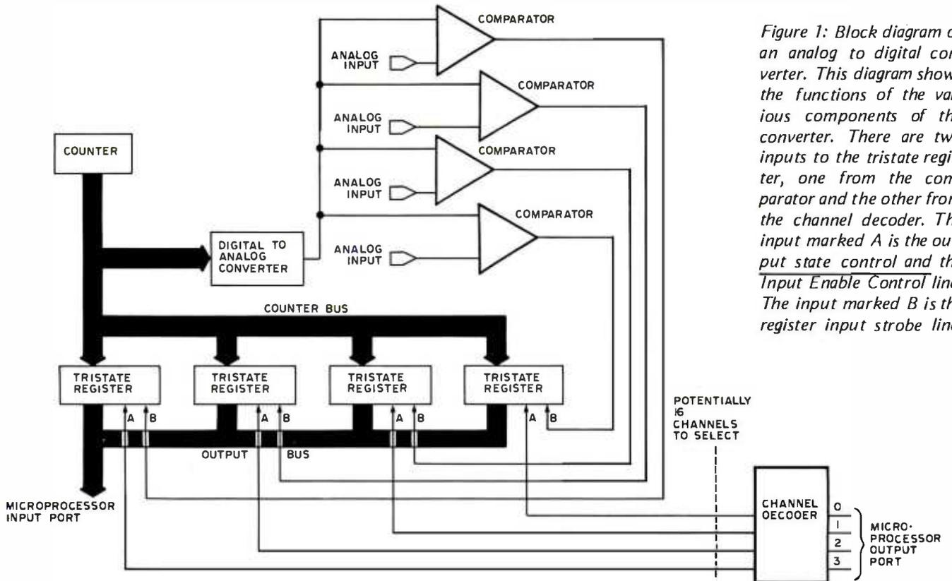
Figure 1: Block diagram of an analog to digital converter. This diagram shows the functions of the various components of the converter. There are two inputs to the tristate register, one from the comparator and the other from the channel decoder. The input marked A is the output state control and the Input Enable Control line. The input marked B is the register input strobe line.
