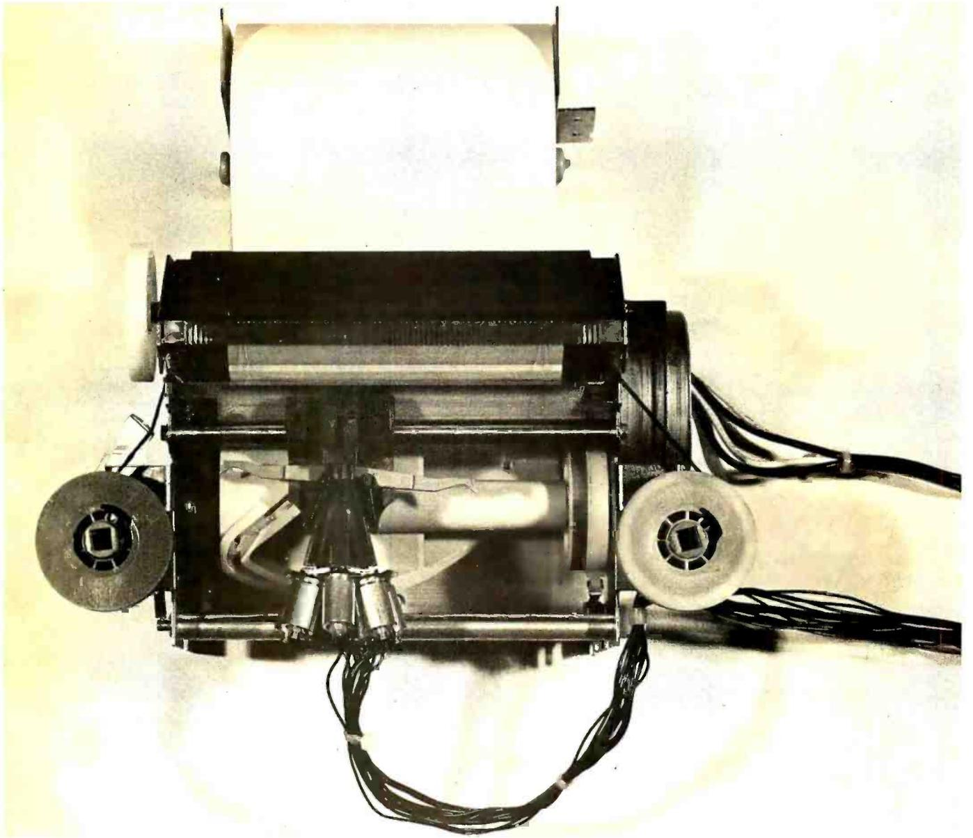
*Photo 2: This photograph displays the mechanical parts of the PR-40 printer. The seven solenoids can be seen to converge in a line at the print head. The positioning mechanism for the printing head is seen as the spiral groove under the head mechanism.*
