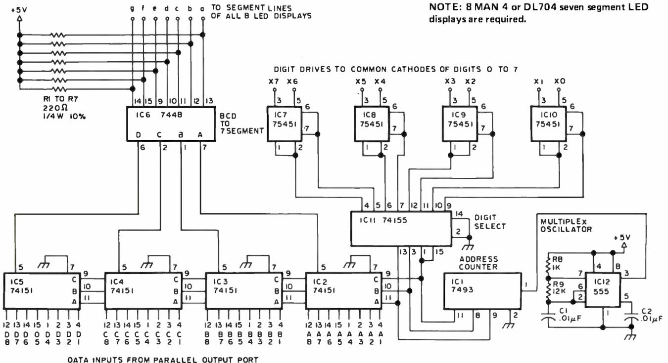
power configuration uses one 7 segment driver for each 7 segment LED in the display. Constant power is supplied to all digits. The multiplexed configuration uses only one 7 segment driver for several digits. Power is supplied to only one digit at a time, but is switched at a high rate so all digits appear to be on constantly. Since only one digit is powered at any given time, a certain amount of power is saved. This principle is widely used in electronic calculators.
