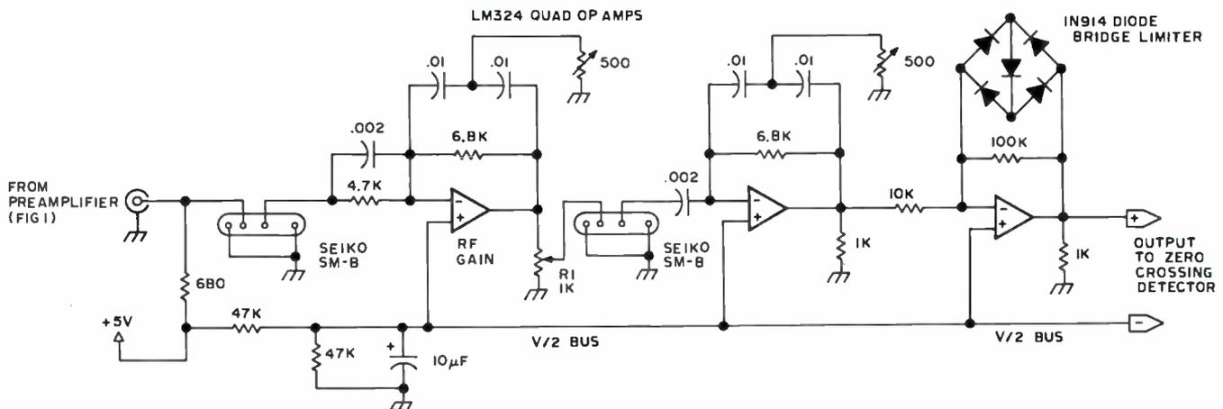
**Figure 2: Mini-O mechanical filter front end amplifiers.** This active circuit uses two mechanical filters manufactured by Seiko to provide a narrow bandwidth of 14 Hz at the  $-3$  dB points and a gain of 40 to 60 dB. The output passes through a diode bridge limiter implemented with an operational amplifier section, prior to reaching the zero crossing detector of figure 3. The physical construction of this circuit is shown in photo 3.
