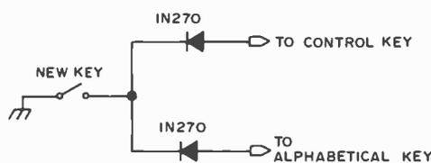
Figure 2: Simple circuit to add control keys to a keyboard. The new key is wired to both the control key and the alphabetical key. The diodes are needed to isolate the keys from each other.
