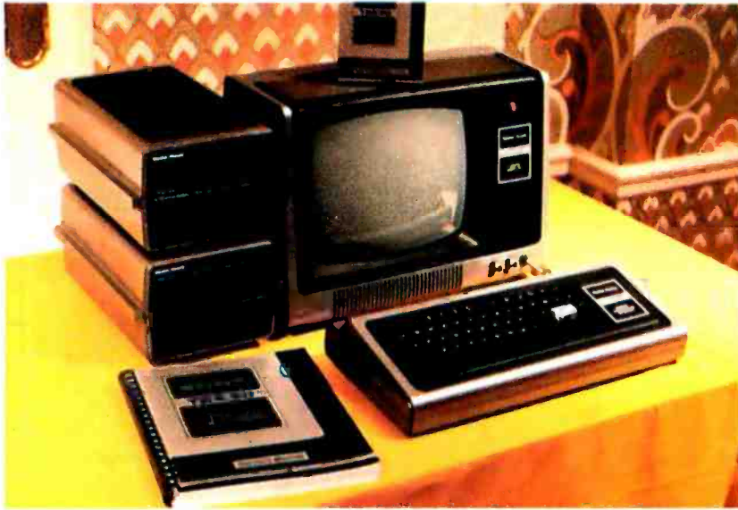
Photo 1: The New Radio Shack TRS-80 home computer system. Shown are the keyboard, video display monitor, instruction manual and prototypes of the upcoming memory expansion module and disk drive.
