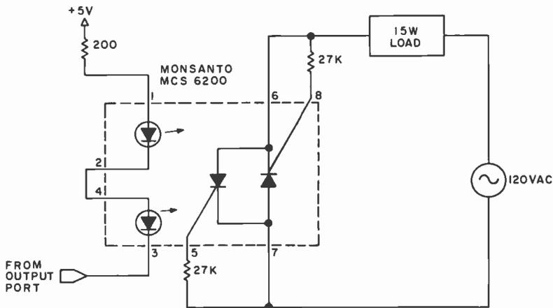
Figure 3: Using a dual SCR optoisolator for full wave control of an AC operated device.
