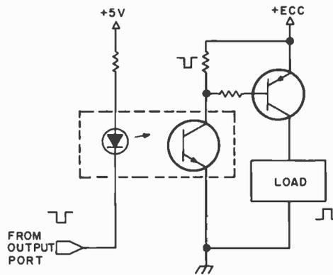
Figure 8: Using an external PNP transistor to increase the load current capability. This circuit is useful when the load must have one side common to the control system ground.
