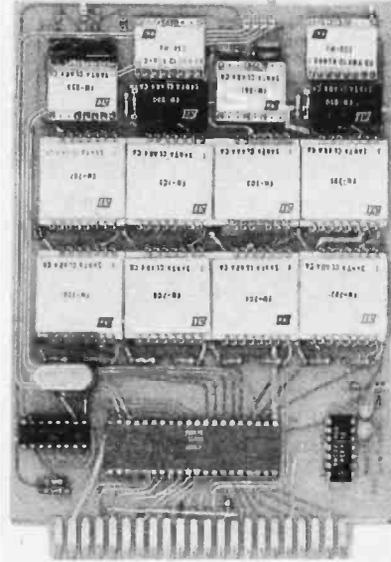
This touch tone transmit module contains a central office quality tone transmitter and receiver and is suitable for applications such as automatic dialing and receiving and automatic credit card verification. The module is built on an industry standard 4.5 by 6.5 inch 44 pin printed circuit board and is priced at \$1499 in single quantities, from Wintek Corp, 902 N 9th St, Lafayette IN 47904, (317) 742-6802. ■
