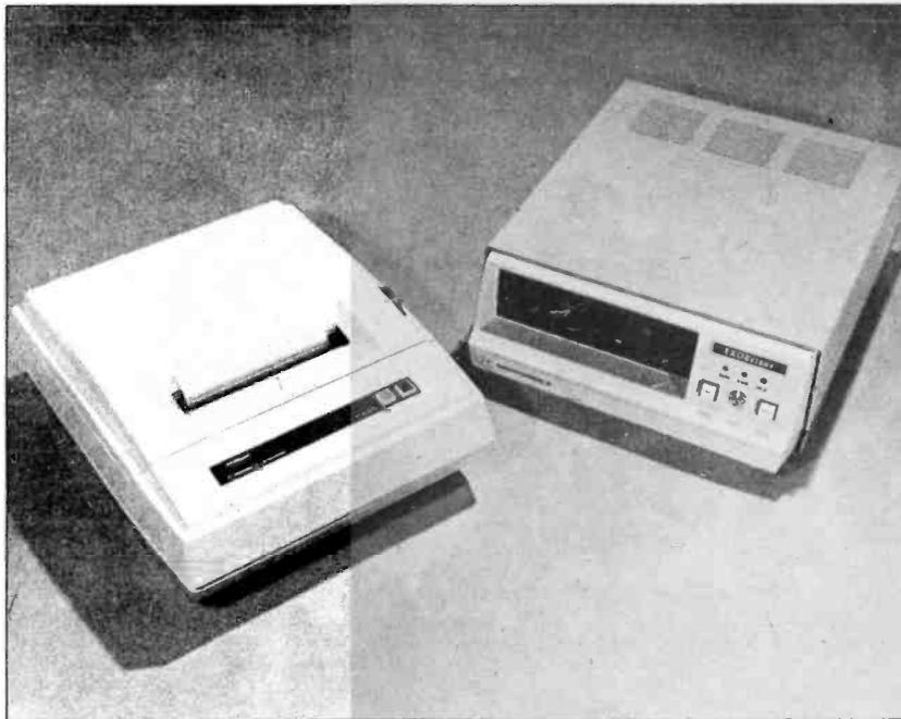
Designed for use with the Motorola Exorciser or Micromodules, this impact printer produces lines of up to 80 5 by 7 dot matrix characters at a speed of 110 characters per second (about 65 lines per minute). The print head moves in both directions on 8.5 inch (21.6 cm) wide roll paper and uses a conventional Teletype ribbon. A peripheral interface module and interconnecting cable are included with the printer, making the device functionally equivalent to a
