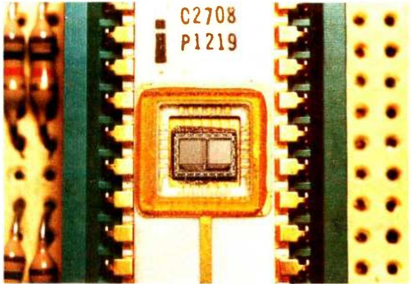
*Photo 1: A closeup of a 2708 erasable read only memory. Visible through the transparent quartz window are the two banks of FAMOS (Floating gate Avalanche injection Metal Oxide Semiconductor) storage devices. The contents of this memory storage circuit are erased by exposing the window to ultraviolet light.*
