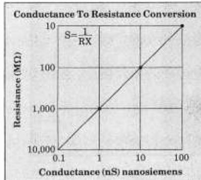
Beginner or pro, you'll find the meter you now have can't measure nanosiemens. So what? With the 8020A *conductance* function, you can measure the equivalent of 10,000 megohms in nanosiemens. Like capacitor, circuit board and insulation leakage. And, you can check transistor gain with a simple, homemade adapter. Only with the 8020A, a 13-oz. heavyweight that goes where you go, with confidence.
