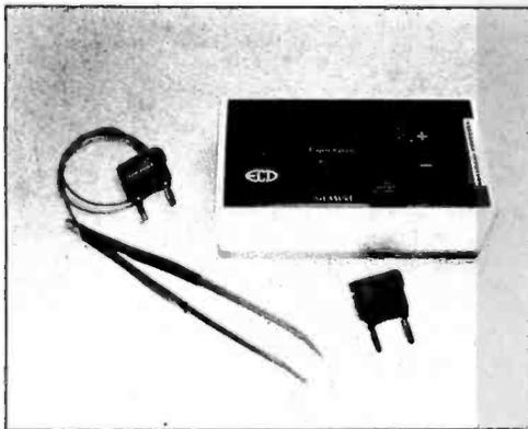
This chip probe for ECD Corp C-Meter expands the capability of the hand held 3-1/2 digit battery operated capacitance meter to function as a unique inexpensive portable measuring
