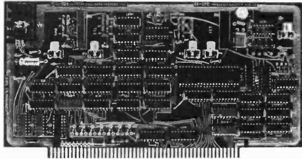
**88-UFC UNIVERSAL FREQUENCY COUNTER:** The 88-UFC is an S100 compatible frequency and period measurement module. The 88-UFC has four software selected inputs. Frequency measurement to above 600MHz and period measurement to 1/10th microsecond are standard. The counter provides nine digits of readout and is priced at \$179.00 in kit form.
