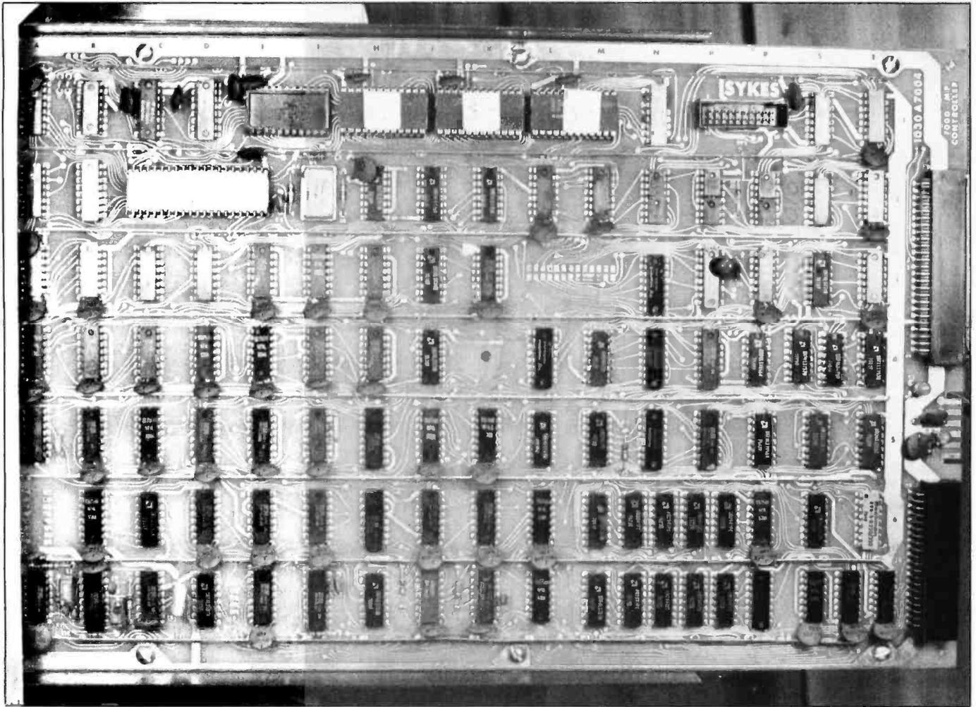
*Photo 3: The Sykes floppy disk controller board. This board mounts on the bottom of the Orbis drive; it contains a 6502 processor with read only memory programming needed to implement the high level command sequences available on the bidirectional interface.*
