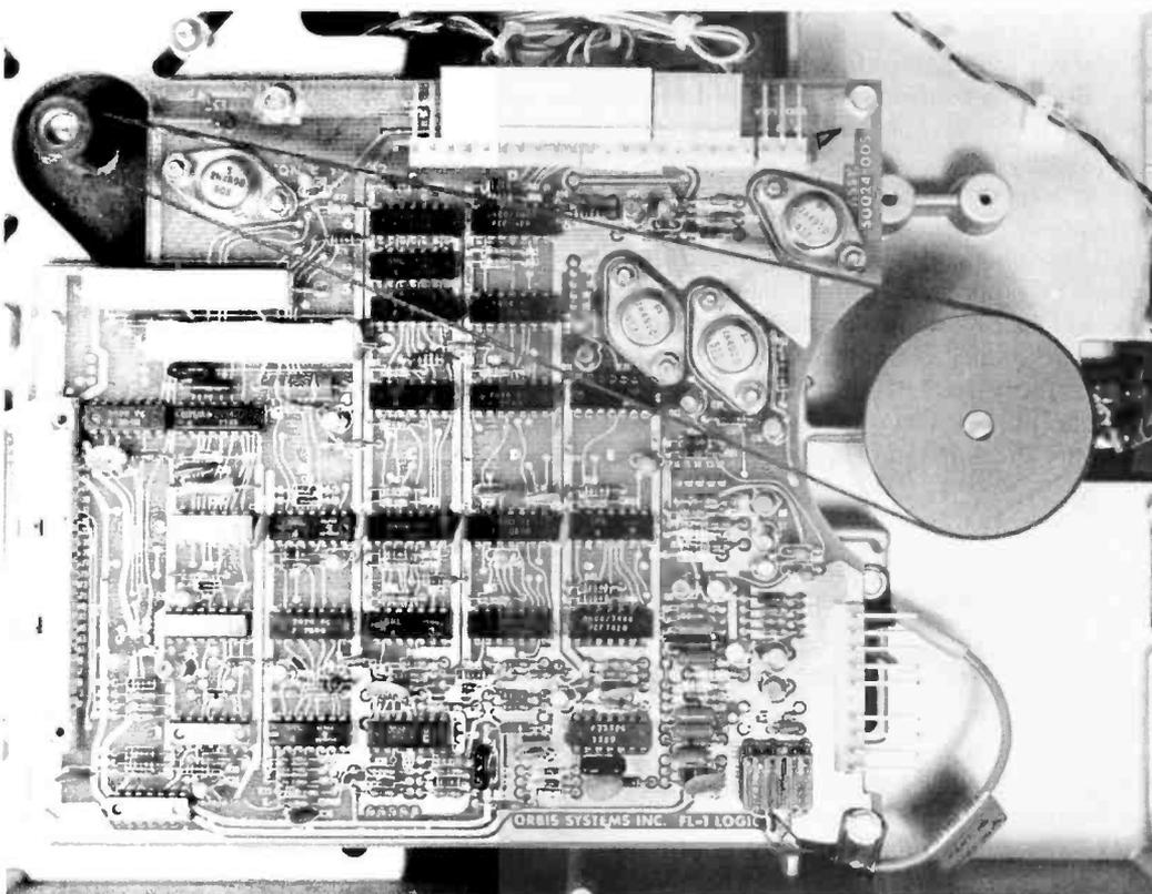
*Photo 2b: Bottom view of the Orbis disk drive used by Sykes, showing the built in control electronics and belt drive for the disk spindle. The Sykes interface (photo 3) has been removed for this picture.*
