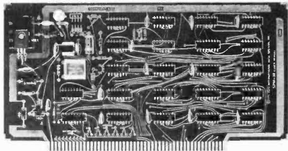
**88-SPM CLOCK MODULE:** The 88-SPM provides a time of day clock and an independent realtime clock on one S100 compatible module. Provisions are included for battery backup so the 88-SPM can maintain the time during power-off conditions. \$96.00 kit
