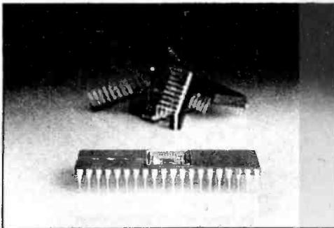
The INS8154 combined memory and input output chip is well suited to low end microprocessor applications. It includes 128 bytes of programmable memory and two 8 bit parallel IO ports. The chip is designed so that each bit in either port can be set, reset or read with a single microprocessor instruction. The 40 pin package is priced at only \$8.75 in 100 piece quantities, from National Semiconductor Corp, 2900 Semiconductor Dr, Santa Clara CA 95051, (408) 737-5000. ■
