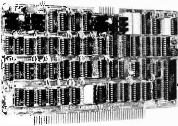
The Naked Terminal is a complete dumb terminal on an S-100 board. It contains a microprocessor with its own memory, its own software drivers, and its own internal bus. We built it that way so it won't take up any of the 64k memory address space of the S-100 bus. Keyboard and video monitor cables are available at additional cost.
