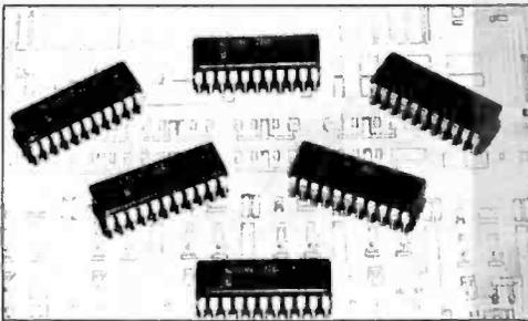
This microprocessor bus compatible chip incorporates a complete 8 bit digital to analog converter. The NE5018 includes a 5 V stable reference, a high slew rate buffer amplifier, a digital to analog converter and an 8 bit input latch. The device has a typical settling time of 2  $\mu$ s, requires supply voltages of 15 and -15 V and is priced at \$6.95 in quantities of 100 from distributors or direct from Signetics, 811 E Arques Av, Sunnyvale CA 94086, (408) 739-7700. ■
