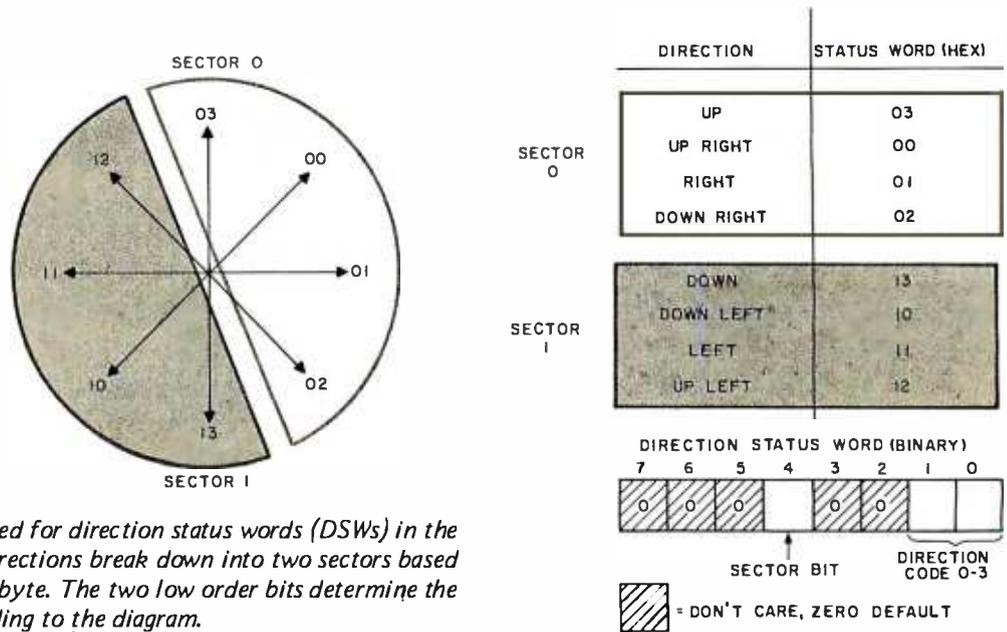
Figure 2: In the representation used for direction status words (DSWs) in the Microbot program, the possible directions break down into two sectors based on the status of bit 4 of the DSW byte. The two low order bits determine the direction within each sector according to the diagram.
