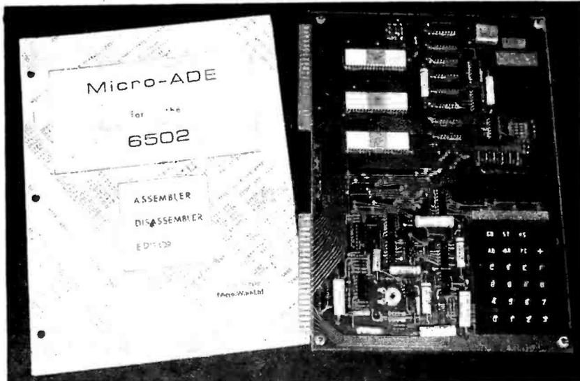
Micro-ADE is a complete assembler, disassembler and text editor package for 6502 based computers, customized especially for the KIM-1 with at least a 4 K memory expansion board. The two pass assembler can be used to assemble small programs directly in
