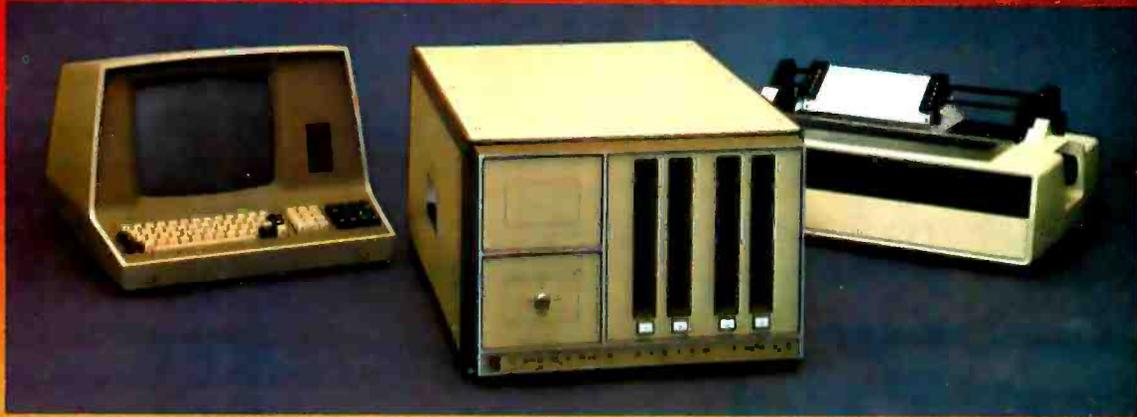
**A fast Z80 microcomputer with up to 512 kilobytes of RAM, 4 disk drives and 1 megabyte of disk storage—with CRT terminal and fast printer. Even an optional PROM programmer. Strong software support, too, like FORTRAN IV, Extended BASIC, and Macro Assembler.**
