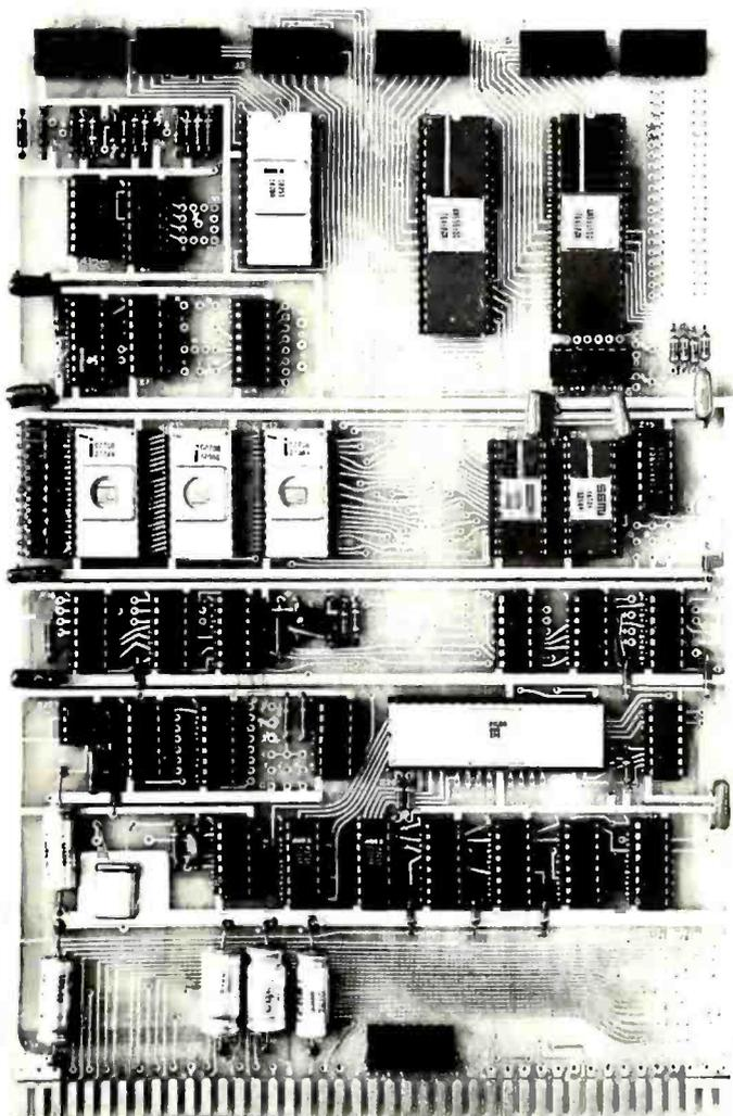
Shown above is a fully loaded RM Z-80 CPU System. Actual size: 7"x 10"
