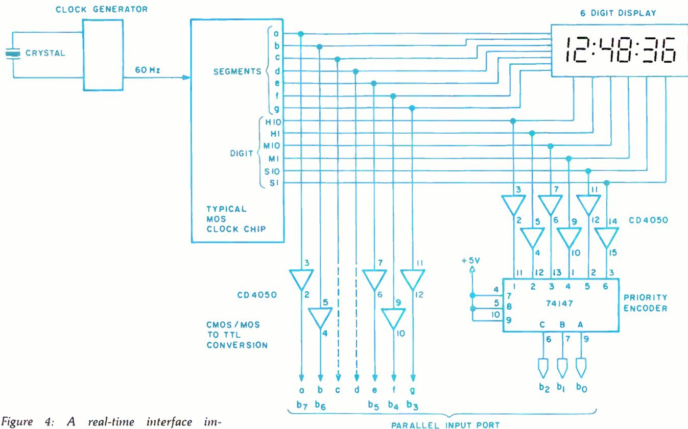
Figure 4: A real-time interface implemented using a typical clock chip.
