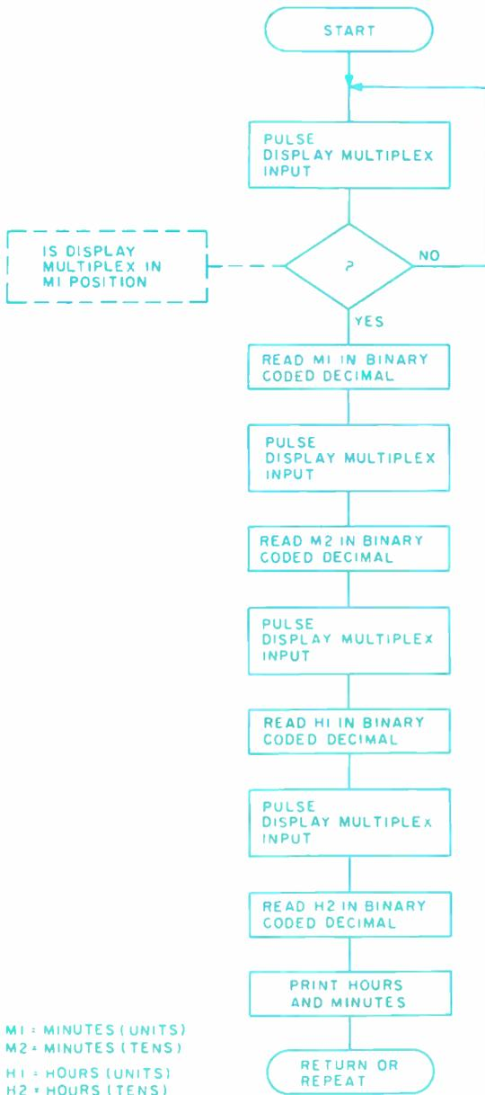
Figure 7: Flowchart of the program given in listing 1.
