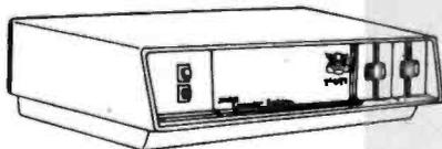
This sleek new mainframe is neatly trimmed to hold six S-100 boards, two mini-floppy drives, and is available in five colors. Power requirements: 115/220 VAC, 50/60 HZ. Weight: 27 lbs. (with drives). Dimensions: 21.375" Wide X 8.4" High X 15.875" Deep. Power Supply: 8 volts at 18 Amps unregulated. 16 volts at 3 amps unregulated. 16 volts at 3 amps unregulated. 5 volts at 3 amps regulated. 12 volts at 3 amps regulated.
