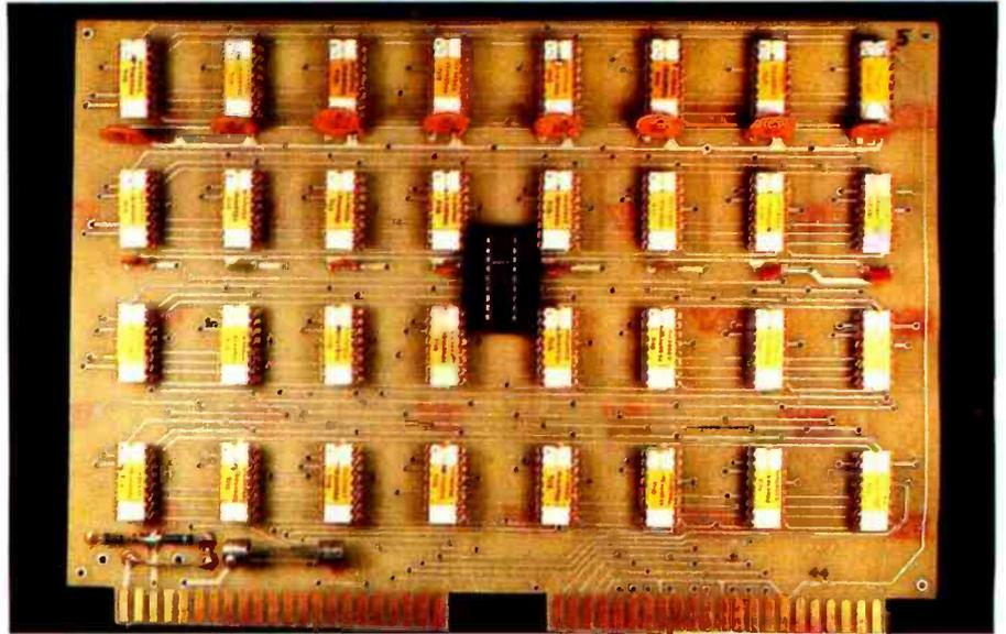
**Photo 2:** An exhibit of advancing memory technology. The single black integrated circuit at the center can replace the entire board of components. The center component is the Intel 8185 1 K-byte static programmable memory. The board is a 1 K-byte memory board from a Scelbi 8B microcomputer system, which used the 8008 microprocessor (circa 1975).
