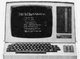
**Z-89 Computer System:** includes: Z19 Display, a built in 5 1/4" Floppy Disk, 2 serial ports, and 16K of memory. 2295.00
