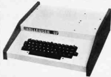
**The Challenger 4P.** A 4-slot computer with one open slot. Highly sophisticated 16 color video display. 32 rows x 64 columns, upper and lower case. 8K BASIC-in-ROM 8K RAM. 200-20KHz programmable tone generator. AC remote interface. Expandable to 32K RAM and two mini-floppy drives. **\$698.**
