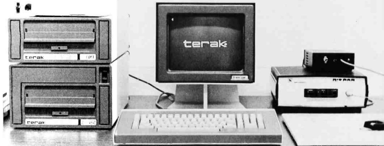
Photo 1: The Terak microcomputer with dual floppy-disk drive, video display, and keyboard. The Summagraphics Bit Pad consists of the digitizing tablet and the microcomputer control unit.
