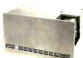
Packaged in the same physical size as the industry standard 5 1/4" minifloppy disk drive. The micro-Winchester stores thirty times as much data (6.38 megabytes unformatted), accesses data twice as fast (170 milliseconds) and transfers data twenty times faster (3.0 megabits per second.)
