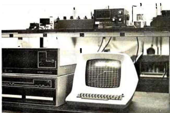
Photo 1: An Altair 8800b microcomputer, floppy-disk drive, and Lear-Siegler ADM 3A terminal interfaced to a pH meter.
