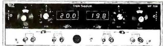
Two 0-20 VDC supplies, 0-2A full load. May be used in series to provide 0-40 VDC, 0-2A. One 5 VDC (0.4A full load) fixed supply. Two digital voltmeters 0-99.9 VDC with separate inputs on the front panel.
