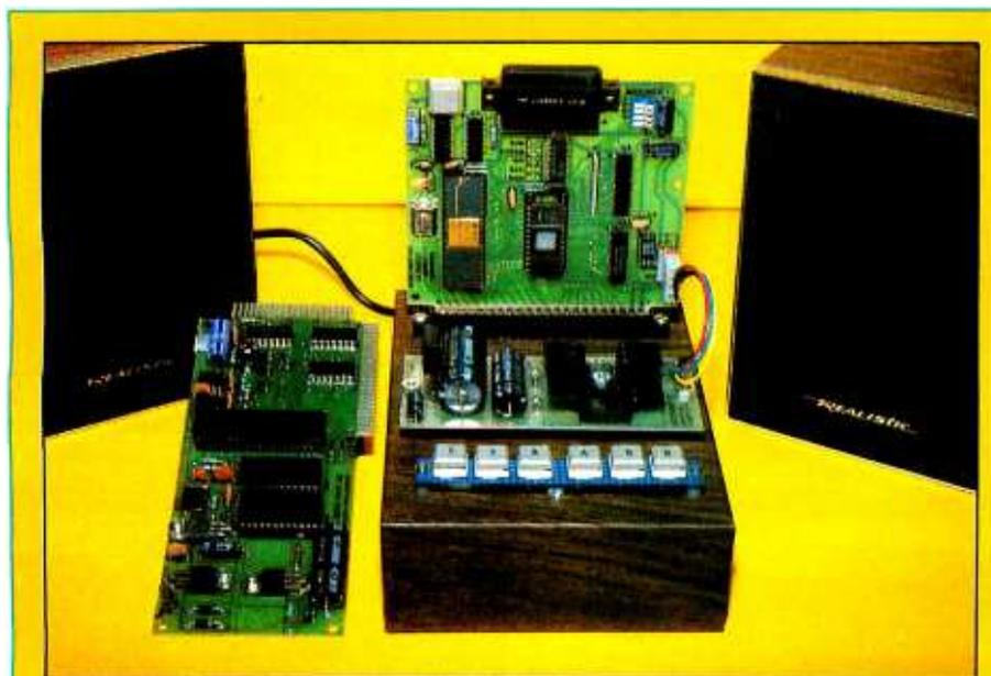
**Photo 2:** The Z8/Micromouth demonstrator. A Z8-BASIC Microcomputer is configured to run a ROM-resident program that exercises the Micromouth speech synthesizer presented in the June Circuit Cellar article. A Micromouth board similar to that shown on the left is mounted inside the enclosure. Six pushbutton switches, connected to a parallel input port on the Z8 board, select various speech-demonstration sequences. The Micromouth board is driven from a second parallel port on the Z8 board.
