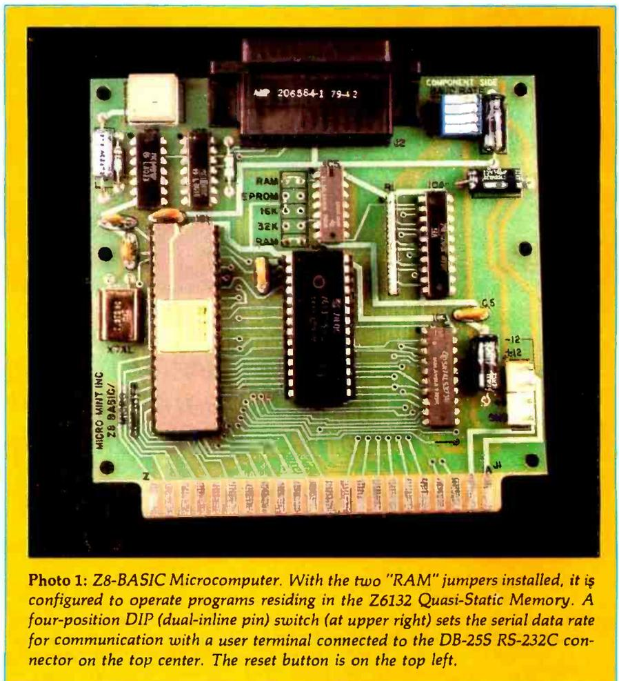
Photo 1: Z8-BASIC Microcomputer. With the two "RAM" jumpers installed, it is configured to operate programs residing in the Z6132 Quasi-Static Memory. A four-position DIP (dual-inline pin) switch (at upper right) sets the serial data rate for communication with a user terminal connected to the DB-25S RS-232C connector on the top center. The reset button is on the top left.
