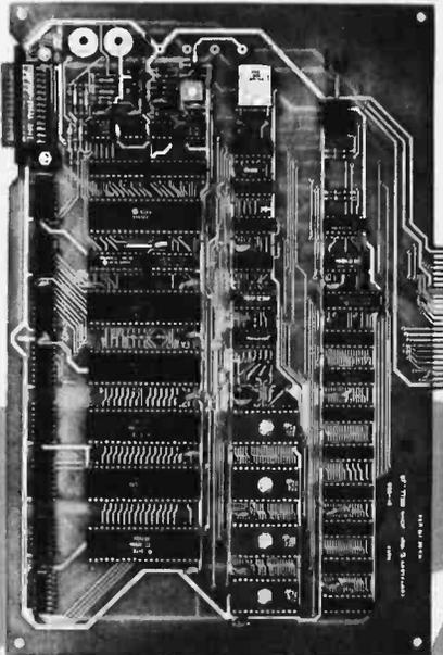
JBE's 7 3/4" x 11 3/4" 6502 base Microcomputer has the capacity for 16K of EPROM, 4K of RAM, 8 Parallel Ports and 1 Serial Port. Monitor and Tiny Basic are also available. The fully populated version includes:
