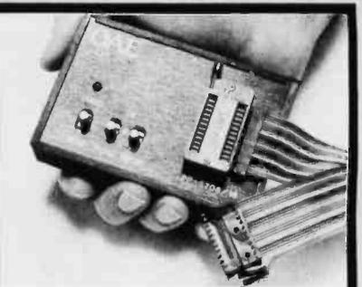
OAE's PP-Series EPROM Programmers plug directly into any vacant EPROM socket and allow you to transfer data directly from RAM to EPROMs. No additional power supplies are required. All timing & control sequences are handled by the programmer. Each unit includes internal DC to DC switching regulator, ZIF socket and 4 ft. ribbon cable terminated with a 24 pin plug. Programmers are available for all EPROMs from 2708's thru 2532's.
