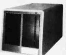
Packaged in the same physical size as the industry standard 5 1/4" minifloppy disk drive. The micro-Winchester stores thirty times as much data (6.38 megabytes unformatted), accesses data twice as fast (170 milliseconds) and transfers data twenty times faster (5.0 megabits per second.)
