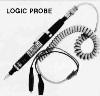
Compatible with all logic families using a 4 to 15V power supply. Thresholds automatically programmed. Visual indication of logic levels to show high, low, bad level or open circuit logic pulses.
