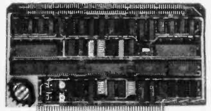
New, from JADE, one of the most advanced, technologically sophisticated Serial/Parallel Interrupt Controller systems in the world. On a single IEEE S-100 standard board, JADE has packed two bi-directional parallel ports with full handshaking, four serial channels (asynchronous, IBM-compatible bi-synch, synchronous, HDLC/SDLC) with complete modem control lines, and 16 counter-timer channels.
