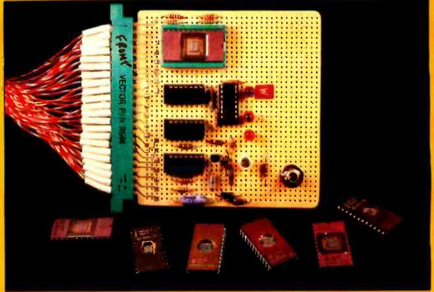
Photo 3: Type-2716 EPROM programmer, adapted from "Program Your Next EPROM in BASIC" (March 1978 BYTE, page 84). The circuit, which is driven through parallel ports, programs a 2716 in about 2½ minutes and is controlled by a BASIC program.
