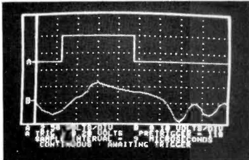
The APPLESCOPE system combines two high speed analog to digital converters and a digital control board with the high resolution graphics capabilities of the Apple II computer to create a digital storage oscilloscope. Signal trace parameters are entered through the keyboard to operational software provided in PROM on the DI control board.
