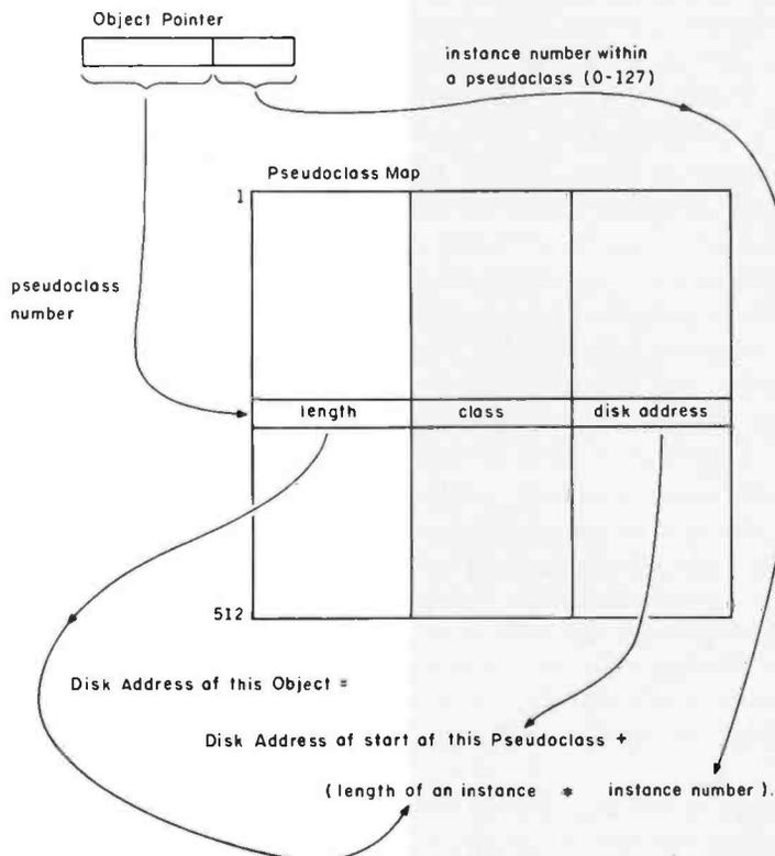
Figure 5: Information encoded in an object pointer.
