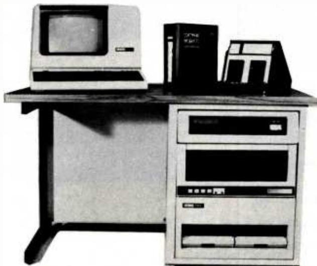
**CI-MWS03-SB** — LSI 11/2 computer workstation. LSI 11/2 CPU, 64KB Memory, power supply, KEV 11, in 16 slot rack mountable chassis. 2 port serial I/O. CRT terminal. 1 mega byte floppy disk system. Desktop workstation ..... **\$7,795.00**
