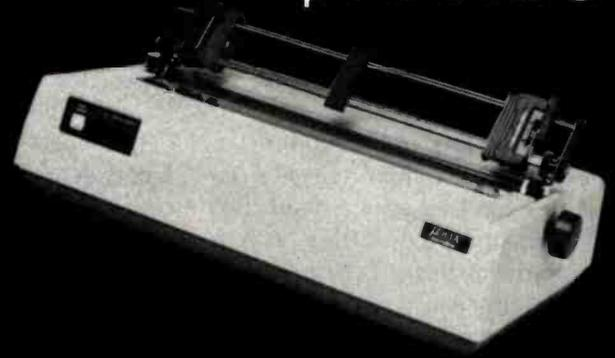
120 CPS, Bi-directional logic seeking 9x9 dot matrix, full 96 ASCII char. Set with true descenders centronics parallel port and RS232 serial port (up to 1200 Baud) standard, 136 col, includes Okigraph dot addressable graphics, friction feed and removable tractor. 31 lbs., 110 volt standard, 220 volt optional.
