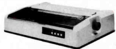
40 cps • Uses Diable Standard Printwheels • Built-in word processing functions • Universal power supply • Optional bidirectional tractors • Prints original plus 2 copies • Quick-change cartridge Ribbon
