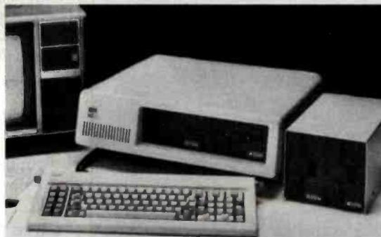
Minimum system requirements are an IBM System Unit with 16 Kbytes of RAM and 5 1/4" Diskette Drive Adapter. Drive models supported depend on DOS used. An optional cable available from Percom is required for external (add-on) drives.
