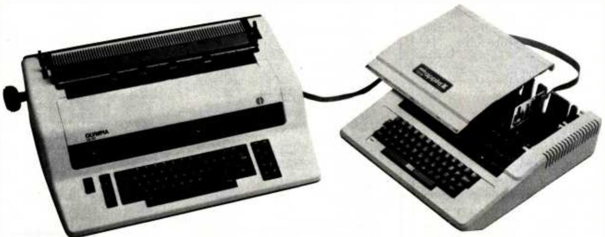
The Dataface D101 Apple II™ Interface Card gives you a letter quality printer while allowing the full use of your office electronic typewriter. The D101 requires only one card, the cable is included. Installation—simply plug in! No jumpers to set and no soldering necessary.
