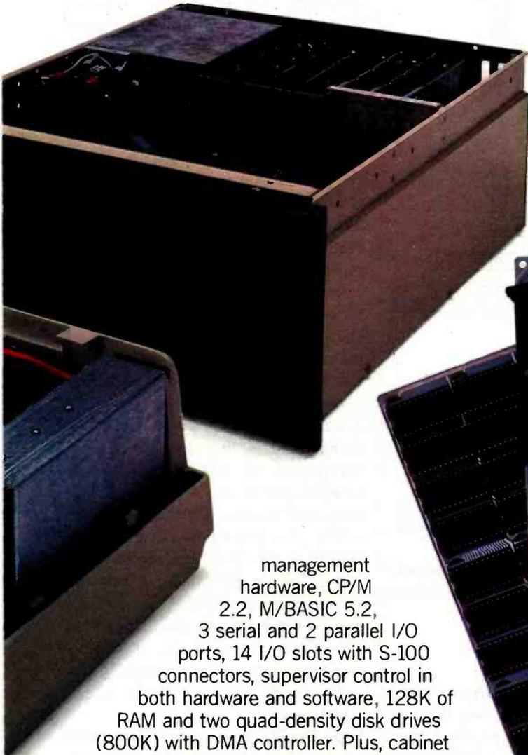
management hardware, CP/M 2.2, M/BASIC 5.2, 3 serial and 2 parallel I/O ports, 14 I/O slots with S-100 connectors, supervisor control in both hardware and software, 128K of RAM and two quad-density disk drives (800K) with DMA controller. Plus, cabinet (either desk-top or rack-mount), and power supply. The same system with 8" floppies and a full Megabyte of formatted storage costs \$5,659. And, we offer OEM pricing.
