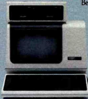
And by virtue of the fact that Digital's personal computing terminal is VT100-based, you get all the features that people buy VT100s for in the first place. Features like smooth scrolling with up to 132 columns display, split-screen viewing, double-height and width characters, and reverse video.
