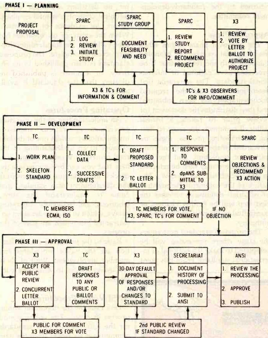
Figure 3: The standardization process is divided into three stages: planning, development, and approval. This flowchart depicts the milestones in each stage, beginning with the project proposal to SPARC (Standards Planning and Requirements Committee of ANSC X3), through the appropriate technical committees (TC) and ANSC X3 (American National Standards Committee for Information Processing Systems), culminating with submission to the secretariat and finally to ANSI.
