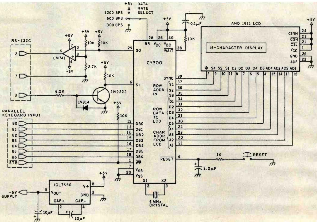
Figure 5: Schematic diagram of a single-line LCD computer terminal built around the CY300 and the AND 1811 display module. This style of RS-232C driver circuit was designed to use minimal  $\pm 5\text{-V}$  power, so it's not guaranteed to work through a long cable to the host computer.
