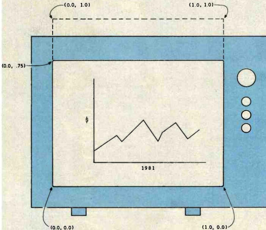
**Figure 8:** The unit screen is square, but most display screens are rectangular. The convention that has been adopted is to represent on the display screen only the lower 75 percent of the unit screen. That is, any point with a y coordinate greater than 0.75 will not be seen.
