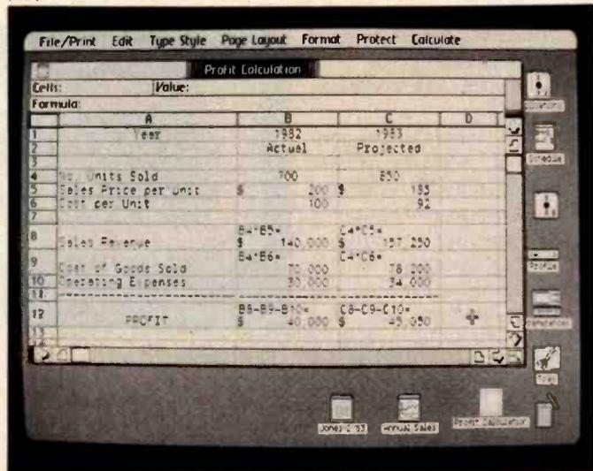
Photo 8a-b: The Lisa Calc program. Photo 8a shows a simple spreadsheet; 8b shows the same spreadsheet after the "Show Formulas and Values" command is executed.
