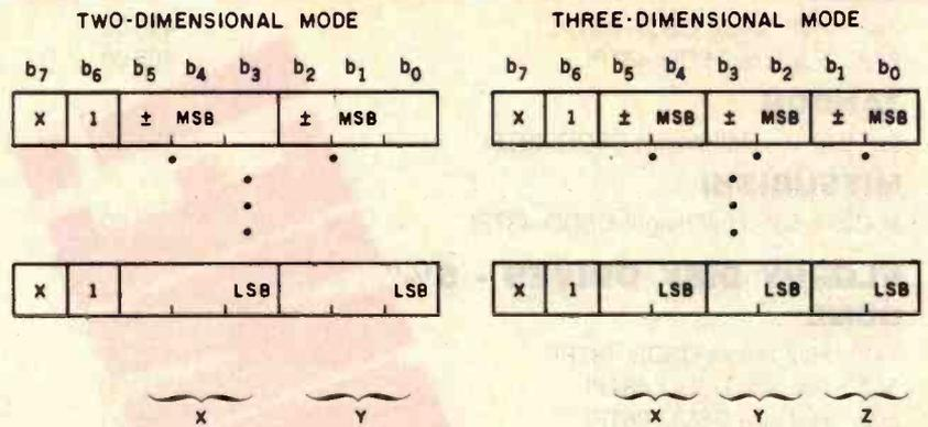
Figure 10: In NAPLPS, coordinates are specified with a varying number of bytes. In the two-dimensional mode, each byte contains 3 bits of the x coordinate and 3 of the y. In the three-dimensional mode, each byte contains 2 bits each for the x, y, and z coordinates. MSB indicates the most significant bit; LSB, the least significant bit.
