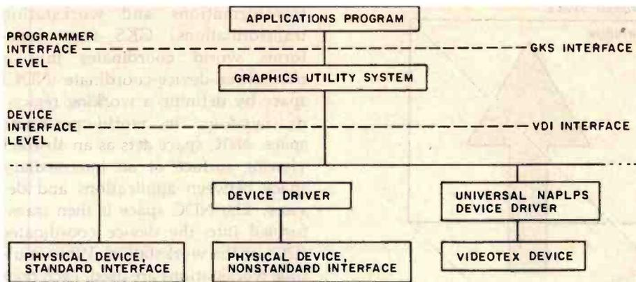
**Figure 1:** The two main levels of graphics standardization are the programmer and device-interface levels. The Graphical Kernel System (GKS) provides a standard interface between the application program and graphics utility programs. The Virtual Device Interface (VDI) standardizes the interface between graphics utilities and device drivers.
