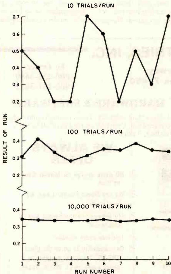
Figure 3: Results of 10 different Monte Carlo runs to find the shaded area of figure 2 showing the statistical fluctuation for three different numbers of trials per run. The exact result is 0.333.
