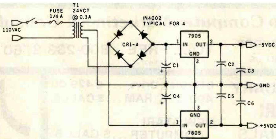
Figure 2: Design of a suggested power supply. The power must be extremely stable if the unit is to live up to its potential.
