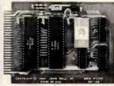
6502 MPU, 6522 VIA, 2716 EPROM, 2114 RAM single board computer. Single 5 volt power supply at 400 Ma. Two independent 8 bit I/O ports with handshake lines. RC controlled 1 MHz clock.
