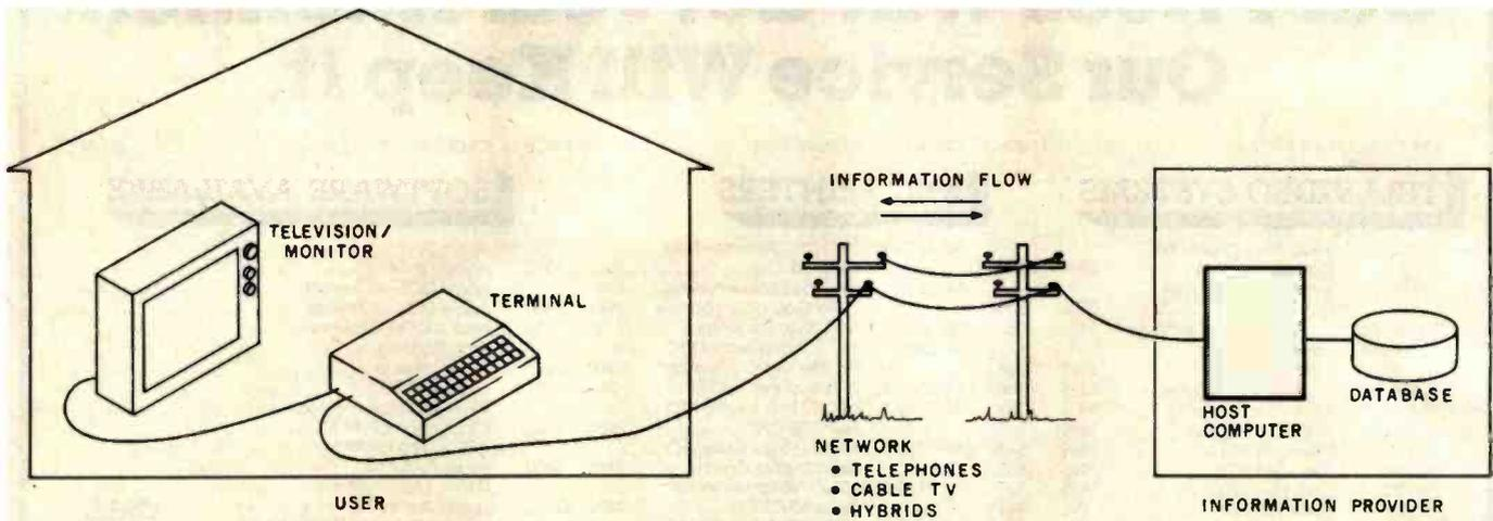
**Figure 2:** A diagram of a typical videotex system. Videotex is defined here as two-way communication of textual and graphical information between a low-cost, user-friendly terminal and a large, central host computer. Communication can be by telephone lines, television cables, or a hybrid system using a broadcast television channel for information sent from the host computer and using telephone lines for information sent from the terminal.
