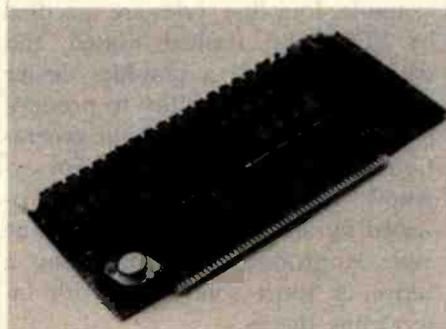
*Where it all started: pictured is the popular Multiuser I, Macrotech's first product. This widely used board provides 256 Kbytes of dynamic ram with 4K page memory mapping (called M<sup>3</sup>), 8/16 bit operation, 24 bit addressing and byte parity checking.*
