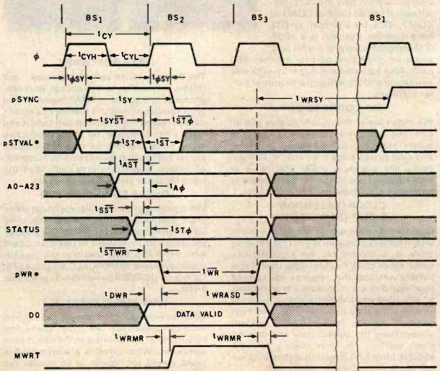
Figure 4: Timing diagrams for basic bus cycles. Figure 4a shows a read cycle; figure 4b shows a write cycle; and figure 4c shows the timing required for the RDY, XRDY, and SIXTN\* signals (when pSYNC is false, RDY and XRDY are tested only when the master is in a wait state).
