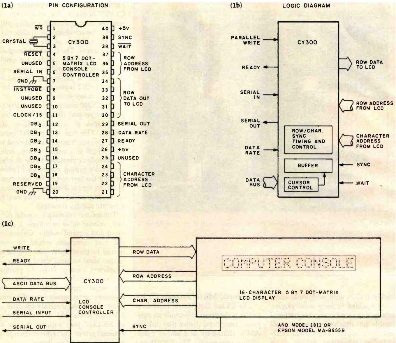
Figure 1: Descriptive information on the Cybernetic Micro Systems CY300 LCD Console Controller. Figure 1a shows the pinout specification of the CY300, 1b is a functional logic diagram of the CY300, and 1c shows a block diagram of a display system using the CY300.
