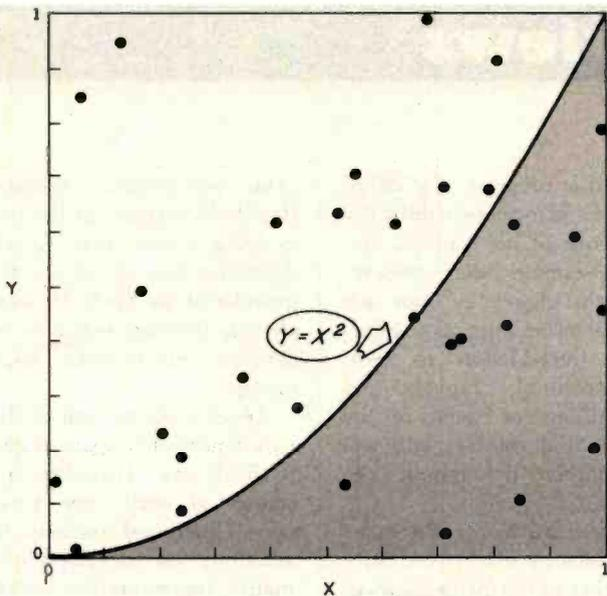
Figure 2: Plot of 30 random  $x, y$  points giving a Monte Carlo approximation of the area under the curve  $y = x^2$  in the unit square. The area ( $A$ ) can be estimated as points under the curve divided by total points. In this instance  $A = \frac{11}{30} = 0.37$ . The true result is 0.333.
