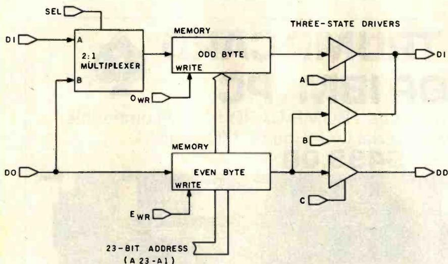
**Figure 2:** Block diagram of the circuitry needed by S-100 bus slaves for byte and word transfers under the IEEE-696 standard.
