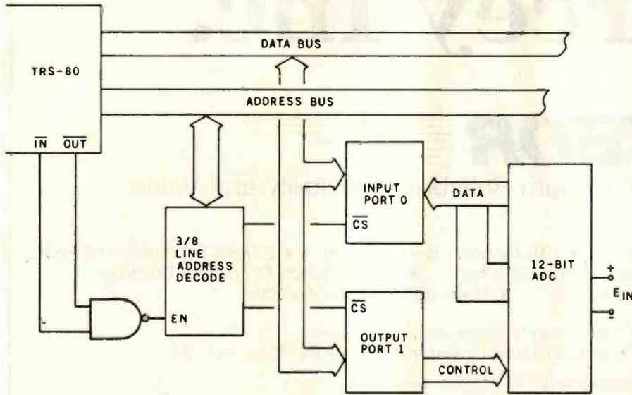
Figure 1: Diagrams of the complete interface circuit. In figure 1a, a block diagram of the circuit shows how the I/O port address is decoded and how the eight data lines are partitioned into an input bus and into an output bus. Figure 1b is a schematic diagram developed from figure 1a. Note that all eight data lines are used when transferring data to the computer and only three lines are used by the computer to control the ADC.
