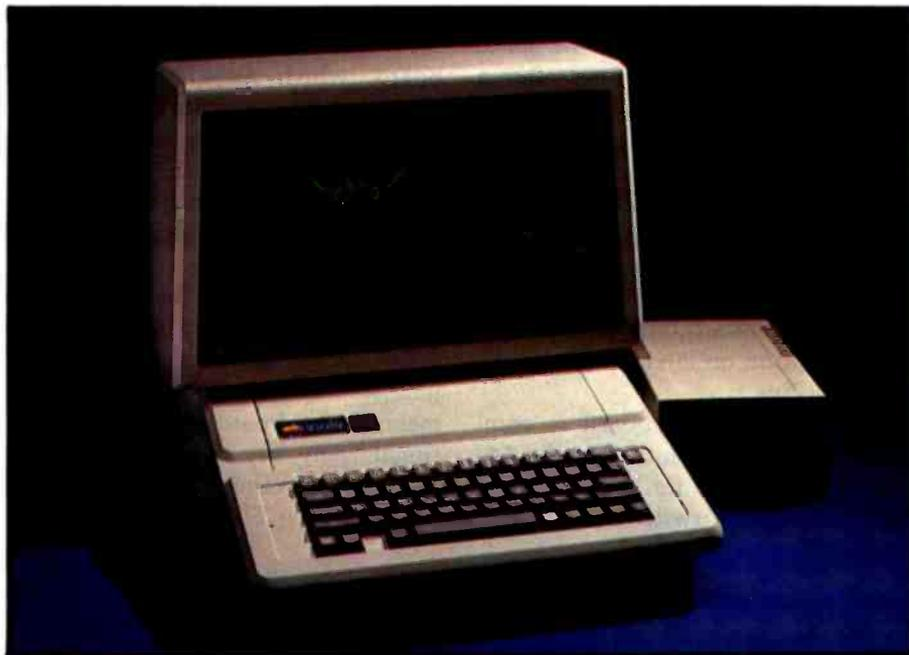
**Photo 1:** An Apple IIe system made up of the Apple Monitor III, the Apple IIe computer, and a Disk II 5 1/4-inch floppy-disk drive.
