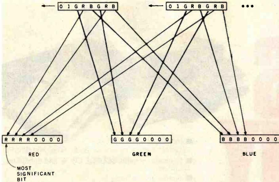
**Figure 13:** Color information is encoded in a manner similar to that used for coordinates. Each data byte contains 2 bits of information for each of the primary color components: red, green, and blue. A varying number of bytes can be combined to specify colors with almost unlimited precision. Here, 2 data bytes have been combined to yield 4 bits of information on each red, green, and blue component of a color.
