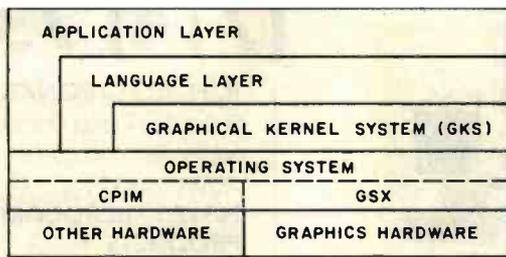
**Figure 3:** This layer model shows the relationship of GKS and VDI to other components in a graphics system. Each module may call the functions of the adjoining layer below. An example of this is the Graphics System Extension (GSX) to the popular CP/M family of operating systems.
