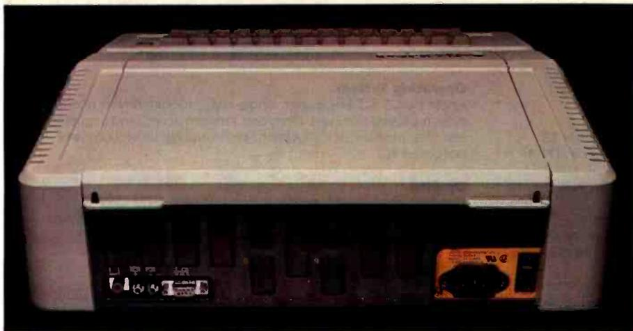
**Photo 2:** The rear panel of the Apple IIe. Instead of the plastic slots found in the Apple II, the Apple IIe's metal back panel is designed to mount 9-pin, 19-pin, and 25-pin D-type connectors in precut recesses, providing more reliable connections and reduced RF interference. The built-in game-paddle connector has also been changed to a 9-pin D-type; however, the older-style connector is still available inside the case to accommodate existing devices.
