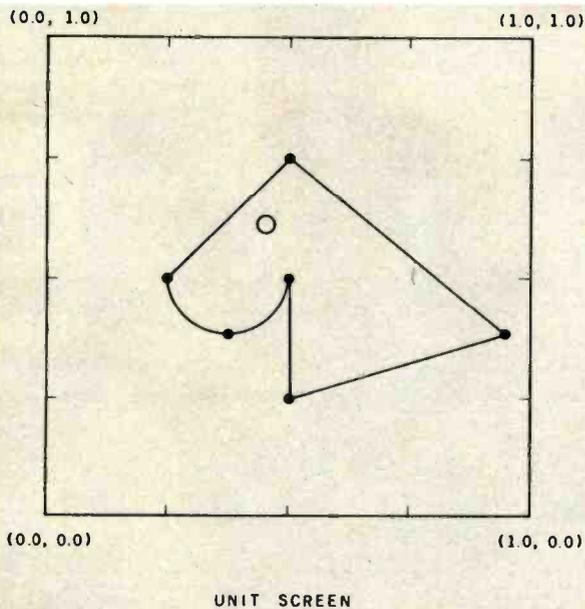
**Figure 7:** The unit screen of NAPLPS. All coordinates are represented as fractions between 0.0 and 1.0. The figure on the screen was drawn with the commands listed on the left. The advantage of this coordinate scheme is that it can be easily implemented on display screens of various resolutions and sizes.
