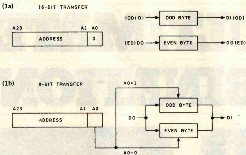
**Figure 1:** Data transfers as performed according to the IEEE-696 standard. In figure 1a, a 16-bit transfer is shown using all of the available data lines. Data whose least-significant address bit is 0 is considered even, while data whose least-significant address bit is 1 is considered odd. Figure 1b shows how the odd and even bytes are employed during an 8-bit-wide transfer of 16-bit data (called a byte-serial transfer).
