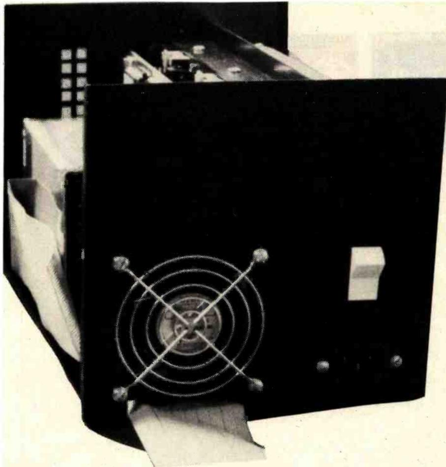
Photo 5: Ventilation details of the disk-drive assembly.
