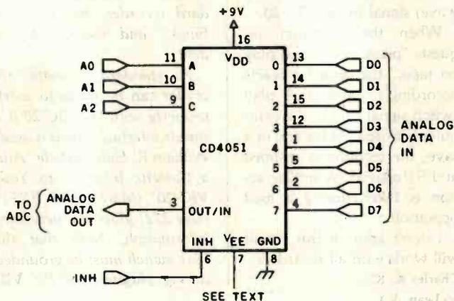
Figure 2: The 4051-type bilateral switch and its pin assignments.
