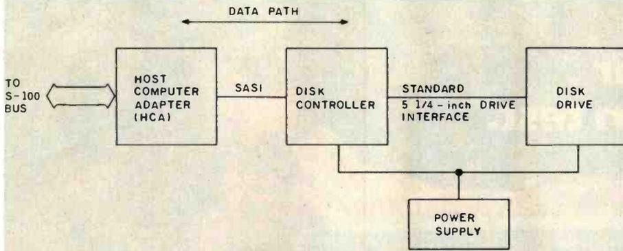
Figure 1: Winchester disk-drive subsystem block diagram.
