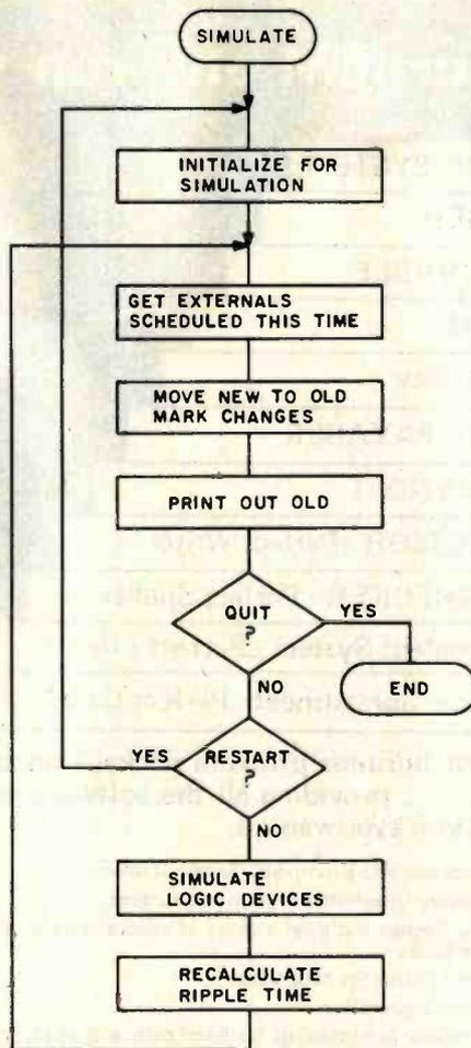
capability should be included to allow predefined blocks of circuitry—macrocircuits—to be installed simply. A macrocircuit is a black box with specified input and output signals; the description of the macrocircuit includes the logic devices required to generate the output from the inputs, using internal
