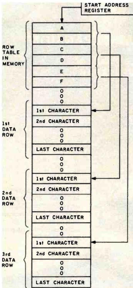
Figure 2: Contiguous row-table format. Each data row (screen line) is stored contiguously within memory. The start address register points to the first row table.
