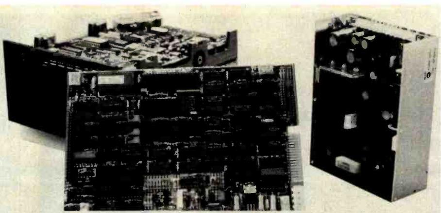
Photo 3: The Winchester disk-drive subsystem components before assembly.
