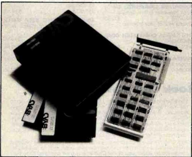
**Photo 2:** The DS1 from Byad uses a technically more elegant approach to integrating the Z80B system into the IBM PC. When the Z80B is in control, the 8088 uses its system memory for disk and print buffering.
