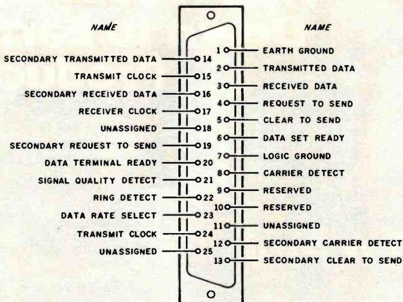
**Figure 1:** Pinout specifications of the RS-232C interface. The popular DB-25 connector is most often used for RS-232C connections, but it is not required by the EIA standard.
