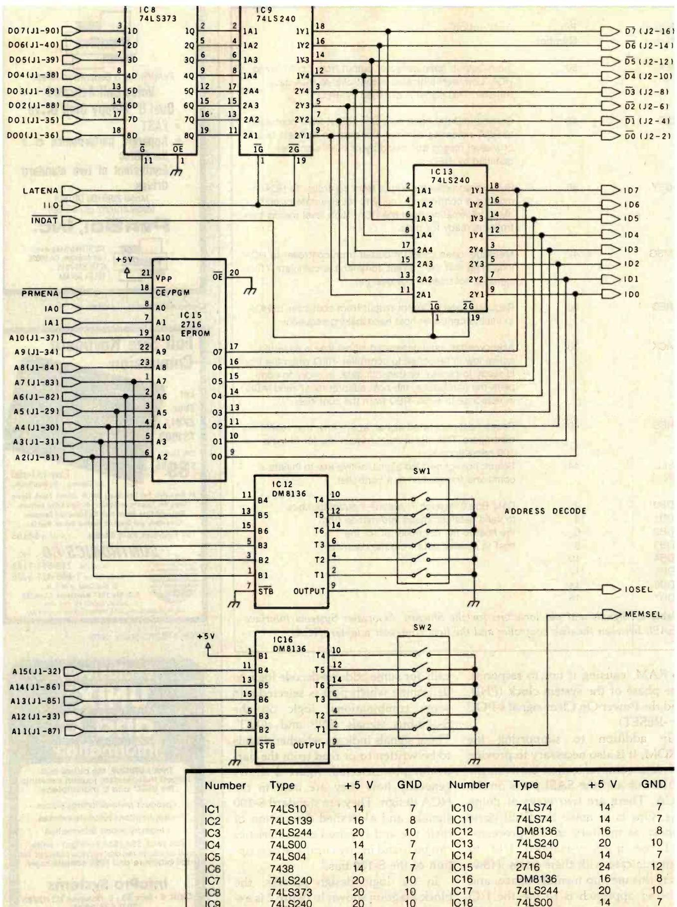
Figure 3: Diagram of the address-decode logic of the HCA.
