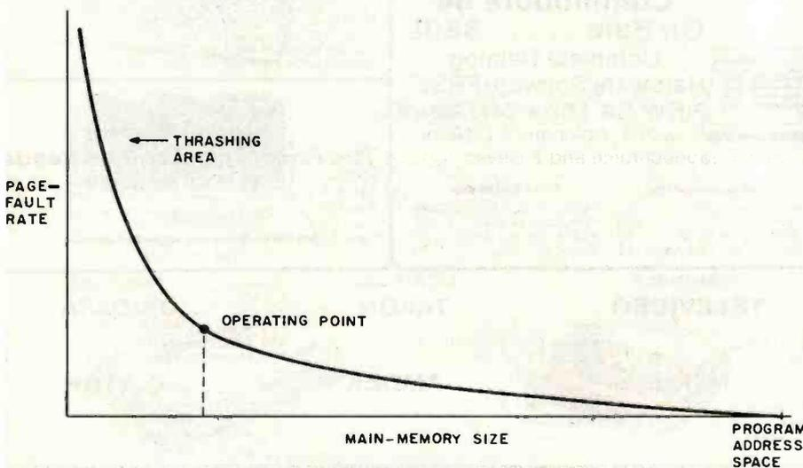
**Figure 4:** A graph showing how the page-fault rate (i.e., the rate of accesses to pages not present in main memory) is related to the size of main memory. The operating point is the memory size sufficient to hold a program's most frequently accessed routines—its working set. Adding memory past this point has little effect on the page-fault rate. Of course, as the needs of a program change, the operating point will shift.
