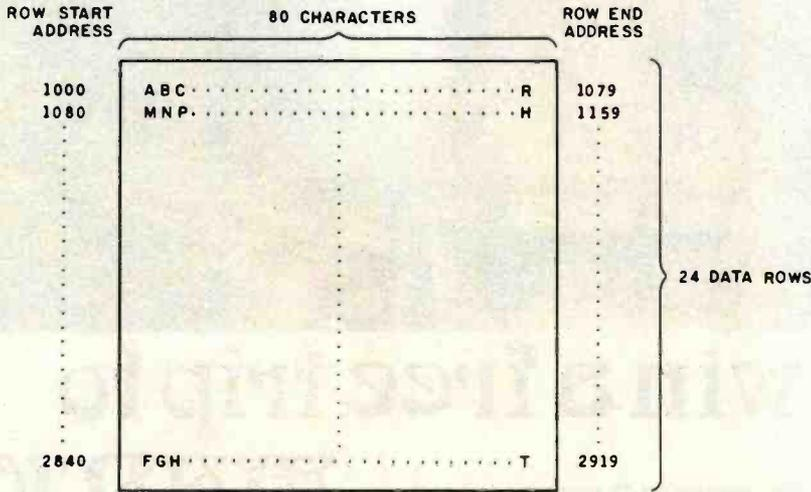
**Figure 1:** A typical (80 by 24) display employs sequential memory addressing for its 1920 bytes of video memory.
