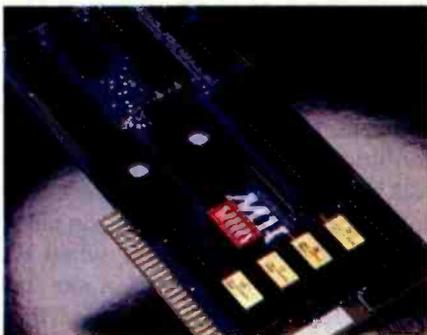
FOR APPLE II COMPUTERS, Microbuffer II features on-board firmware for text formatting and advanced graphics dump routines. Both serial and parallel versions
