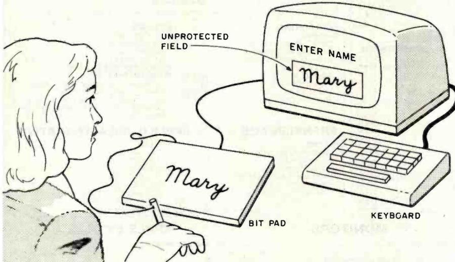
**Figure 7:** Input from a bit pad can be translated into a series of Incremental-Line instructions and placed into an unprotected (user) field.
