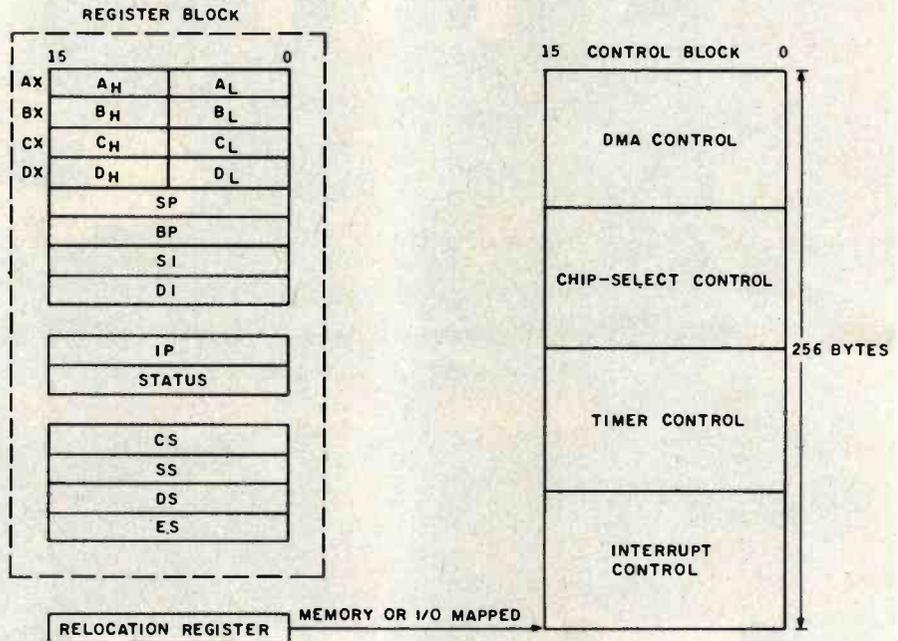
**Figure 2: The 80186 register file.** Each of the four segment registers—CS, SS, DS and ES—defines a 64K-byte area of memory. There are four general-purpose registers: AX, BX, CX, and DX. The pointer and index registers are stack pointer (SP), base pointer (BP), source index (SI), and destination index (DI). IP is the instruction pointer.
