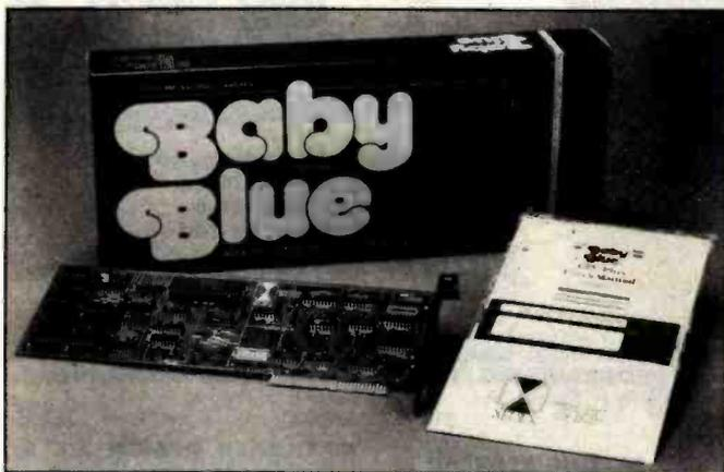
**Photo 1:** The Baby Blue CPU Plus from Xedex converts your CP/M-80 files into PC-DOS format and attaches a header to the file to identify it. You don't have to keep track of two different file formats.
