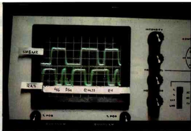
**Photo 4b:** This is a "scope loop," like those in listing 2. The first sMEMR (high-going pulse) fetches an indirect-read instruction (B-(HL)). The next sMEMR carries out the instruction. Because HL points to the instructions location, we have two kinds of read from the same location. The single  $\overline{RAS}$  in the middle is the data read. Finally, an E9 hexadecimal (jump to (HL)) is fetched, restarting the loop.
