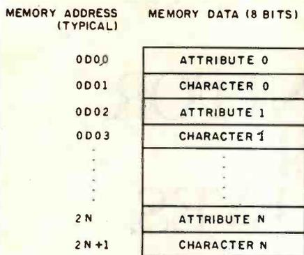
**Figure 4:** The Attribute Assemble mode lets the programmer create a pseudo 16-bit word that describes both the character and its attributes (see text).
