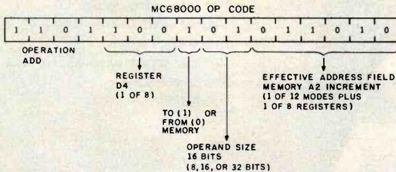
**Figure 2:** The MC68000 ADD instruction op code shows the power available with 16-bit operations. Multiple registers with variable operand sizes and a large address field give a programmer tremendous flexibility in programming.
