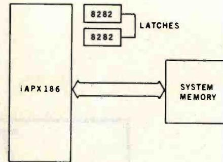
Figure 1: (1a) Chips necessary to make an 8086-based microcomputer system. (1b) Chips necessary to make an 80186-based microcomputer system.
