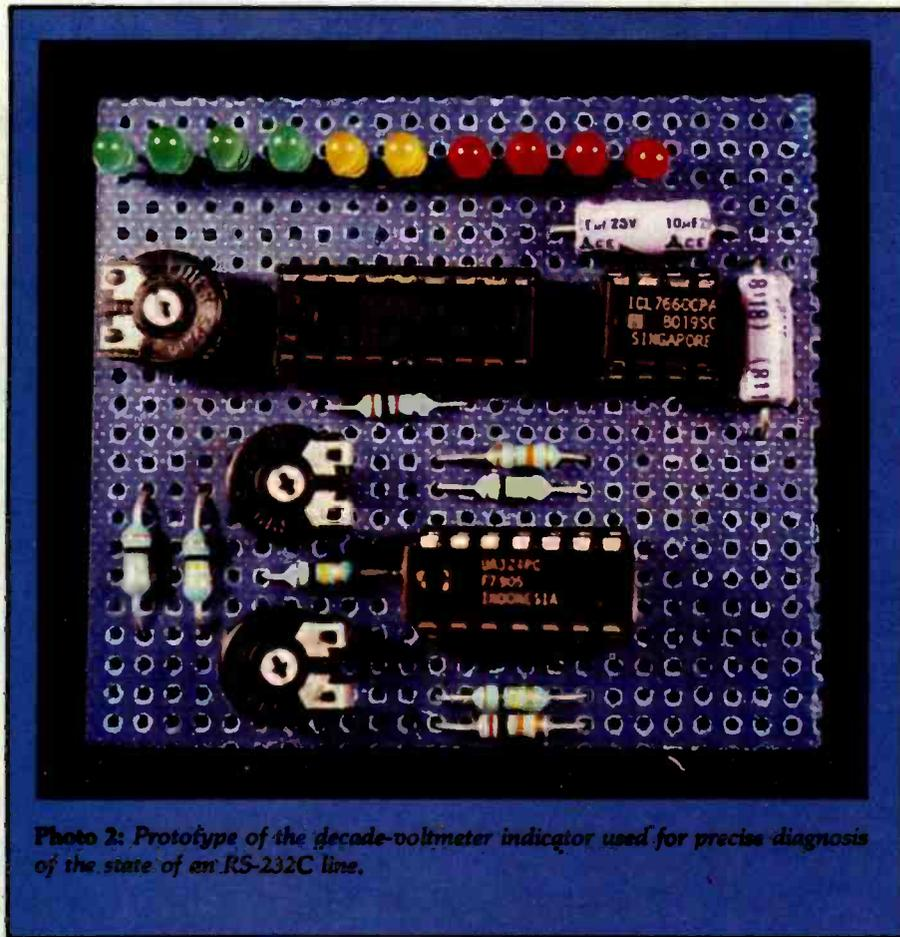
Photo 2: Prototype of the decade-voltmeter indicator used for precise diagnosis of the state of an RS-232C line.
