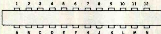
Figure 1: VIC-20 user port I/O connections.
