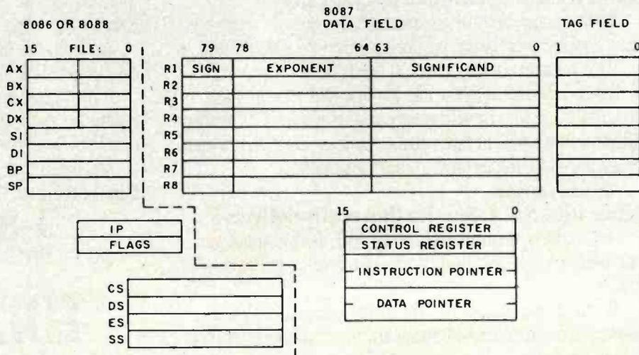
Figure 1: The NDP register set of eight 80-bit registers.
