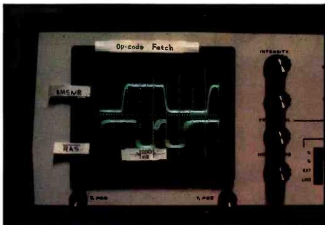
**Photo 4a:** The Z80 clock runs at 3.58 MHz, and the memory clock at 14.5 MHz. An op-code fetch (a short Read with MI high) sets two request flags. The first  $\overline{RAS}$  pulse is the actual op code being fetched, and the one on its heels is a "hidden refresh." The time elapsed for each vertical line on the scope face is 200 ns. The horizontal smear on  $\overline{RAS}$  is the 69-ns latency time of the cycle generator.
