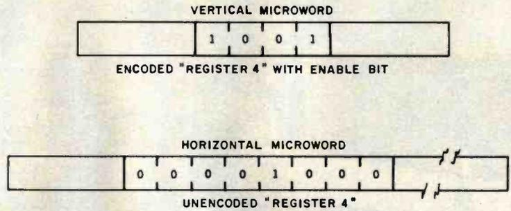
Figure 4: Comparison of horizontal and vertical microcode patterns.
