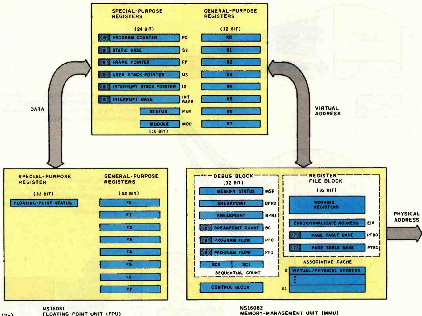
**Figure 3:** Component interconnection in the NS16000 family. Figure 3a shows the logical interconnection of the microprocessor and its memory-management and floating-point units, while figure 3b gives an overview of the physical interconnections.
