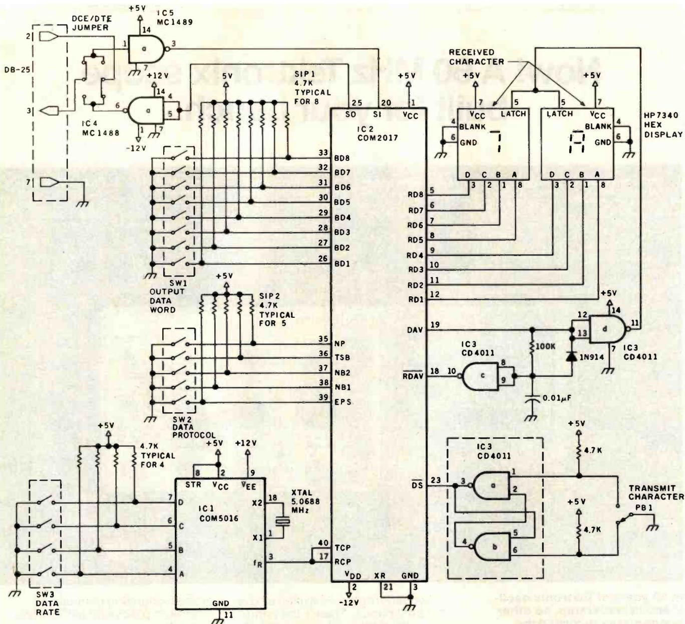
Figure 6: A terminal-simulator circuit used to test the functioning of an RS-232C communication link. This simple-minded device transmits a single, switch-selected ASCII character on demand or receives a single character for display in hexadecimal form.
