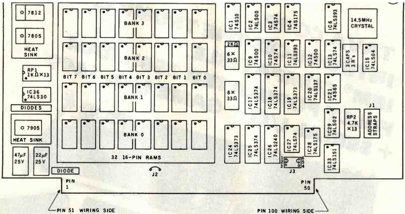
Figure 6: Layout of ICs on wire-wrap circuit card. Note that, in some places, resistors and capacitors are shown in IC-like blocks.
