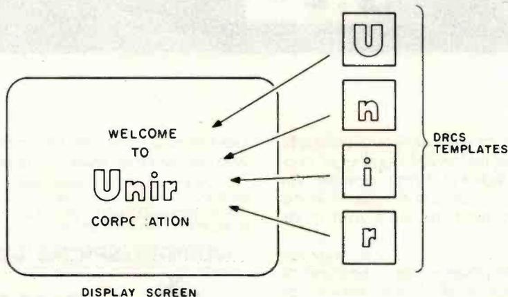
Figure 4: Once a DRCS set has been defined, its characters can be mapped just like text characters onto the display screen.
