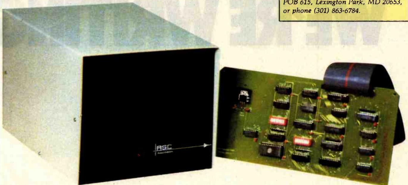
Photo 6: The completed disk subsystem showing the drive assembly and the HCA printed-circuit card.
