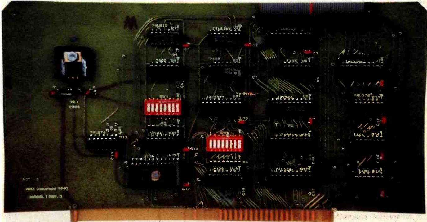
Photo 1: The host computer adapter (HCA) printed-circuit card.
