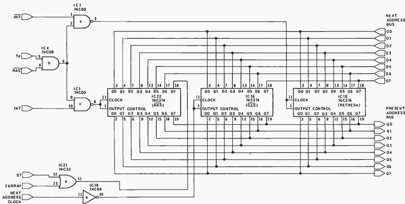
**Figure 3:** This section of the circuit latches the row-address, column-address, and refresh pointers for the Optic RAM addressing. Address registers IC22 and IC16 hold the row and column addresses, respectively, while the third register, IC10, is the refresh register.
