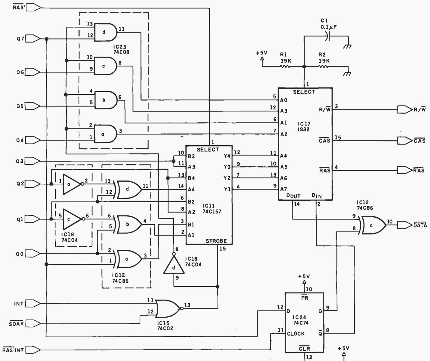
**Figure 4:** Consisting of two inverter sections, three exclusive-OR gates, and a multiplexer, the address-descrambling circuitry undoes the internal address scrambling done by the Optic RAM. The soak circuit makes the Optic RAM light-sensitive by depriving it of refresh cycles.
