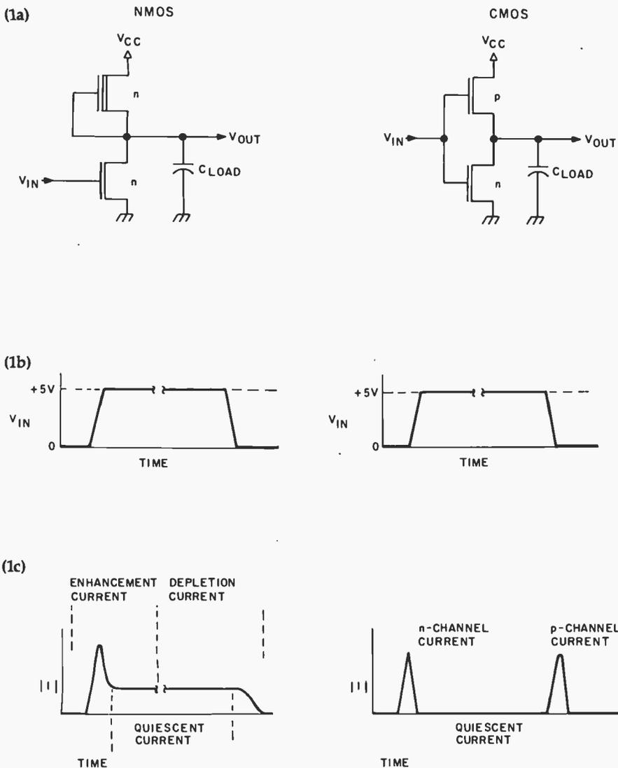
**Figure 1:** A comparison of NMOS and CMOS technologies. Figure 1a shows the schematic diagrams of an inverter as implemented in both NMOS and CMOS. A hypothetical input waveform and the resulting transistor currents are shown in 1b and 1c.
