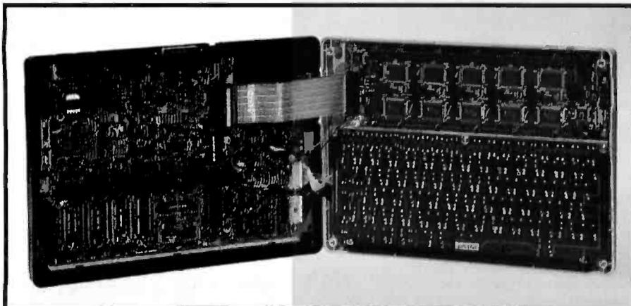
**Photo 2:** Inside the Model 100. The main circuit board is on the left, while the keyboard and liquid-crystal-display boards are on the right. Notice the four slots for additional RAM in the lower left corner of the main circuit board.
