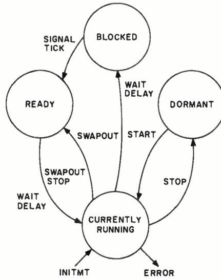
Figure 3: The MTK80 task state diagram.
