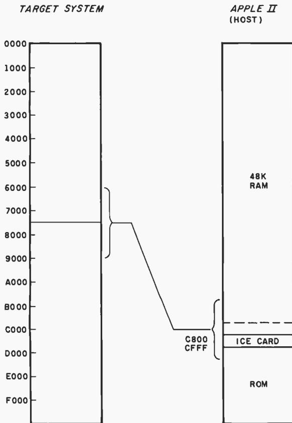
Figure 2: Any 2K-byte block of memory space in the target system can be mapped into the normally empty memory slot from location C800 to CFFF hexadecimal in the Apple.
