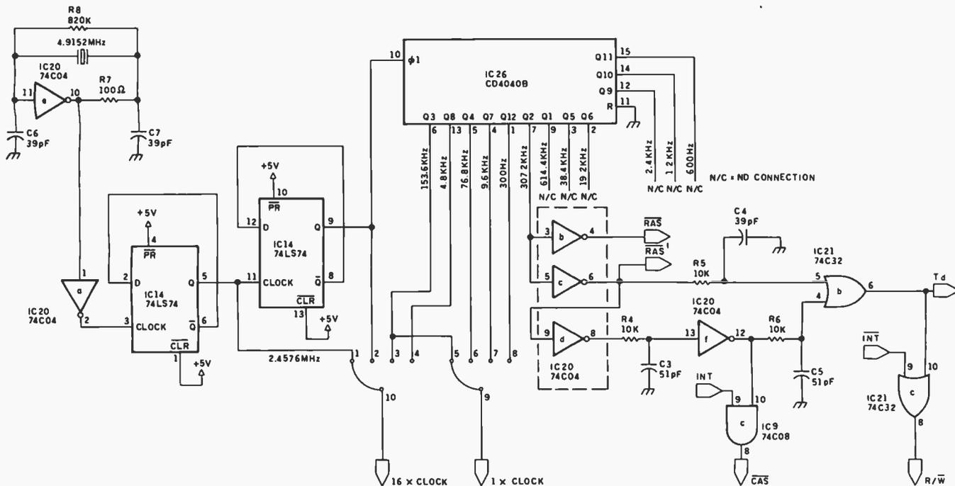
**Figure 1:** A schematic diagram of the timing-generator circuit, which contains a CMOS oscillator circuit to generate the fundamental clock rate. This signal is divided down to produce the frequencies for various possible output data rates and controlling the IS32. The data-rate-clock signals control the sequence of operation of the interrupt generator and the transmitter circuit.
