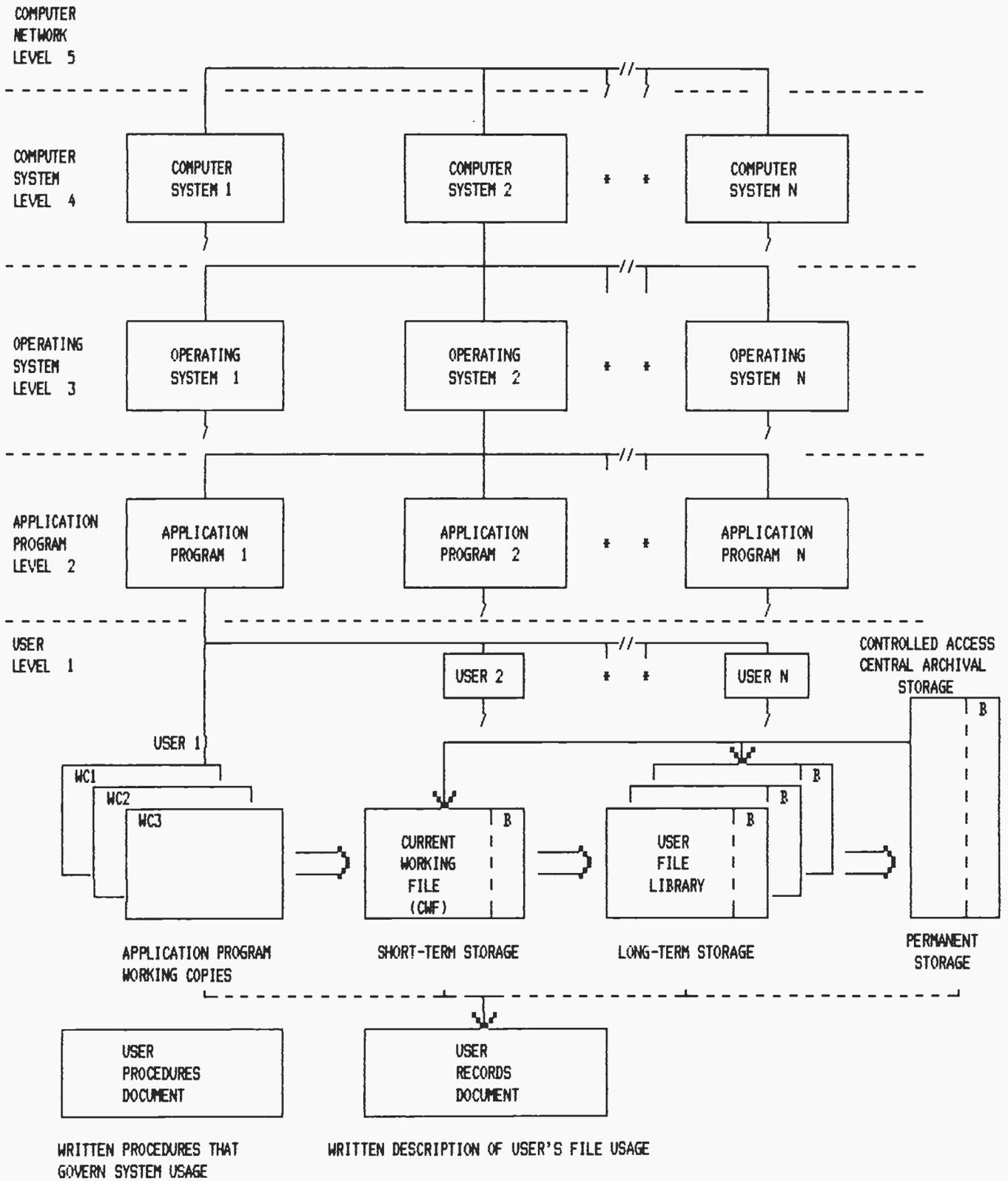
**Figure 1: Data file management system block diagram.** The system is divided into five levels, each with its own procedures for control. You must design your own specific and detailed procedures for maintaining the security of your data files and application programs.
