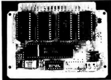
BASIC ON  $\mu$ P — STRINGS, INTERRUPTS, MUCH MORE: HARDWARE 16 BIT MULT AND DIVIDE 37  $\mu$ S. 42  $\mu$ S -VOLTAGE REGULATOR, RS-232C FOR PROGRAMMING, 4K EEPROM (X2816A), 4K RAM, AUTO START PR UP :EXPANSION BOARDS AVAILABLE. MICRO XCPU — \$195 EPROM BURNER VERSION FOR DIE HARDS — \$125
