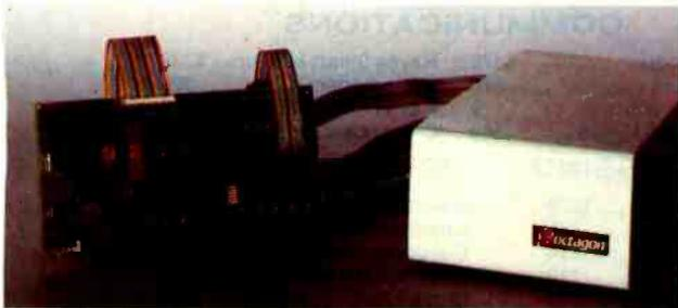
1010 hard disk controller chip to control up to four 5¼" drives, this unique board gives you automatic seek, automatic retries after error; comes with both CP/M 80 and CP/M 86 bios; and includes two serial ports and one Centronics-compatible parallel port.
