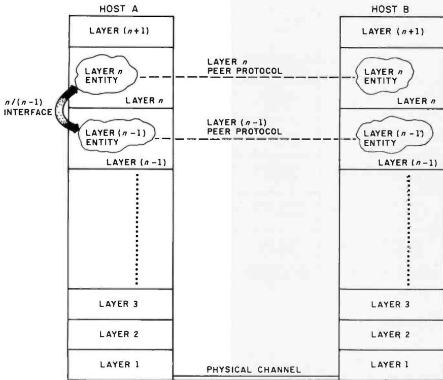
**Figure 1:** A layered networking implementation of two interconnected host computers. Although a given layer (layer *n*) in one computer should communicate with the corresponding layer in the other computer, all communication actually takes place through the physical channel, which employs layer-1 protocol.
