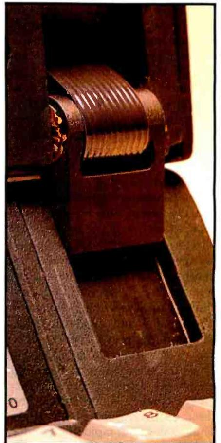
**Photo 2:** Keys to the user-friendliness of the Gavilan's packaging are the two spring-loaded posts and the hinge assemblies that attach the display housing to the computer. The posts permit the housing to form a cover that seals the keyboard when not in use yet rises to lift the display into its operating position.
