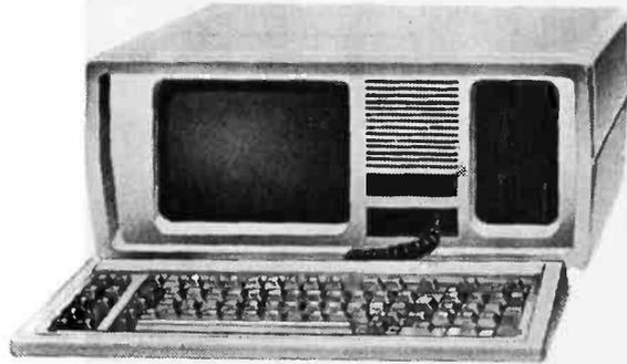
Includes 64K IBM-PC with two 320 KB floppy disk drives, color controller graphics card, monochrome monitor
