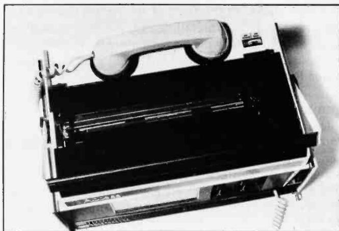
Photo 4: A telephone handset in the acoustic modem cups.
