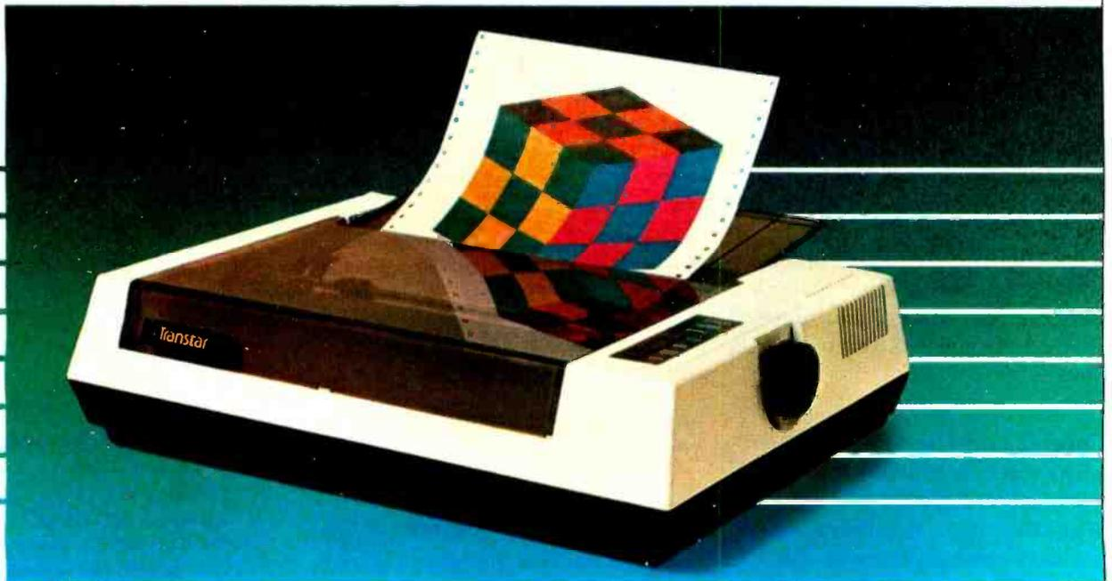
**T**he technology of the all-new Transtar 315 color printer revolutionizes color impact printing! Unlike old-fashioned printers needing multiple passes with pins to print color, the Transtar 315 employs an innovative 4-hammer print head to allow 7 colors and more than 30 shades to be printed in a single pass!
