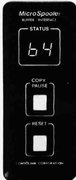
The basic Microspooler contains 16K bytes of memory and an LED display that indicates the amount of memory in use and how much data is yet to be printed. Options include memory expansion of up to 64K bytes and serial interfacing capabilities. The suggested retail price for the parallel-to-parallel interface unit is \$199. For full particulars, contact Consolink, 1840 Industrial Circle, Longmont, CO 80501, (800) 525-6705; in Colorado, (303) 651-2014. Circle 682 on inquiry card.
