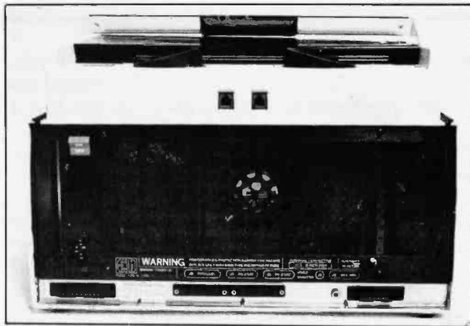
Photo 5: The rear panel of the Access showing (left to right, top): power cord storage compartment, on/off switch, and fan. Bottom panel (left to right): bidirectional parallel port, two RS-232C serial ports, external video monitor jack, and IEEE-488 port.
