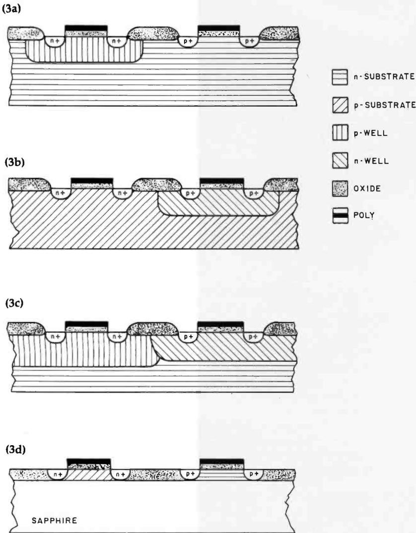
**Figure 3:** Cross sections of transistors formed by each of the four major CMOS processes. Figure 3a is a p-well bulk CMOS transistor; figure 3b shows an n-well bulk device; figure 3c is an example of a twin-tub bulk CMOS transistor; the transistor in figure 3d is formed using silicon-on-sapphire technology.
