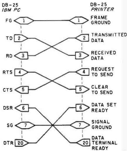
**Figure 1:** A cable must be specially wired to connect the IBM Personal Computer to a printer through an RS-232C serial link. Because both the computer and the printer are set up as data-terminal equipment (DTE), connections must be crossed so that each communicates with data circuit-terminating equipment (DCE).
