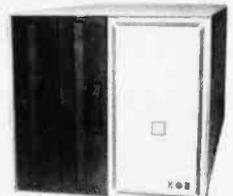
Our most popular computer features a 4 slot S-100 bus and 8" industry standard format. Reads and writes the IBM 3740 format as well as any byte size sector. Expandable? Yes, add a hard disk or cartridge subsystem when your data base grows, includes CP/M operating system.
