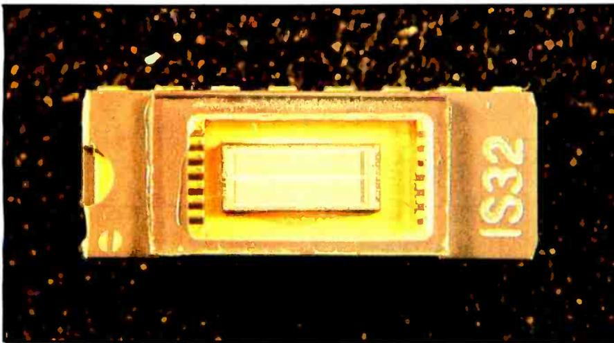
**Photo 4:** The IS32 Optic RAM, a 64K-bit dynamic memory device specially packaged with a quartz lid for optical use in image-sensing applications, is made by Micron Technology Inc., 2805 East Columbia Rd., Boise, ID 83706, (208) 383-4000.
