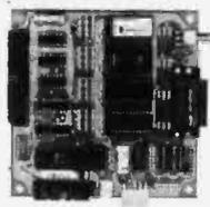
**8051-Based Single-Board Computer with Monitor/Debugger**
