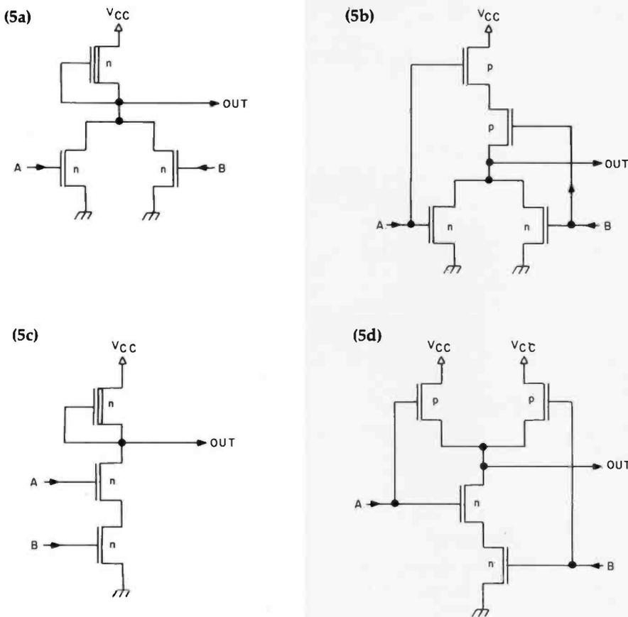
**Figure 5:** A comparison of typical logic gates in NMOS and CMOS form. Figure 5a is an NMOS NOR gate, while figure 5b is a CMOS version; figure 5c is an NMOS NAND gate, and figure 5d is a CMOS version.
