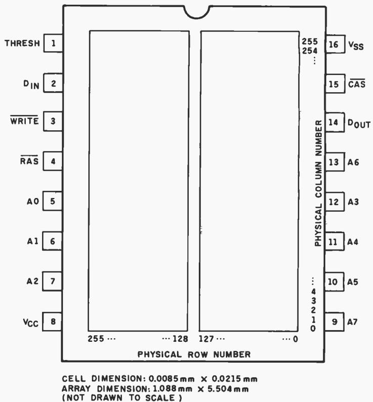
**Figure 7:** A diagram of the topology and pinout configuration of the IS32 Optic RAM (not to scale). Each of the two cell regions, visible through the quartz package lid, contains a 128-by 256-cell array.
