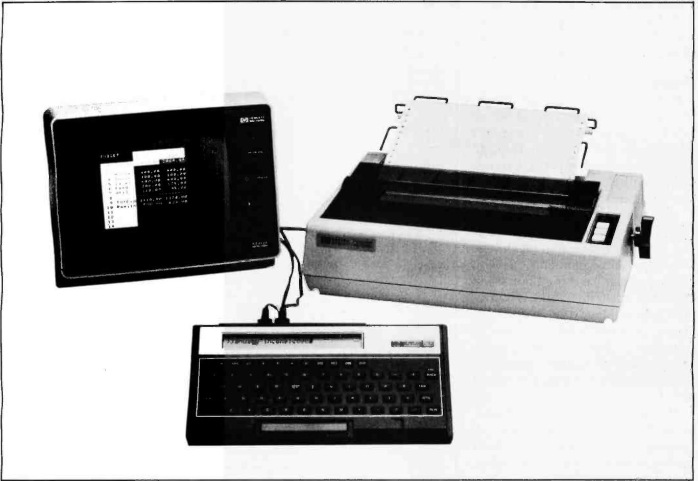
Photo 1: Visicalc spreadsheets can be viewed on the HP-75's single-line display, on a video monitor, or on printouts.
