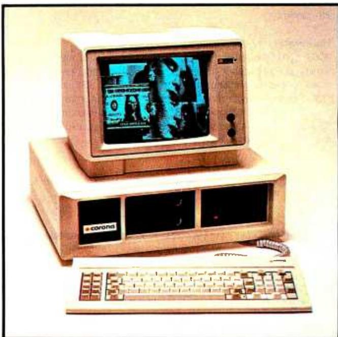
Photo 2: The Corona PC, the desktop version of the Corona portable. The unit shown here has half-height floppy-disk drives, but most units will be shipped with regular-height drives.
