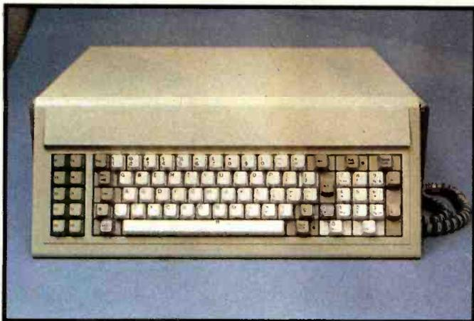
**Photo 6:** The Corona's keyboard, which was produced by Key Tronic. Again, note the similarity to that of the IBM. Also note that future editions of the Corona will have some keys repositioned, specifically the left Shift key and the Return key.
