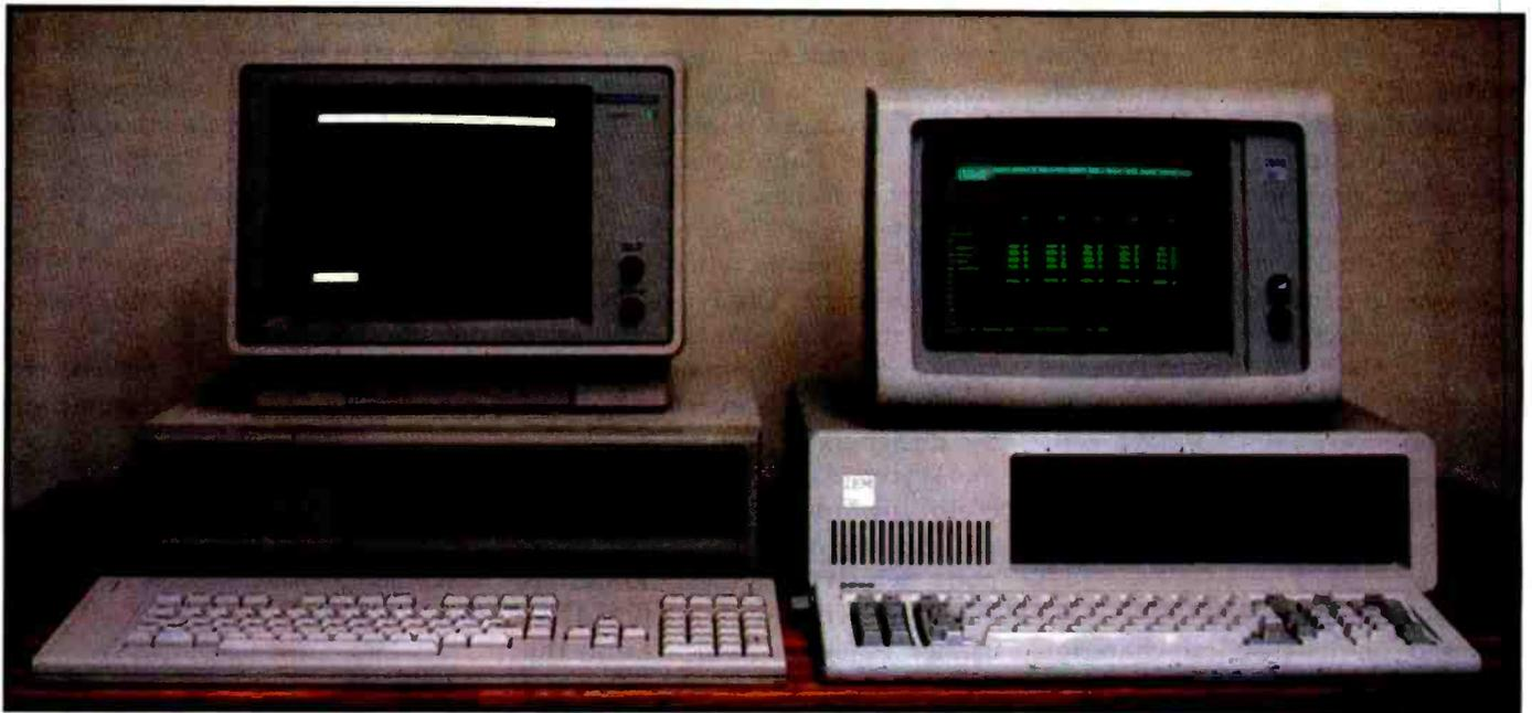
**Photo 2:** Compare the TI and IBM video displays. Although the TI display is easier to read, it looks faded when compared to the IBM display. The contrast and brightness controls were adjusted on both screens to give the best picture (photo by Randy Bullard).
