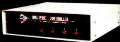
**BTA's MODEL 524 MULTIPORT CONTROLLER** is a code activated one to four serial port expander — but that's not all since it has separate and independent UARTS, buffers and handshaking each port can operate with a different configuration, i.e. different baud rates, stop bits, etc. These features also permit two or more devices to communicate with the 524 simultaneously.
