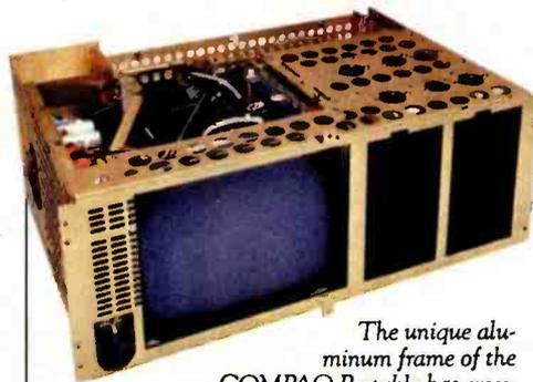
*The unique aluminum frame of the COMPAQ Portable has cross-members that strengthen it front-to-back, side-to-side, and top-to-bottom. It's a design practice commonly used in race cars.*
