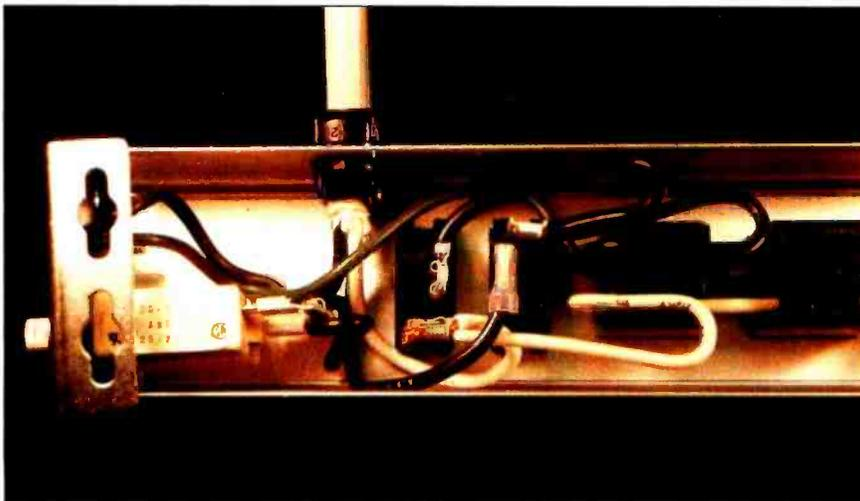
Photo 3: An internal view of the Radio Shack six-outlet power strip. Power enters through the white cord and travels through the switch and a 15-A circuit breaker to the outlets.
