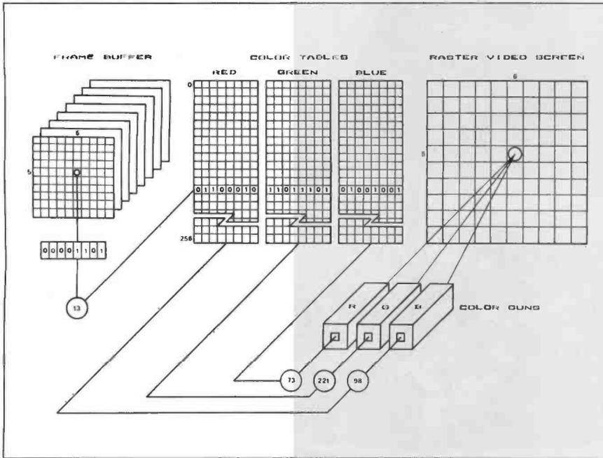
Figure 2: Configuration of a frame buffer or video-display memory with eight bit planes driving the RGB color guns through color tables 8 bits wide by 256 bytes long. The dimensions of both the frame buffer and the raster video screen have been simplified in this diagram for clarity.
