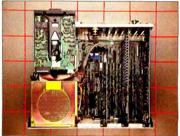
The inside of the Leading Edge. The disk drives are at the upper left (front) of the machine.
