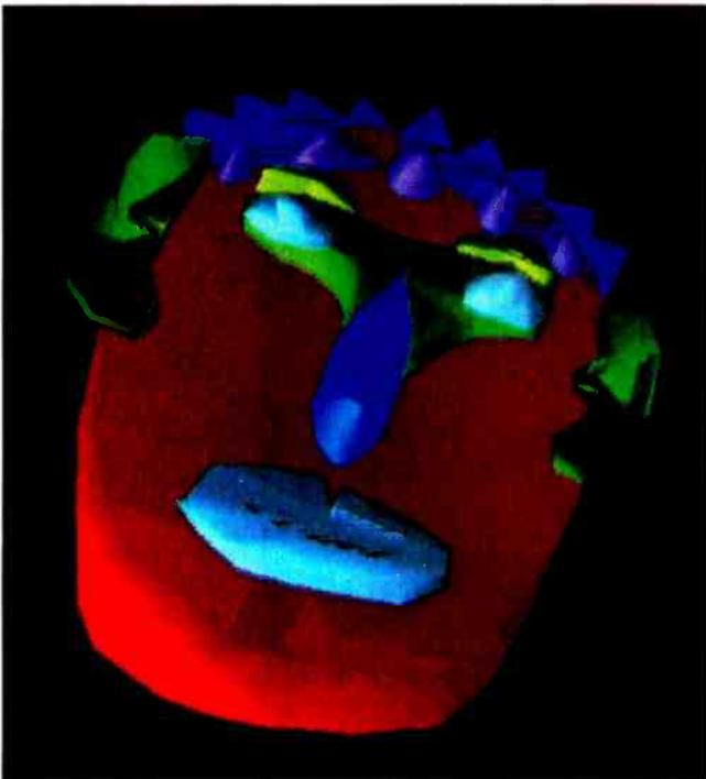
Photo 1a: Front view of "Mask.1," a three-dimensional object with hidden surfaces removed and rendered with smooth shading. The mask is made of 16 simple pieces assembled together (a total of 858 polygons) and was digitized from freehand drawing. All images are copyright © 1984 Isaac Victor Kerlow.
