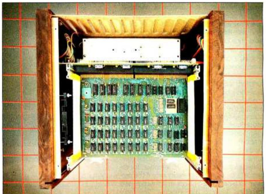
Photo 2: Top view of the Lilith system unit with its front panel removed.
