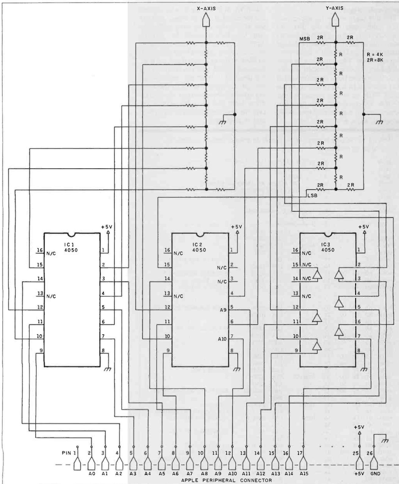
Figure 3: The D/A converter schematic diagram.
