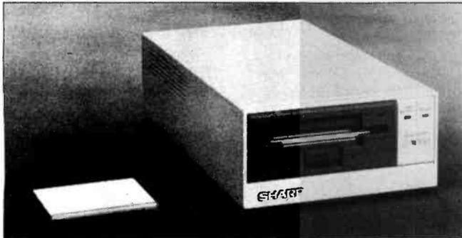
The CE-513F is a portable microfloppy-disk drive for Sharp Electronics' PC-5000 portable computer. Weighing 6 pounds and measuring 5½ by 2½ by 8½ inches, the CE-513F adds 360K bytes of formatted storage (500K unformatted) to the 128K bytes of bubble memory built into the PC-5000.
