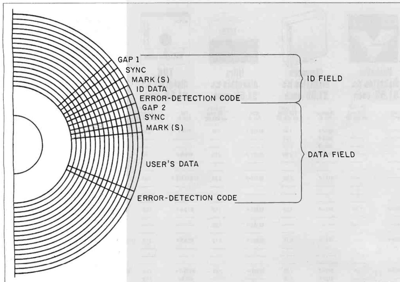
Figure 1: The typical sector composition of a floppy disk. In soft sectoring, each distinct radial slice is divided into an ID field and a data field. Usually, the data field contains from 128 to 1024 bytes of data and is the most important part of the sector.
