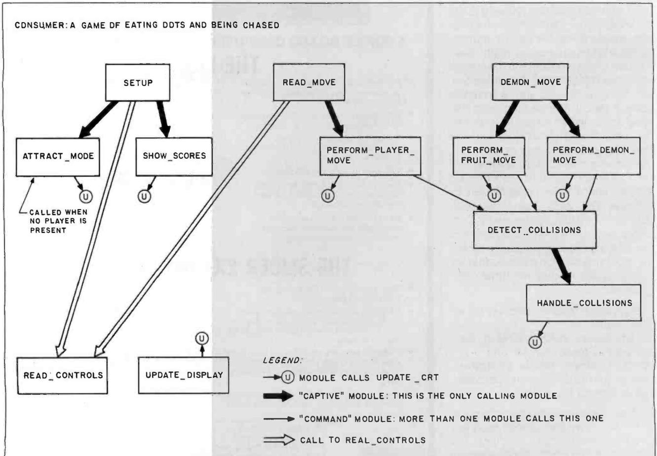
Figure 1: A structure diagram for Consumer. This is not the only "correct" version: many different organizational strategies would work just as well. Note that the higher a module appears in the diagram, the closer to the root module its priority.
