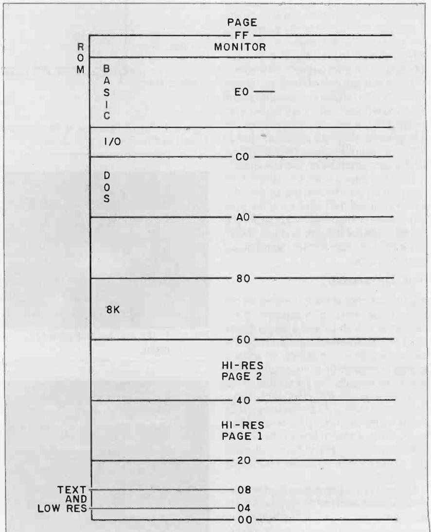
Figure 2: The y-axis paper scale used to label the Apple II+ memory-location display.
