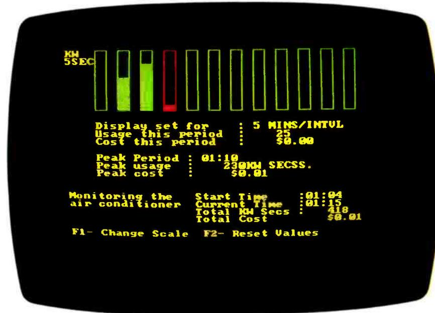
Photo 8: Monitoring software in operation, demonstrating the power consumed by an air conditioner over a predetermined interval. Time starts from left to right. In this example, each rectangle represents 5 minutes. The current time is indicated by the red block, and increasing consumption is registered in real time for the current period and for total elapsed time. After 15 minutes, \$0.01 has been consumed.
