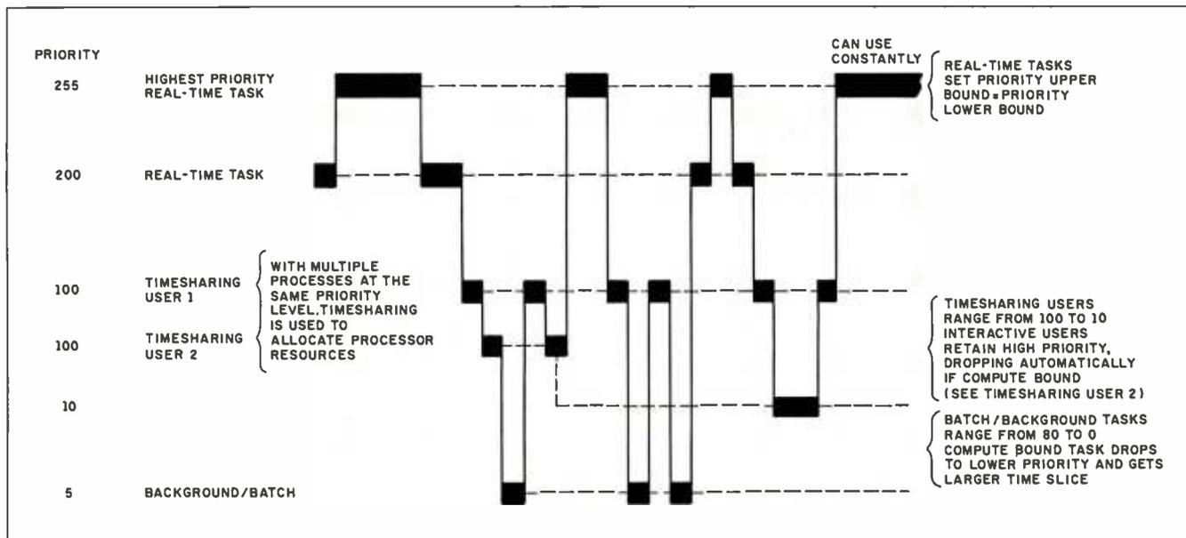
Figure A: An example of task scheduling by the UNOS operating system.
