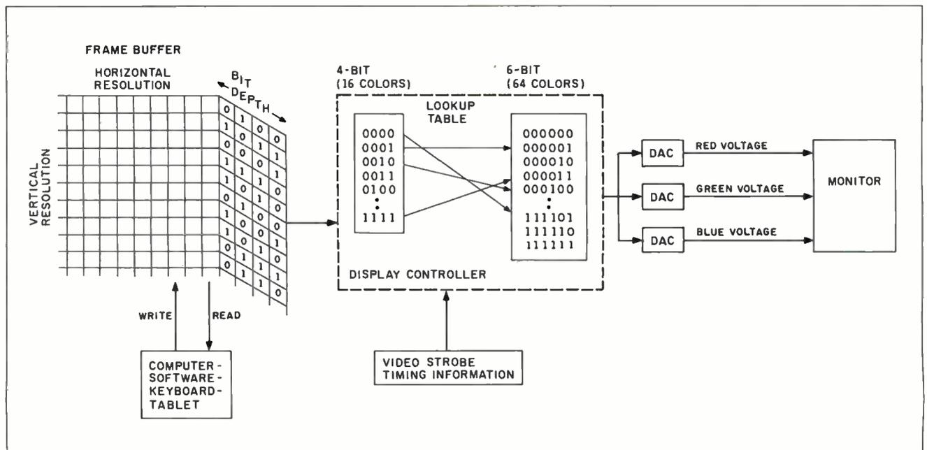
Figure 10: Basic graphics hardware architecture.
