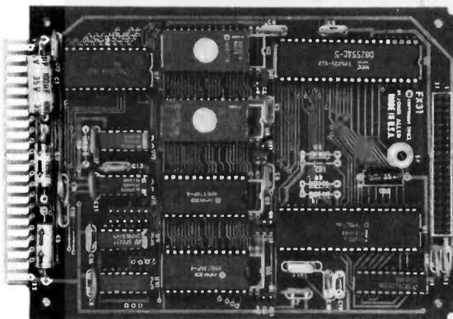
connector brings out the four parallel ports, TTL and RS-232C serial data, and a +5-V ground.
