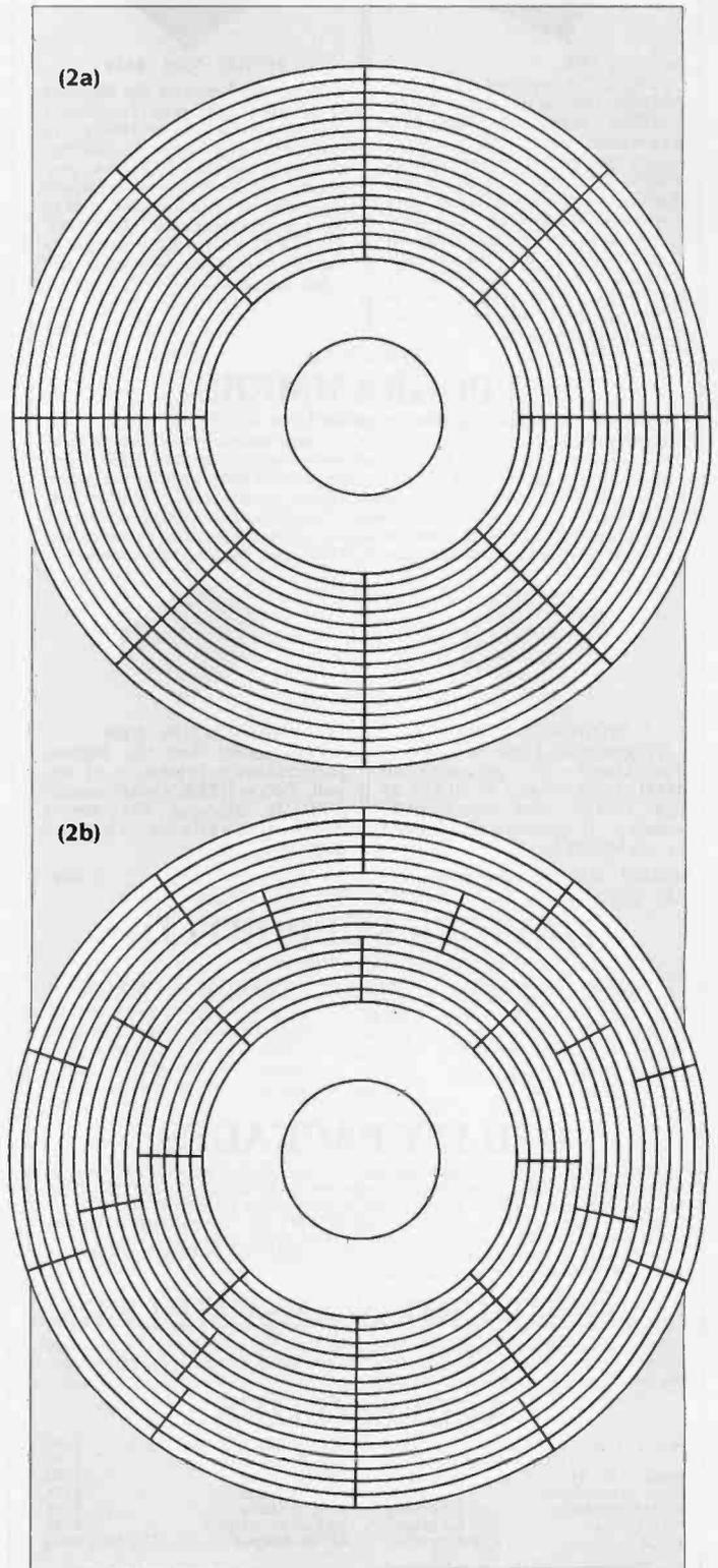
Figure 2: A typical eight-sector layout with radius sectors (a). Sector layout traditionally focused on the pie cut. Newer methods involving fixed-bit-cell sectors (b) enable a disk to hold up to 40 percent more data.
