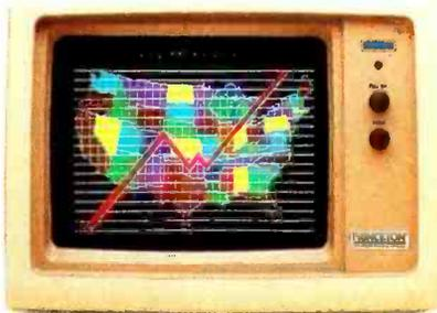
At first glance, the SR-12 might appear similar to the HX-12 with a non-glare screen and .31mm dot pitch supporting 690 horizontal resolution. But take a closer look. SR-12's scan frequency is 31.5 KHz, allowing the SR-12 to support 480 vertical resolution in non-interlaced mode. That means a high-quality, flickerless image with text that's up to monochrome standards. What's more, you get all that quality for \$799.
