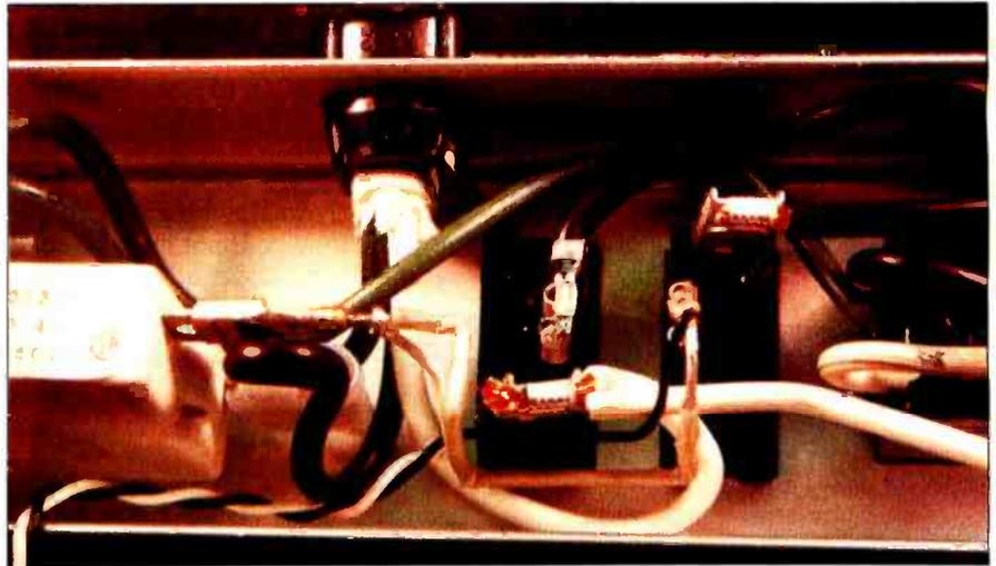
Photo 4: The wire from the hot side of the breaker (black wire) to the switch is replaced with the paper clip sensing resistor. Notice how it is bent to fit the enclosure. It is insulated with heat-shrink tubing. The sensing wires (#22 black-and-white) are connected to the power-monitor electronics.
