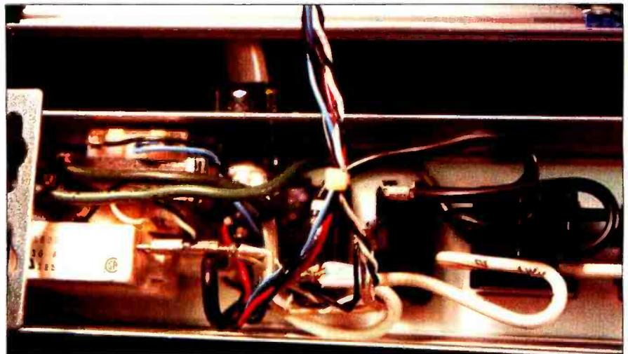
Photo 5: A 12.6-V AC, 300-mA transformer is inserted and secured within the case next to the circuit breaker. Its output is also connected to the power-monitor electronics.
