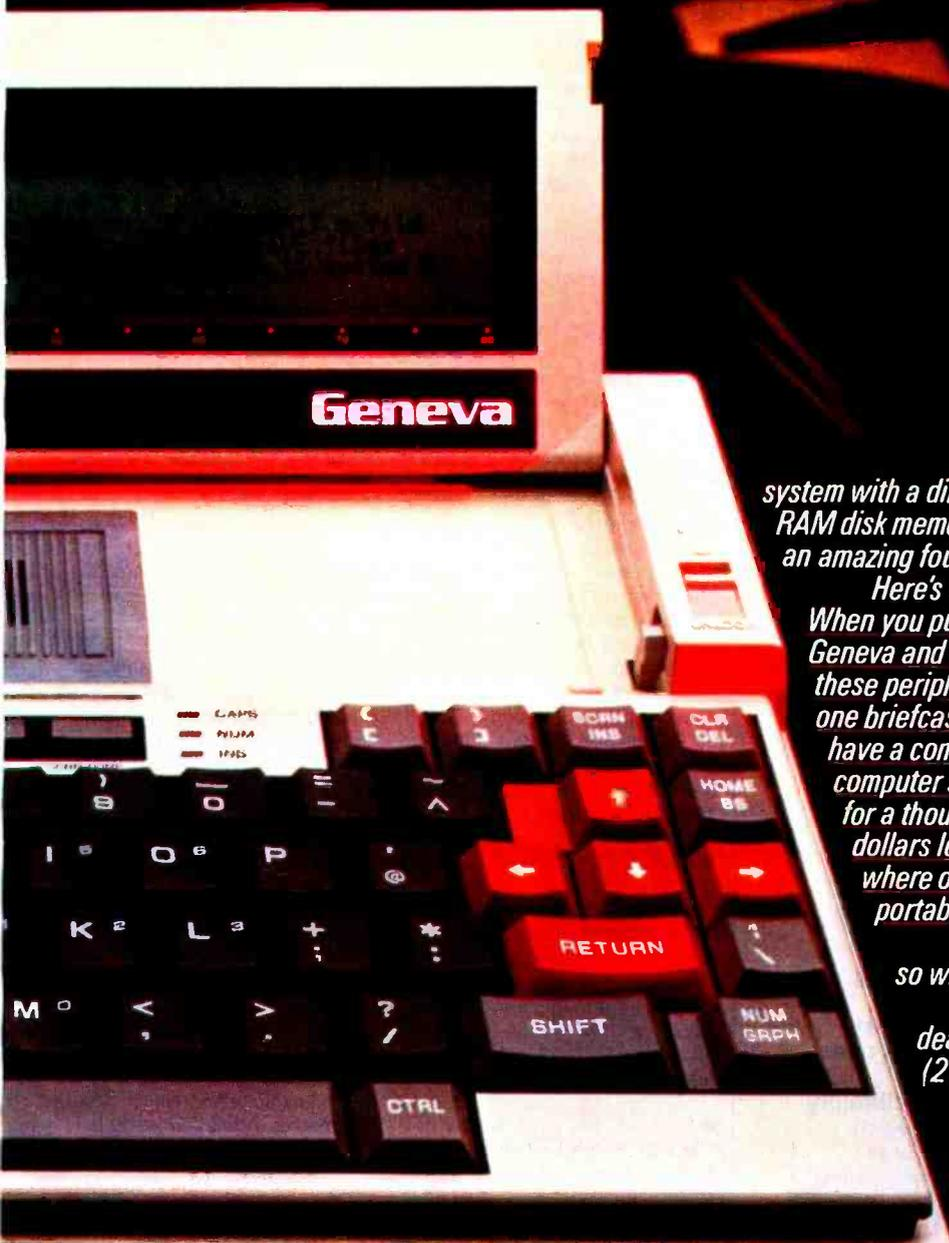
system with a direct connect modem; an extra 120K of RAM disk memory; a 320K 3 1/2" disk drive; there's even an amazing four pound 80-column printer.
