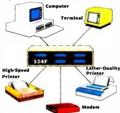
BayTech's versatile networking multiports, capable of any-port-to-any-port interconnection, have virtually unlimited applications. With their features and low cost, the user can create a local network providing simultaneous communication for 5, 9, or 18 RS-232C devices.
