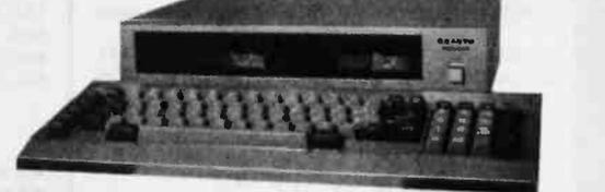
The Sanyo MBC-550 Microcomputer includes 128K byte of memory, a 5 1/4" disk drive along with a parallel printer port. The computer outputs both RGB color and monochrome composite video. Extensive software such as Sanyo Basic, Wordstar, Calcstar and Easy Writer I is included with the MBC-550.
