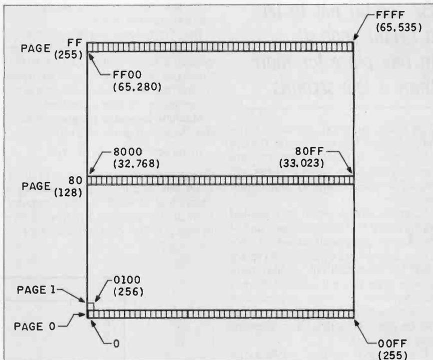
Figure 1: The configuration of the memory-display array. Locations are given in hexadecimal and parenthetically in decimal.
