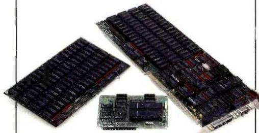
Memory Sockets For Adding Up To 4 Megabytes • 1 Standard and 3 Optional Serial Communications Ports • Parallel Printer Port • Game Port Option
