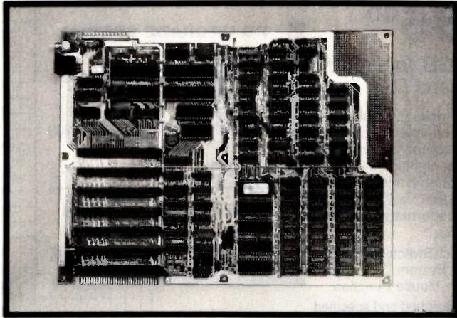
THE **MEGA-BOARD™-XT**, FULLY ASSEMBLED AND TESTED WITH 256K RAM, IS 100% HARDWARE COMPATIBLE THERE IS A HARDWARE RESET SWITCH AND WIREWRAP AREA FOR CUSTOM APPLICATIONS.
