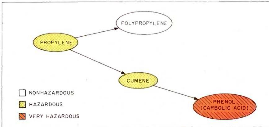
Figure 1: The propylene-phenol production chain.
