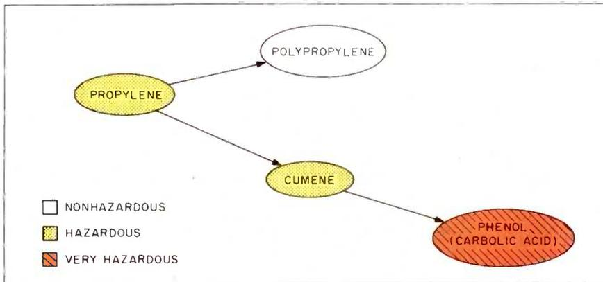
Figure 1: The propylene-phenol production chain.
