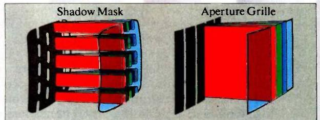
With a Fine Pitch Aperture Grille, Trinitron monitors give you dramatically brighter colors than the conventional shadow mask.
