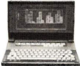
MORROW PIVOT II Portable 14 Lb., w/ 4HR Battery, 640 X 200 Luminescent Screen, 256K or 640K, 2X5 1/4" FLPYS, S.P, RGB/COMPST & Expansion Chassis Ports, 1200 Baud Modem, PC Compatibility w/MS-DOS 2.11 and GSS-VDI for PC Graphics Devices, CLK-CAL w/appointment Scheduler & Calculator from \$1,995
