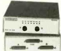
Get all the outstanding features of DATA SPEC's RS232 25 Pin Data Switch Boxes and more with the ABL-25LE. This luxury edition data switch box features 7 L.E.D. indicators (TD, RD, RTS, CTS, DSR, DTR & CD) and gold plated pins.
