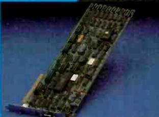
High res color and monochrome video controllers are fully interfaced with system.
