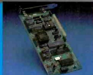
AT compatible disk controller handles 2 floppies, 2 Winchester's.
