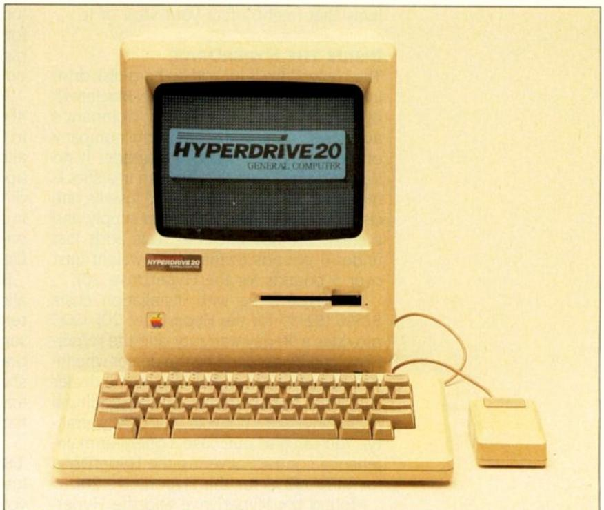
Photo 1: A Macintosh computer with a GCC HyperDrive 20 20-megabyte hard disk in it.
