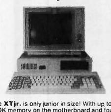
The **XTjr.** is only junior in size! With up to 640K memory on the motherboard and four expansion slots, this stand-alone system is also great for workstations in a networking environment. It can be upgraded to the **TURBO** two speed motherboard and you can also add up to 2 serial & 2 parallel ports or any IBM compatible expansion card. A perfect word processing/data entry system.
