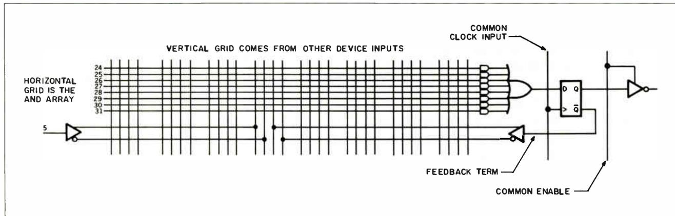
Figure 7: Clocked logic cell from a 16R4 PAL.
