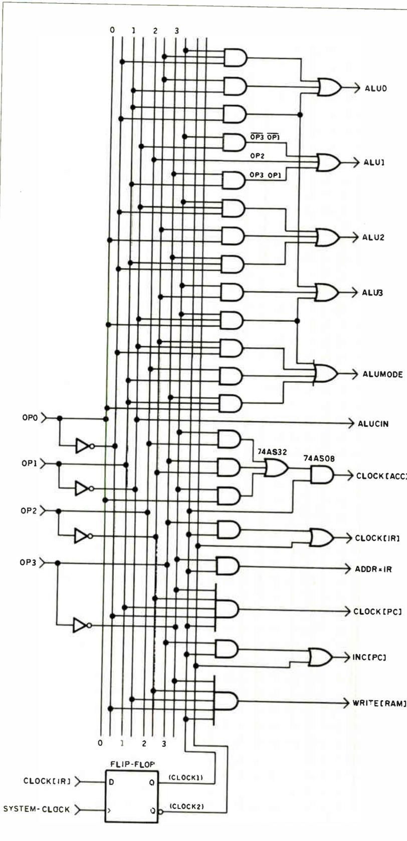
Figure 3: Hard-wired controller schematic. Note that none of the ALU signals depend on whether the controller is in the CLOCK1 or CLOCK2 mode.
