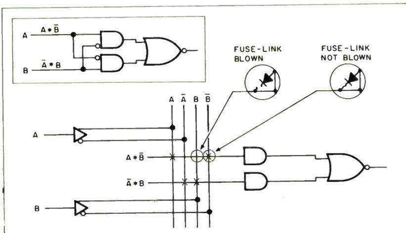
**Figure D:** The PAL device implementation of the function  $/Output = A \cdot B + /A \cdot B$ . The standard combinatorial logic diagram of the function  $/Output = A \cdot B + /A \cdot B$  is shown in the inset to figure D above.
