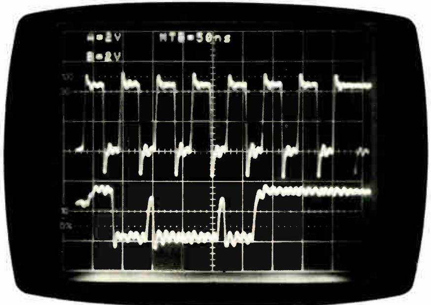
**Photo 1:** The AS output of the DPORT20 PAL. The top trace is the Q0 input; the bottom trace is the AS output. Notice the 9-ns-wide glitches in the AS output between Q0 counts 4 and 5 and counts 8 and 9.
