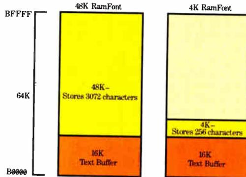
The new RamFont mode displays 3072 programmable characters at the speed of text mode, or replaces the standard character set with one of your choice in 4K RamFont mode.
