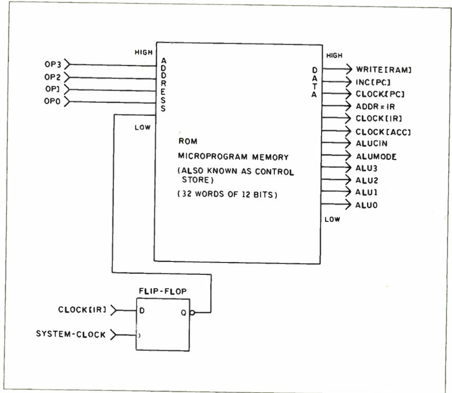
Figure 6: Microcoded controller schematic.
