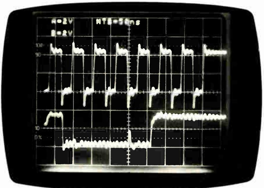
**Photo 2:** Glitching of the AS output of the DPORT20 PAL implemented in a 16L8B device occurs only between counts 7 and 8.
