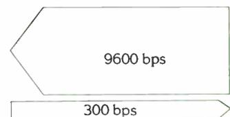
*Courier HST divides the frequency bandwidth of a dial-up phone channel into non-overlapping high-speed and low-speed carriers.*
