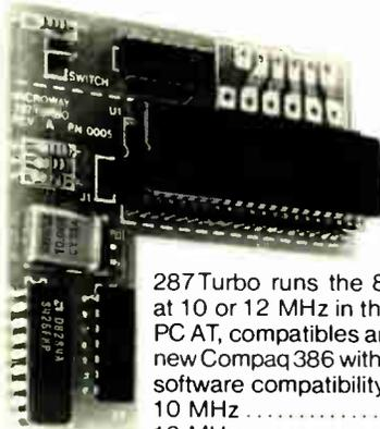
287 Turbo runs the 80287 at 10 or 12 MHz in the IBM PC AT, compatibles and the new Compaq 386 with 100% software compatibility.
