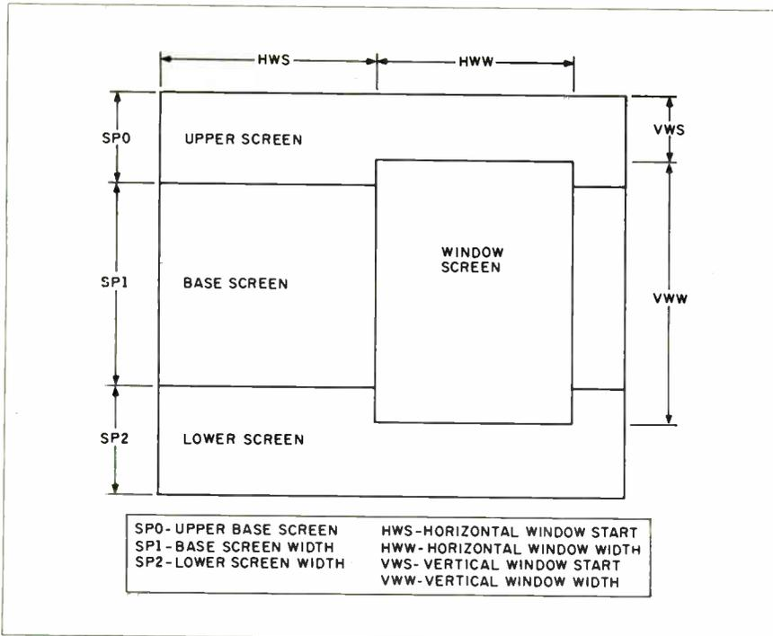
**Figure 1:** Besides establishing basic CRT timing, the timing control registers partition the screen into the upper, base, lower, and window portions. The upper, lower, and base screens are all background screens that are overlapped by the foreground window. The vertical specifications (SP0, SP1, SP2, VWS, and VWW) are in units of rasters, while horizontal specifications (HWS, HWW) are in units of display cycles. Usually, only the base (covering the entire CRT screen) need be defined.
