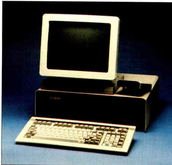
The system also includes a real-time clock with battery backup power, 10 RS-232C serial ports, and a Centronics parallel port. The serial ports use RJ-11 (telephone-type) jacks, which are much more compact and easier to connect and disconnect than the more traditional DB-25 connectors.
