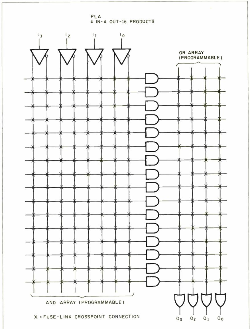
**Figure 2:** A simplified diagram of a PLA showing that both arrays are programmable.
