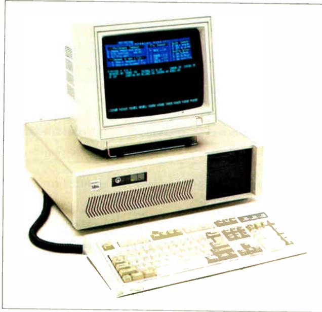
The Kaypro 386 runs on a 16-MHz 80386 microprocessor.
