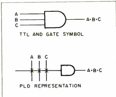
**Figure A:** Differences in the logic notation for a TTL AND gate and a PLD AND gate.
