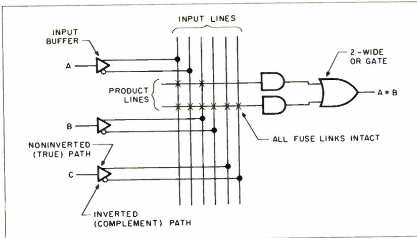
**Figure C:** Portion of the PLD array programmed to implement  $A \cdot B$ . Having all fuses intact in the second product line causes a logic zero to be input to the second AND gate, which does not contribute to the sum at the OR gate.
