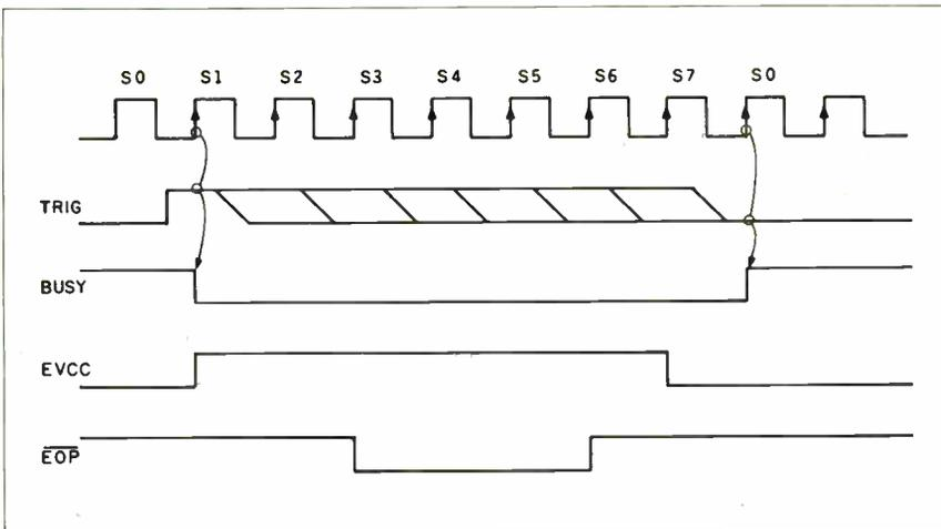
**Figure 7: Timing waveforms of PAL-2, finite state machine.**
