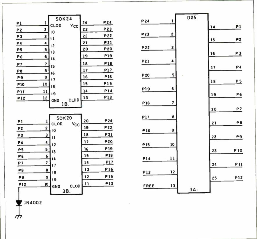
Figure 2: Schematic for the socket board.
