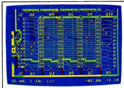
2" by 4" section of a 10" by 16" double-sided board with silkscreen layer
