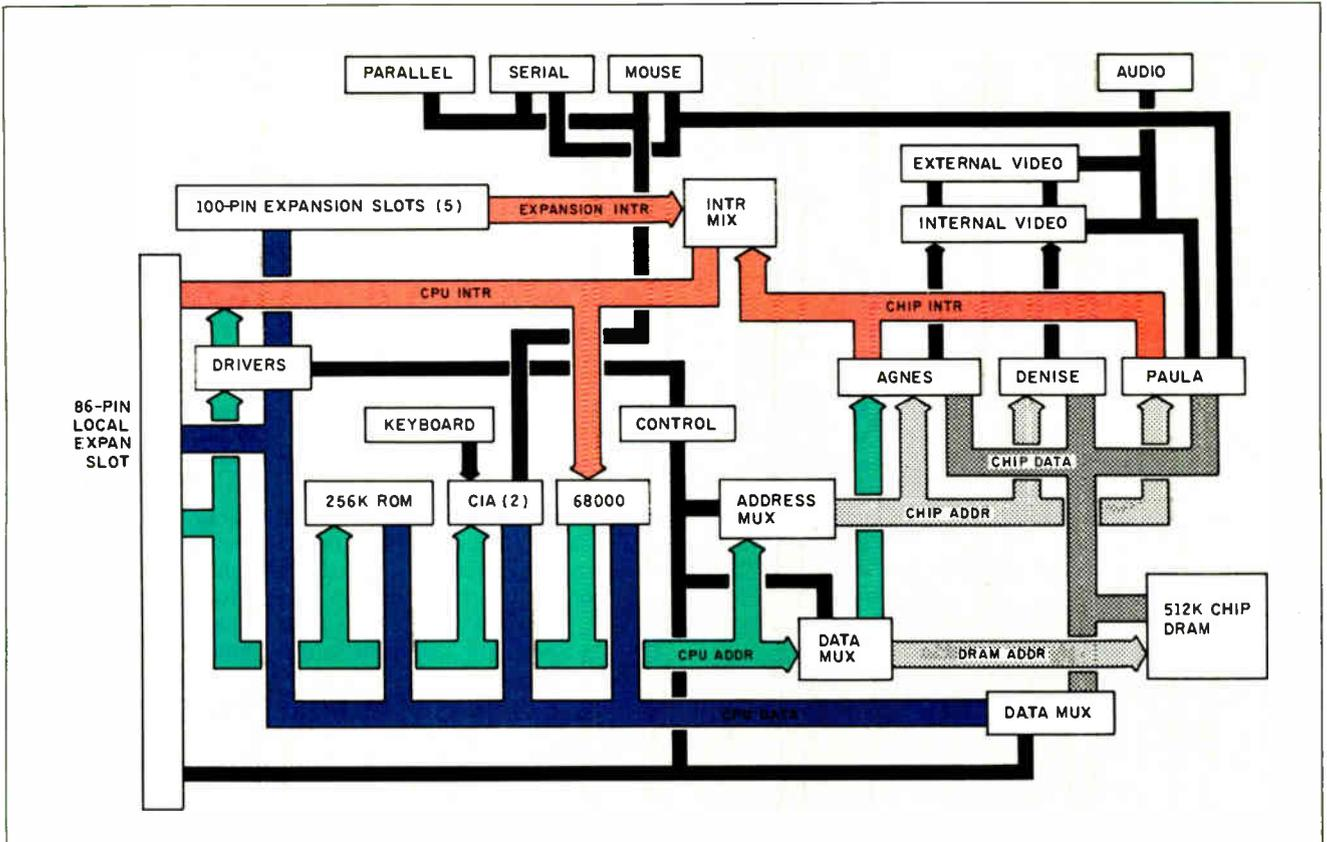
Figure 1: A detailed block diagram of the Amiga 2000.
