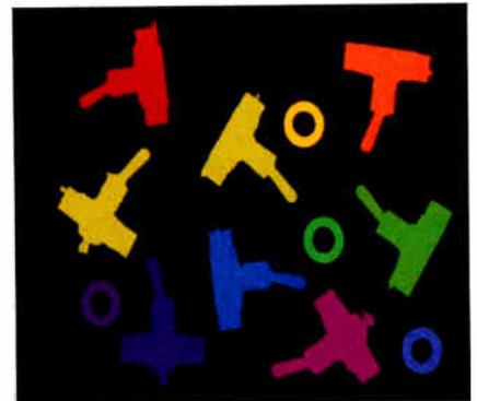
**Photo 18:** The various objects in photo 17 have been labeled with different pixel values. Lookup tables were then used to show the different values in color, a technique known as pseudocoloring.
