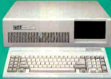
Includes 80286-Based 8MHZ unit, AMI BIOS, 512K on 1MB Mother Board, 1.2 MB Floppy Drive, W.D. Hard/Floppy Controller, Clock/Calendar W/Battery Back Up, AT Style Keyboard, 200-W Power Supply, MS DOS3.1 W/Manual, System Manuals, Full 18 Months Warranty, Run all major software for IBM-PC/AT™
