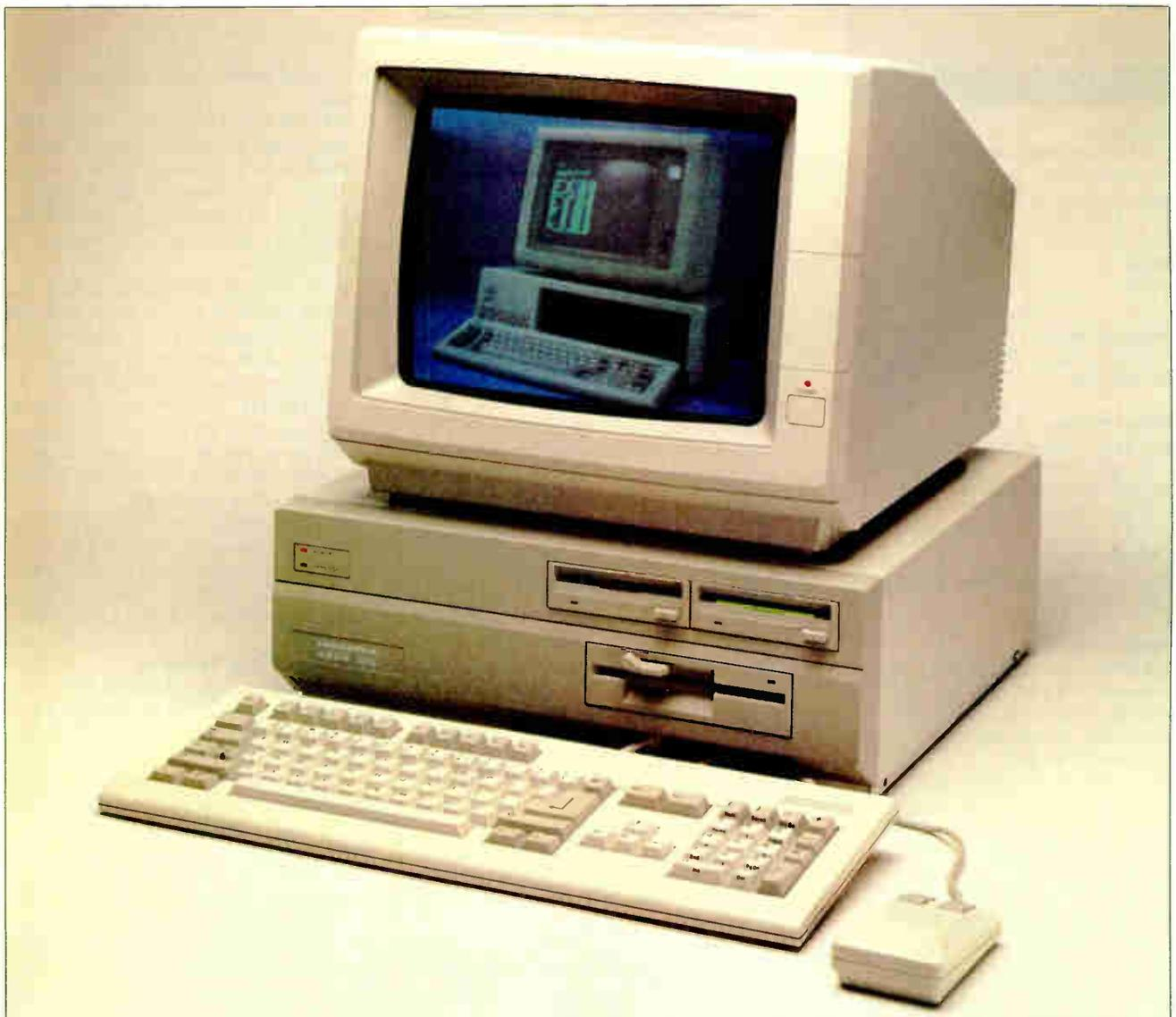
**Photo 1:** The Amiga A2000 computer. The A2000 comes with 1 megabyte of memory and one 3½-inch floppy disk drive. You can also substitute internal hard disks for the second (left) 3½-inch and the 5¼-inch drives that are installed in this machine. The image of the IBM PC shown on the screen was captured using NewTek's Digi-View software.
