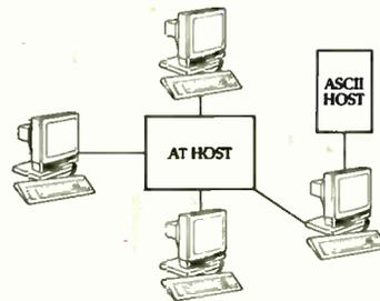
*The PC Station is the only terminal of its kind with dual-host capability, which allows it to be connected to a mainframe host and an AT host simultaneously.*
