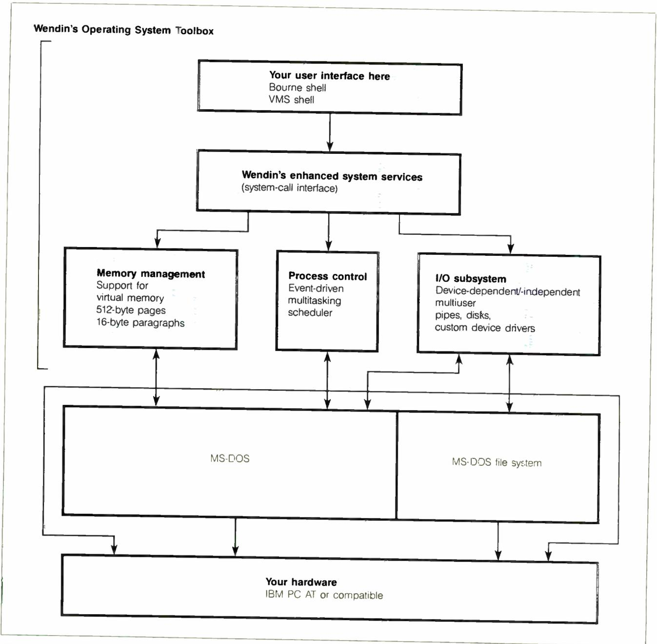
**Figure 1:** An overview of a personal operating system built with Wendin's Operating System Toolbox. The Toolbox uses MS-DOS system calls to a great extent, but it also interacts directly with the hardware.
