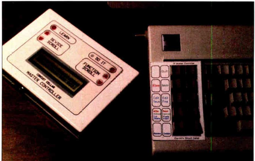
Photo 4: The Master Controller and the IBM PC keyboard showing the MASTER program function-key template.
