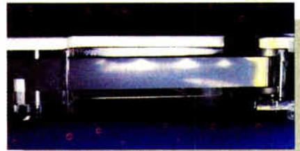
High speed tape seldom enters tape guides parallel to the top and bottom, even with improvements to the tape reel hub designs. The edge pressures which result create "scalping" or "coining" on the tape. The effect is data loss due to head-to-tape separation, flaking media that smears across the head, and "redeposit nodules" that create hard errors.
