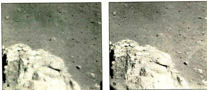
**Photo 3:** Deconvolution, a technique developed during the Ranger missions, involves measuring a camera's tendency to blur high-frequency details and subtracting it from the transmitted images, as shown in these before (a) and after (b) images from a later Surveyor mission.
