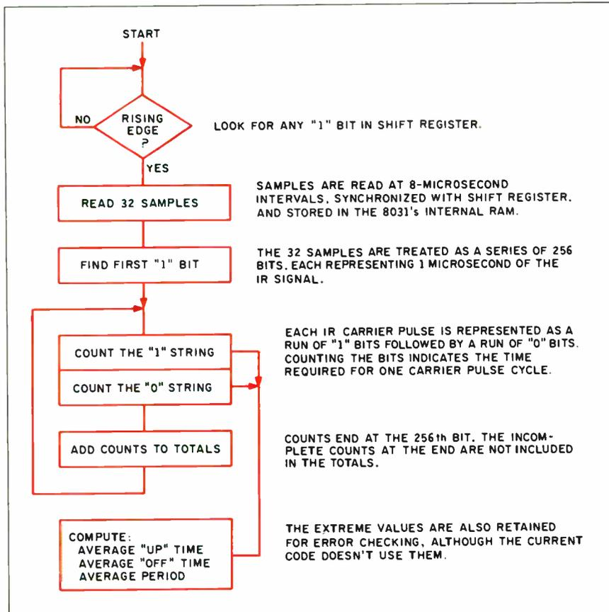
Figure 2: Carrier-frequency measurement flowchart.
