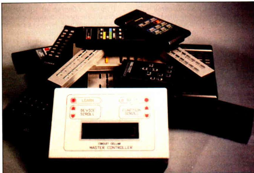
**Photo 1:** The six-button Master Controller can duplicate the functions of the 14 controllers shown in the background.
