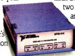
Our RS Converter bridges the electronic gap between RS-232/422 and IEEE-488. You can use it to control your lab's GPIB network via your computer's RS-232/422 port. Or to control RS-232/422 devices via an IEEE-488 bus. Each Bus Converter comes with two full duplex serial ports and a 2K to 32K byte data buffer for maximum throughput. All switches and connections are external—you never have to open the unit. Just hook-up the appropriate devices and the system is ready.
