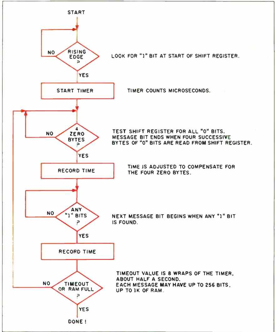
Figure 3: Signal-capture flowchart.
