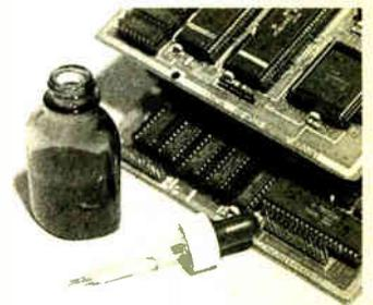
port, a peripheral expansion bus, three bi-directional parallel ports and an industry standard 765A-compatible disk controller for up to four disk drives (any combination of 3 1/2", 5 1/4" or 8" drives). An on-board SCSI expansion bus lets you connect directly to a hard disk drive or additional computers.
