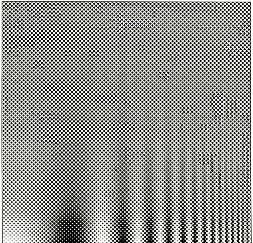
**Figure 4b:** Sinusoidal grating printed at 18.75 cells per inch on a LaserWriter Plus.
