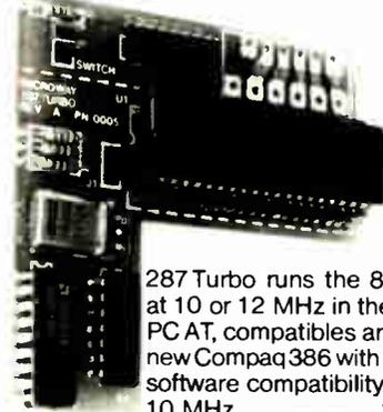
287 Turbo runs the 80287 at 10 or 12 MHz in the IBM PC AT, compatibles and the new Compaq 386 with 100% software compatibility.
