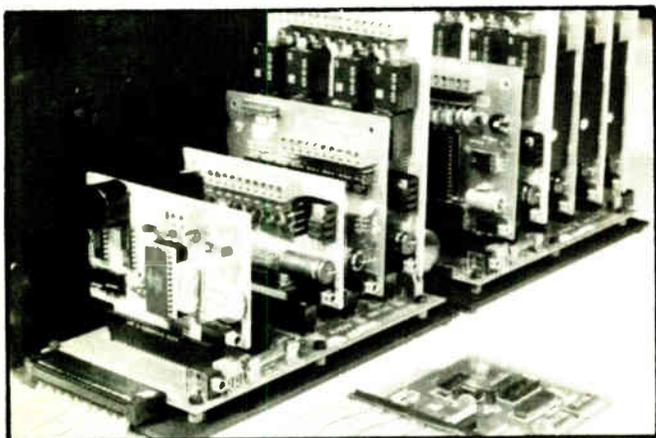
An A-BUS system with two Motherboards
