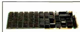
Logic (AST Compatible) AT Multifunction Board w/128K (Expandable to 2.0 Mb) . . . 209
