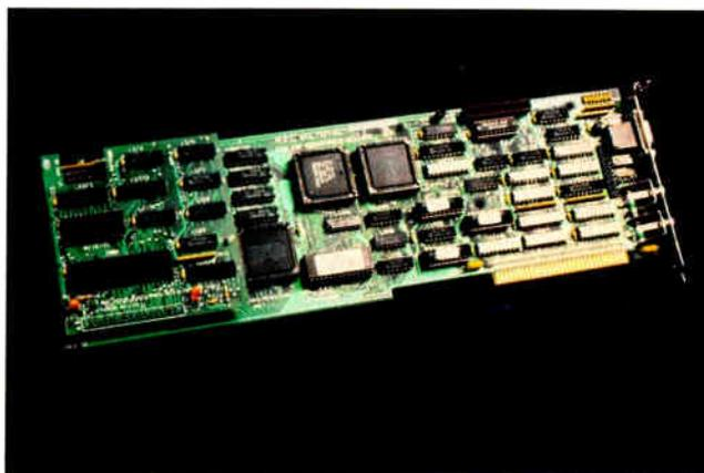
*MultiSync board for the MultiSync monitor.*
