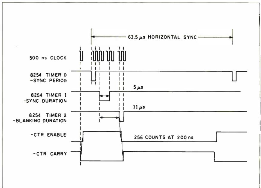
Figure 6: Timing pulses generated by the display/receiver's 8254 PIT.
