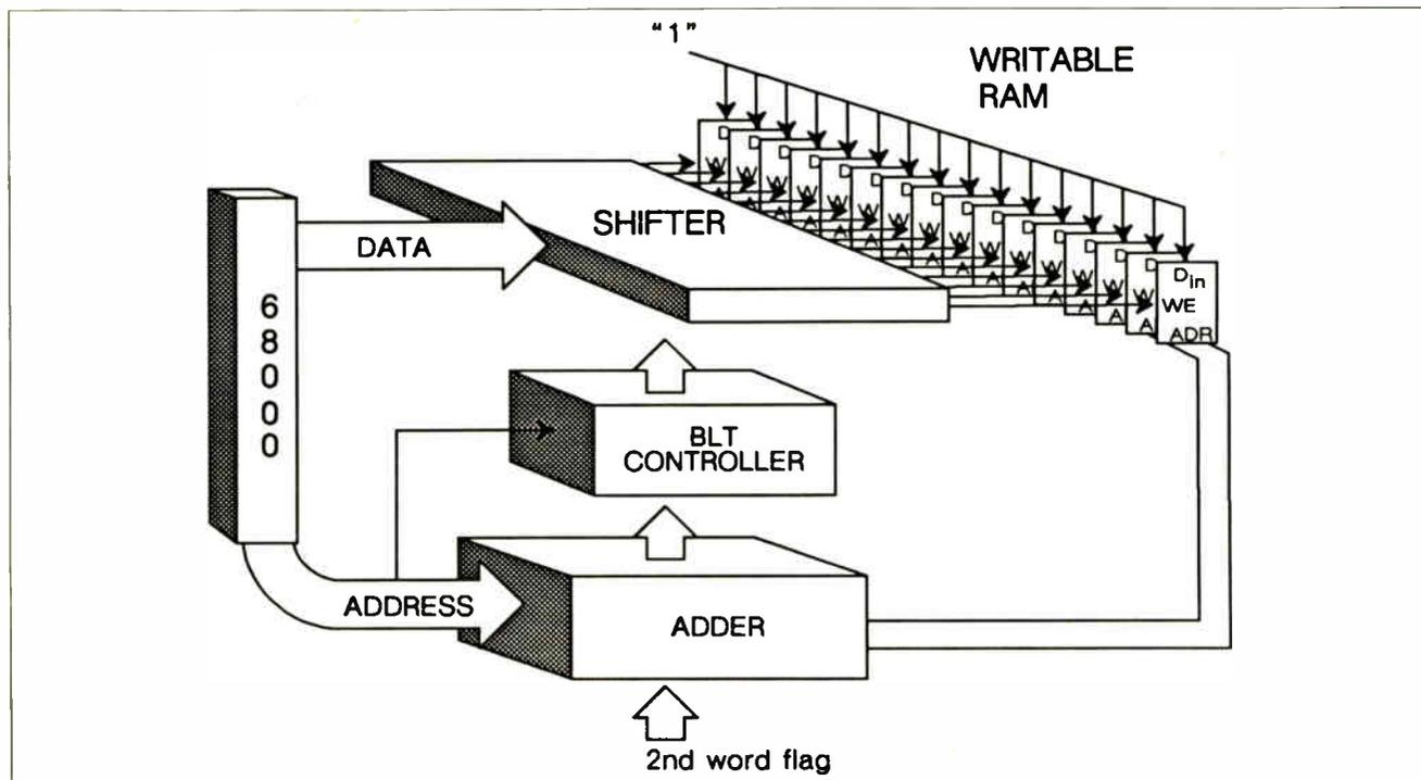
**Figure 5:** The most significant flags blit mode. Data is shifted and sent to the write-enable pin of the dynamic RAMs. For the second word, the address is incremented. The result is a direct OR to memory in one cycle.
