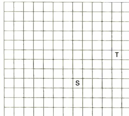
**Figure 3b:** The flag array is shown pictorially as the search algorithm proceeds during the solution of the problem in figure 4. S and T represent source and target. Unchecked cells are blank. The coordinates of the shaded cell are in the FIFO queue.
