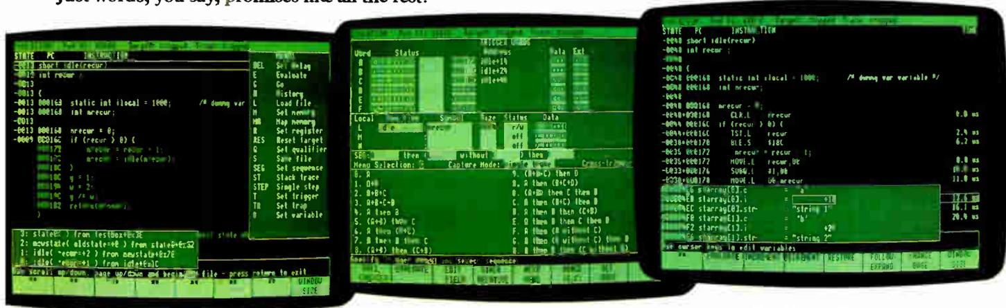
**Code Preview™** lets you see where your code is going. You can follow calls and branches (to 99 levels) on the screen, to select the source line on which to trigger, then set and break in one keystroke! The highlighted trace display (in source) and stack trace window show the path your program took.
