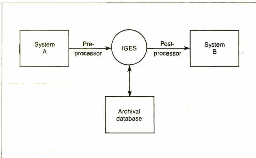
**Figure 3:** The software that translates from a CAD system to IGES is called a preprocessor. The software that goes the other way (translates from IGES to a CAD system) is called a postprocessor.
