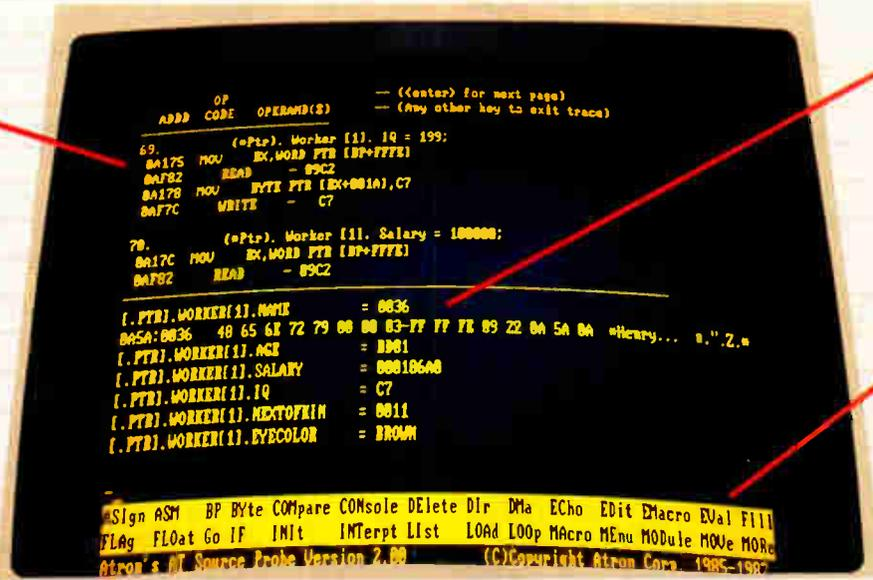
PROBE knows all about your local and complex variables. You can display and change an array of structures as easily as shown in this display.
