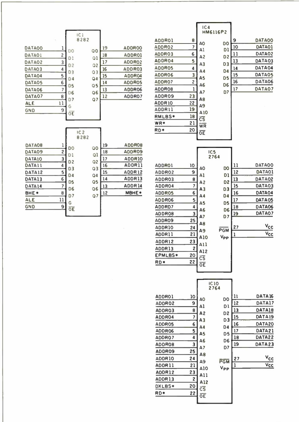
**Figure 5:** A CAD compiler schematic with each device shown separately, along with the signal names listed next to their corresponding pins.
