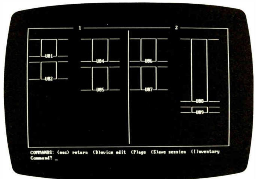
Figure 4: A CADcompiler completed entry form, showing the currently assigned signal names on the corresponding pins.
