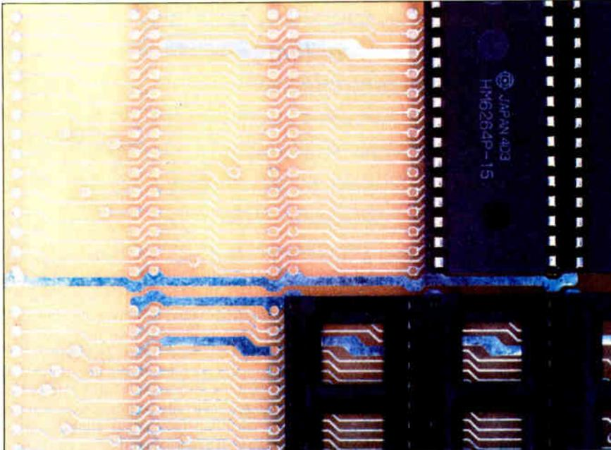
**Photo 1:** A portion of a Wintek printed circuit board, showing the insulating substrate, copper traces, and components. The copper conductors have been covered with solder, giving them a silver color.
