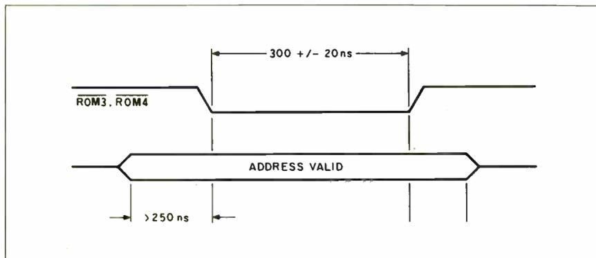
Figure 2: Cartridge-port address timing.
