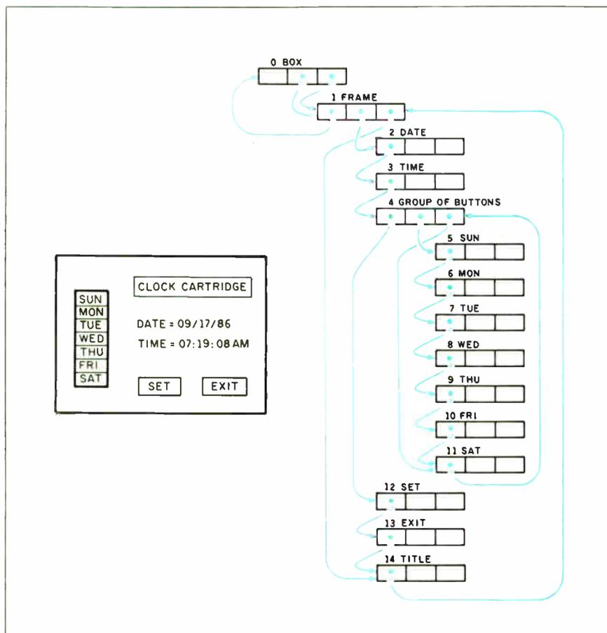
**Figure 5:** The dialog box for CLOCKSET.ASM and the linkage between objects. The first object (0) is the root object, and object 1 is its offspring, or sibling. Object 1 is the parent of objects 2, 3, and 4. Object 4 is the parent of objects 5 through 11.
