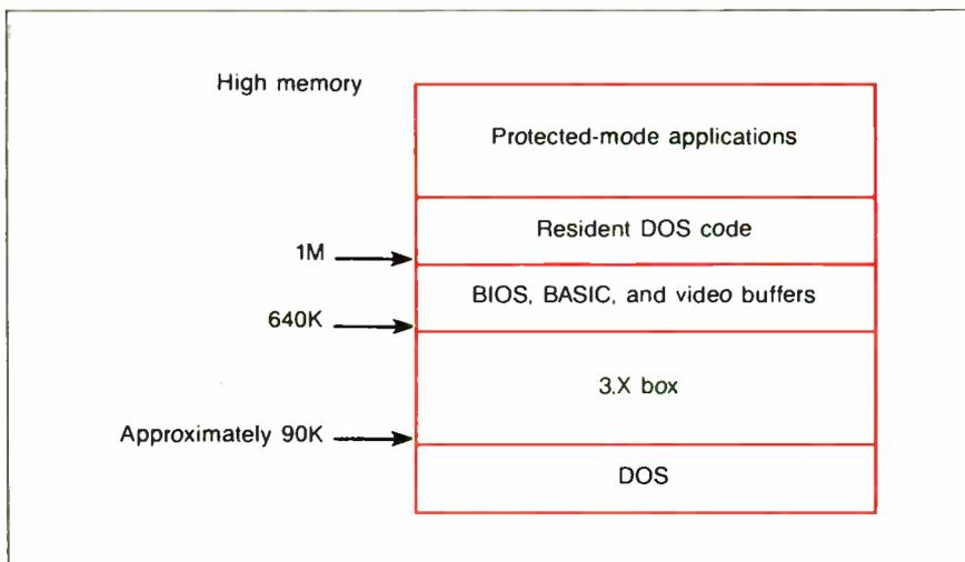
**Figure 1:** A memory map of OS/2. This figure shows a system configured for both protected- and real-mode applications. You can set up an OS/2 system for protected-mode tasks only, in which case the 3.X box disappears and protected-mode applications can use its memory. Also, you can adjust the 640K boundary at the top of the 3.X box to some lower value, freeing the memory between it and the BIOS area for use by protected-mode tasks.
