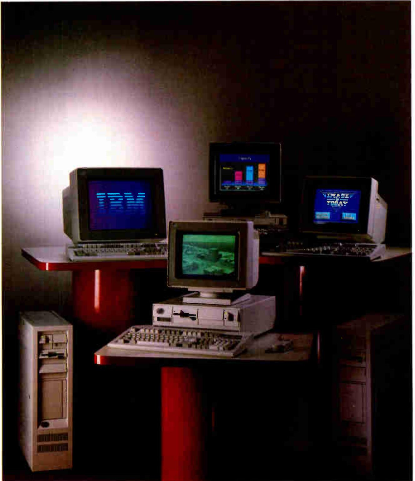
Channel bus. The Model 50, however, is a small-footprint desktop system with three open expansion slots, while the Model 60 is a larger, floor-standing "deskside" system with seven available expansion slots.
