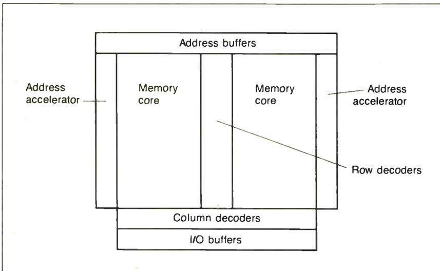
Figure 1: A floorplan for a RAM chip.
