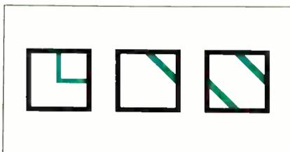
Figure 6: Replacing an L-shaped trace in a cell with a diagonal trace allows the smooth construction of 45-degree traces. Using a double-diagonal cell allows two conductors to occupy one cell.
