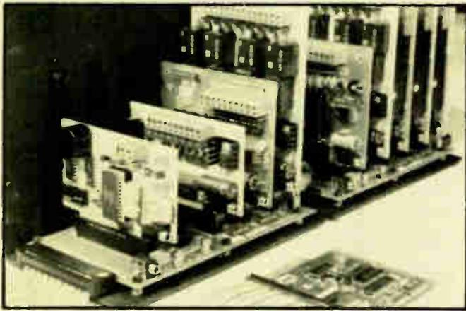
An A-BUS system with two Motherboards
