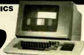
The Leas Sieglar 7107 color graphics terminal is both DEC (VT-100 / VT-51) and Tektronix (4010/4014) compatible. The terminal offers a palette of 4,096 colors with a resolution of 640 by 480 pixels on a 13 inch non-glare black screen. Horizontal pan and image zoom, to 16 times original size, are standard features of this color graphics terminal. The 7107 is the ideal terminal for CAD/CAM applications.
