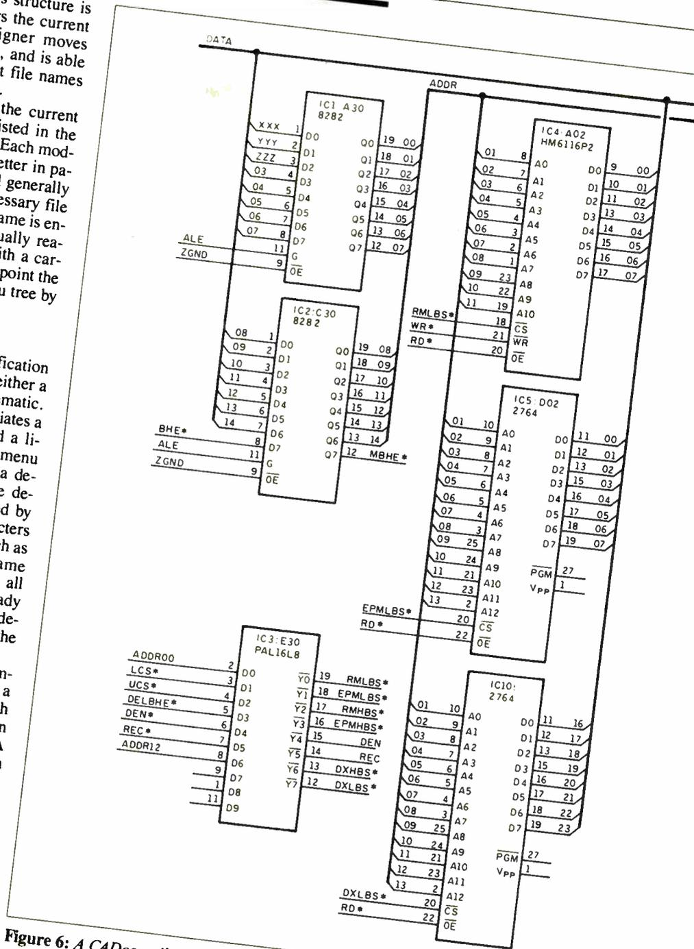
Figure 6: A CAD compiler finished drawing, showing the added data bus lines.
