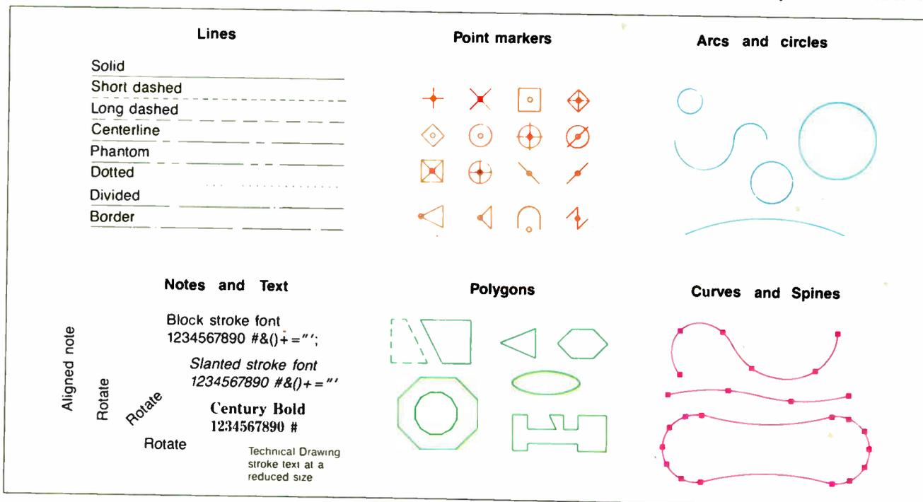
Figure 1: The typical graphics primitives used by standard CAD programs.
