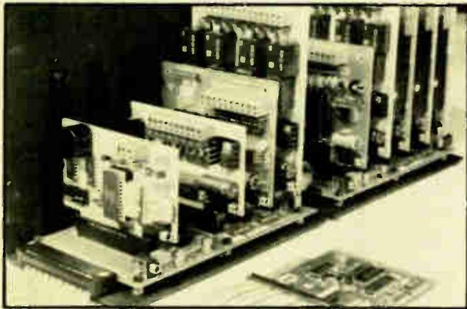
An A-BUS system with two Motherboards
