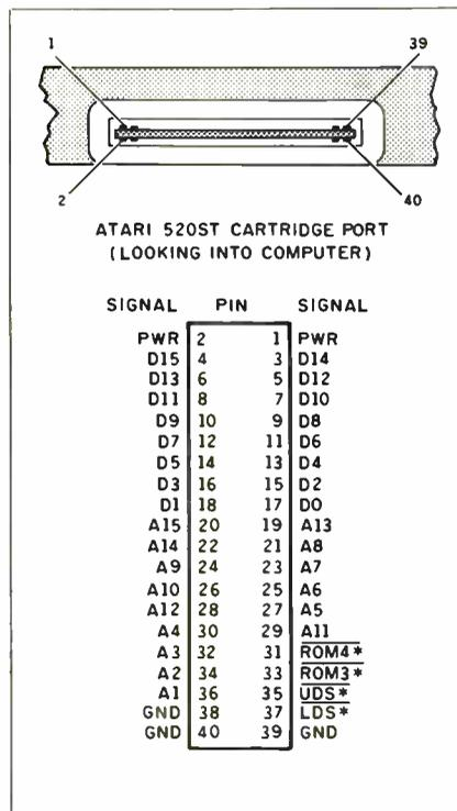
**Figure 1:** The Atari cartridge port and signals.
