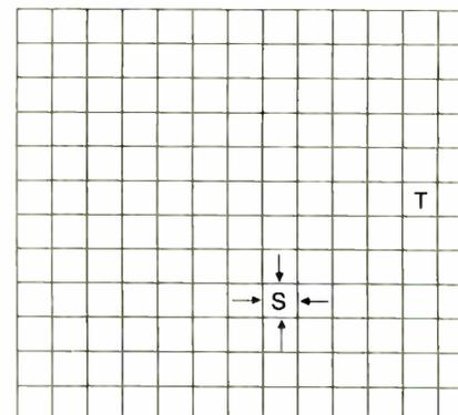
**Figure 3c:** After following steps 4 through 9 once, the flag array now has four additional entries, and four sets of coordinates are in the FIFO queue. The arrows are used to represent the values north, east, south, and west.
