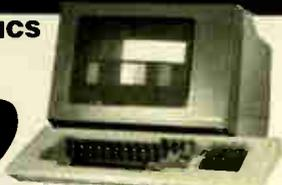
The Leas Sieglar 7107 color graphics terminal is both DEC (VT-100 / VT-51) and Tektronix (4010/4014) compatible. The terminal offers a palette of 4,096 colors with a resolution of 640 by 480 pixels on a 13 inch non-glare black screen. Horizontal pan and image zoom, to 16 times original size, are standard features of this color graphics terminal. The 7107 is the ideal terminal for CAD/CAM applications.
