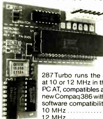
287 Turbo runs the 80287 at 10 or 12 MHz in the IBM PC AT, compatibles and the new Compaq 386 with 100% software compatibility.
