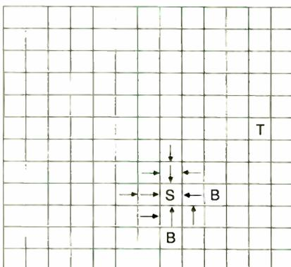
**Figure 3d:** The diamond-shaped search wavefront is a characteristic of Lee's Algorithm. By this point in the search, two cells that already contain traces have been found and have been marked as blocked.
