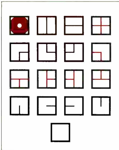
**Figure 2:** All of the possible cell contents for the basic Lee's Algorithm. Component leads are normally soldered to pads (the circular conductor, also called vias); most traces will start and end at a pad. Pads may be used to connect traces on two different layers.
