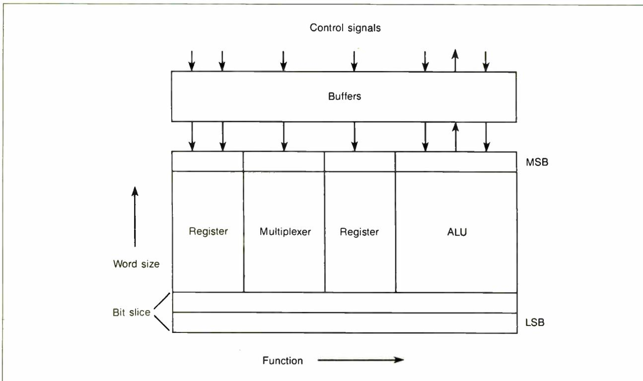
Figure 4: The floorplan used by a silicon compiler for a datapath component.
