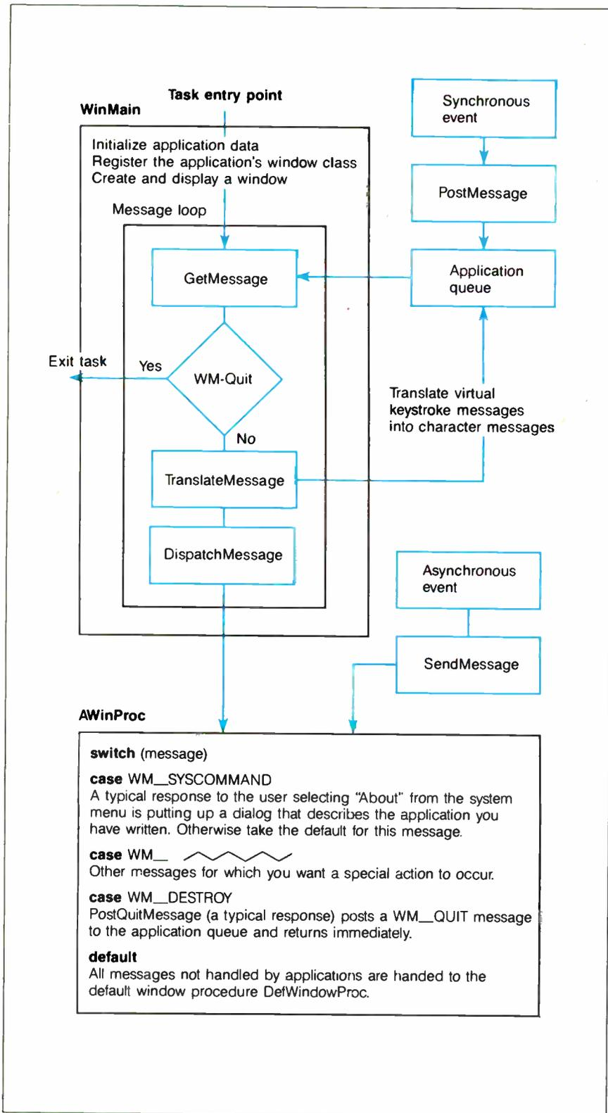
**Figure 2:** Every Windows application must have a `WinMain` procedure, which serves as the entry point to the task. `WinMain` sets the stage for the application and then supervises the removal of messages from the application queue and the distribution of messages among the application's windows. `PostMessage` returns without waiting for the corresponding window to process the message; `SendMessage` doesn't return until the message has been processed.
