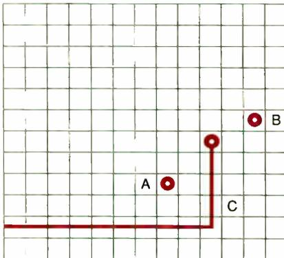
**Figure 3a:** An example of using Lee's Algorithm to find a path from pad A to pad B. Trace C blocks the most direct route.
