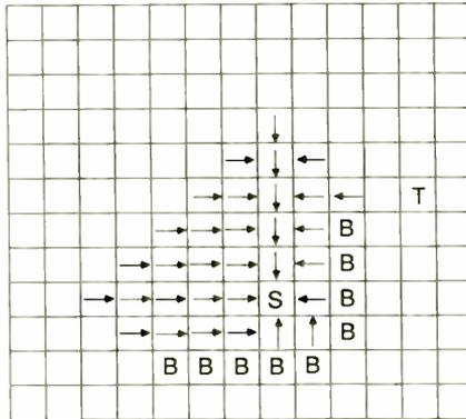
**Figure 3g:** The algorithm has now found a path to the east again, passing over the upper end of trace C. There are now nine sets of coordinates in the FIFO queue.
