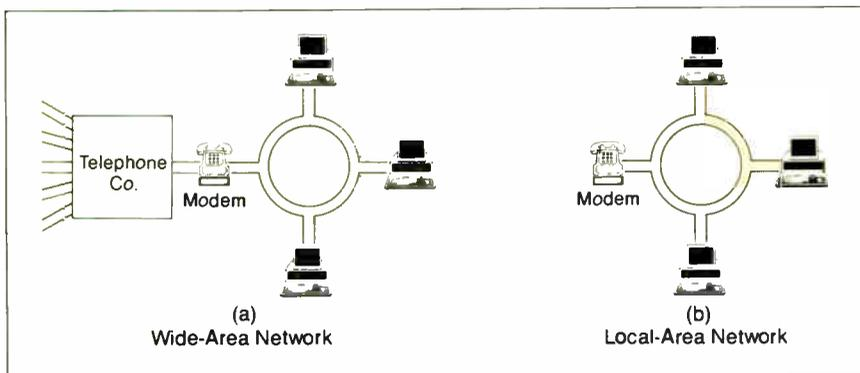
**Figure 2: WAN-centered (a) and LAN-centered (b) viewpoints.** Although the phone system (a) does not qualify as a LAN, the system of devices (b) up to and including the modem might qualify (such as a token-ring network with a modem connection for communication with a branch office).
