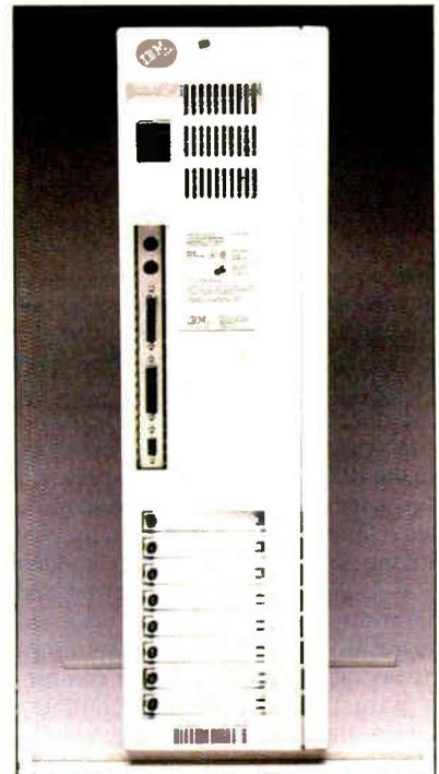
**Photo C:** The rear of the Model 60, showing the connectors for the keyboard, mouse, serial port, parallel port, and video monitor.
