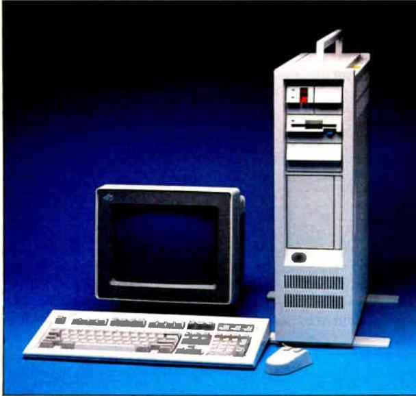
**Photo A:** The Model 60 with the 8503 monochrome monitor. The Model 60 is much larger than the Model 50; in fact, it stands on the floor beside your desk.
