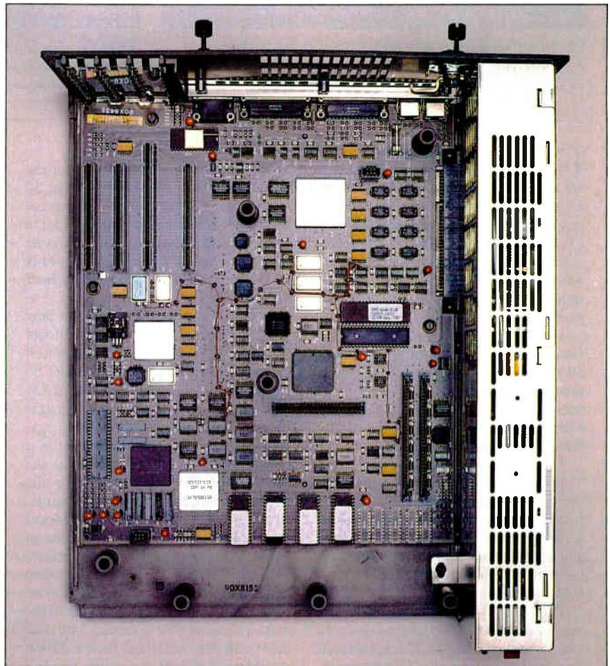
**Photo 3:** The interior of the Model 50. The power supply runs along the right side of the machine, the system RAM is just to the left, and the 80286 is on the left toward the front of the machine. The four Micro Channel slots are in the left rear of the machine.
