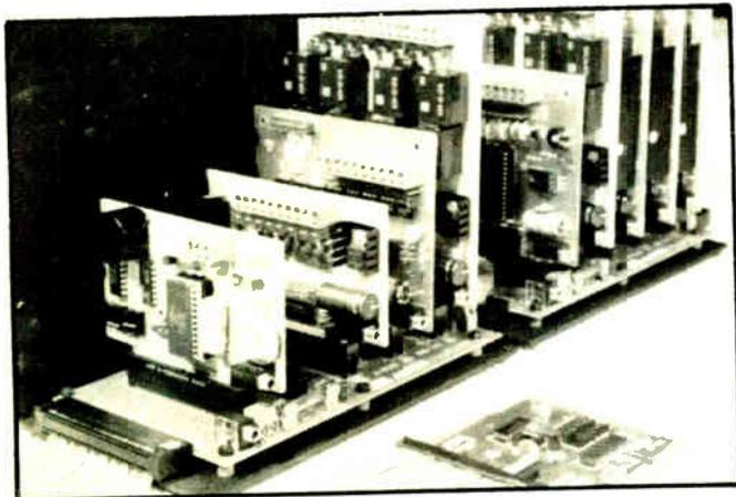
An A-BUS system with two Motherboards
