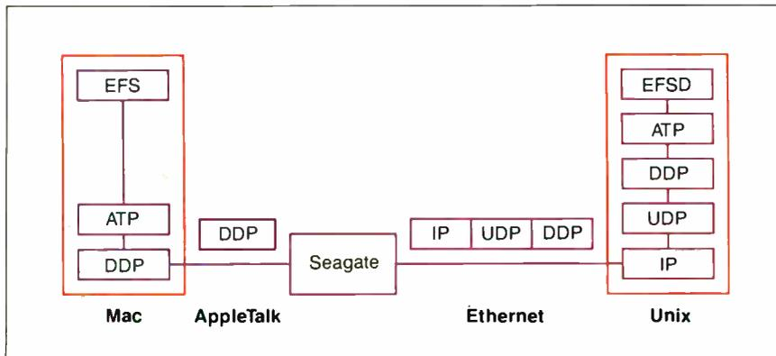
Figure 1a: Exchanging AppleTalk data packets through Seagate.
