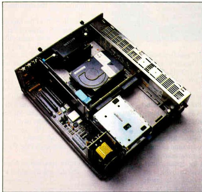
**Photo 1:** The Model 50 with its housing off. Notice how the hard disk (in the center of the machine) plugs directly into its controller board.
