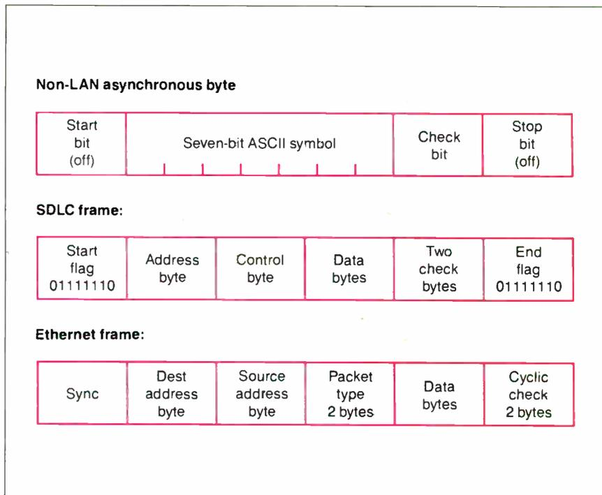
Figure 3: Three of the standard packet formats used for digital communications.
