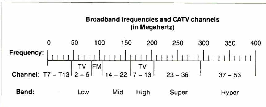
Figure 4: Spectrum of frequencies allocated for broadband transmission.
