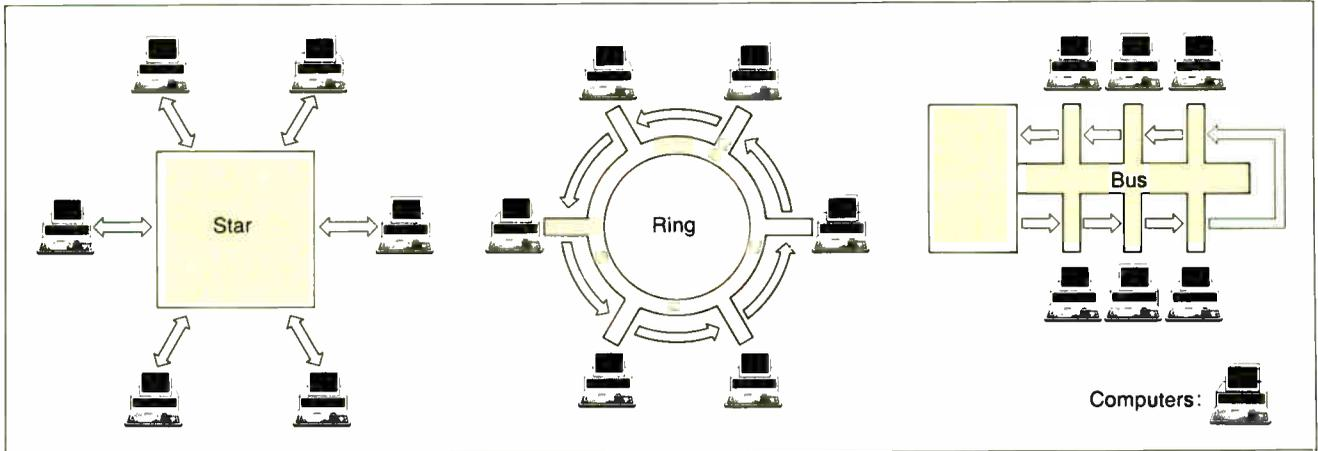
**Figure 1: Network topologies.** In a star configuration, outlying stations communicate through a central hub device. In a ring network, messages circulate the loop, passing from station to station in bucket-brigade fashion. Stations on a bus network send data to a head-end retransmitter that rebroadcasts the information back to the bus.
