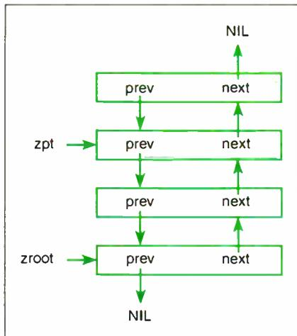
Figure 1: Typical stack structure.
