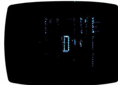
**Photo 7:** Here, I use the Thresh program to remove background noise from the image in photo 6b. The missing IC in 5b now stands out clearly.
