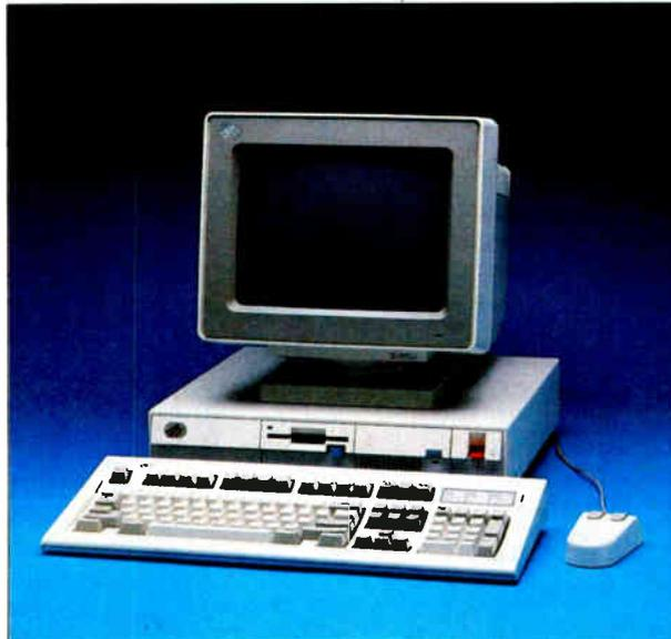
motherboard. The MCGA will automatically emulate the old CGA standard for programs that call for it. The MCGA does not provide compatibility with the Enhanced Graphics Adapter (EGA) standard, but it provides a greater number of colors and higher resolution than the CGA. EGA compatibility will be available from IBM with the addition of the PS/2 display adapter, which was announced for availability sometime this month. The Model 30 is not compatible
