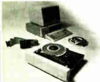
For information interchange, backup and archival storage, IBEX offers a 9-track IBM format compatible magnetic tape subsystem for the IBM PC, featuring:
