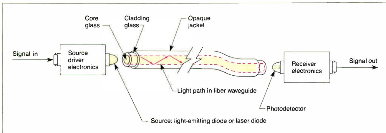
Figure 6: Basic optical-fiber communications link.
