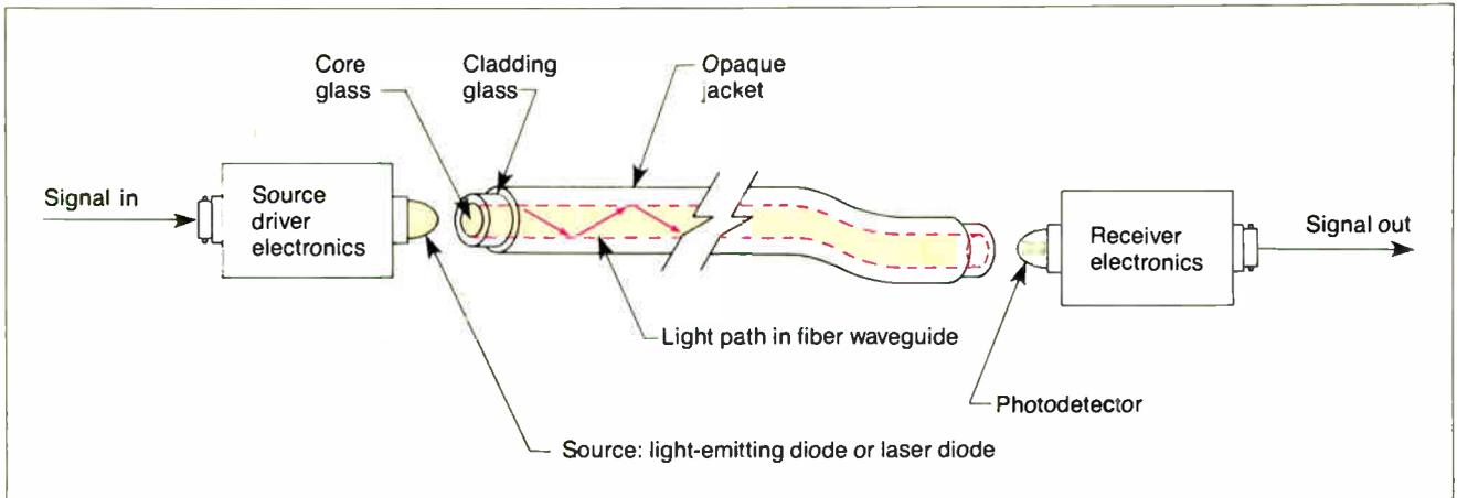
Figure 6: Basic optical-fiber communications link.
