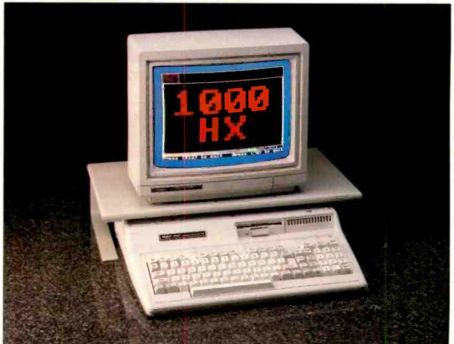
Photo 4: The Tandy 1000 HX, an 8088-based machine with MS-DOS in ROM.
