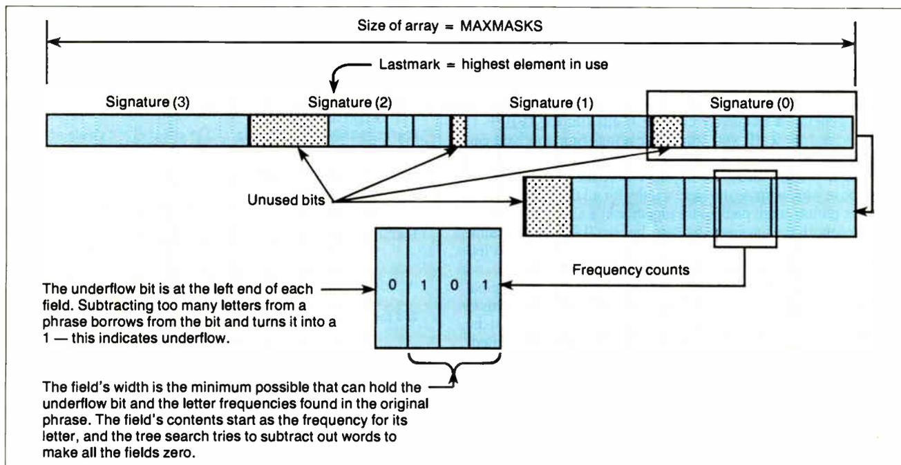
▲ **Figure 2:** The "bit signature" data structure. This is a collection of fields, each holding the frequency of a given letter and an underflow bit. To simplify the algorithm (and to allow the use of arithmetic subtraction to do the subtraction of signatures), the author designed the structure so that frequency-count fields do not cross physical boundaries—longwords, in this case.
