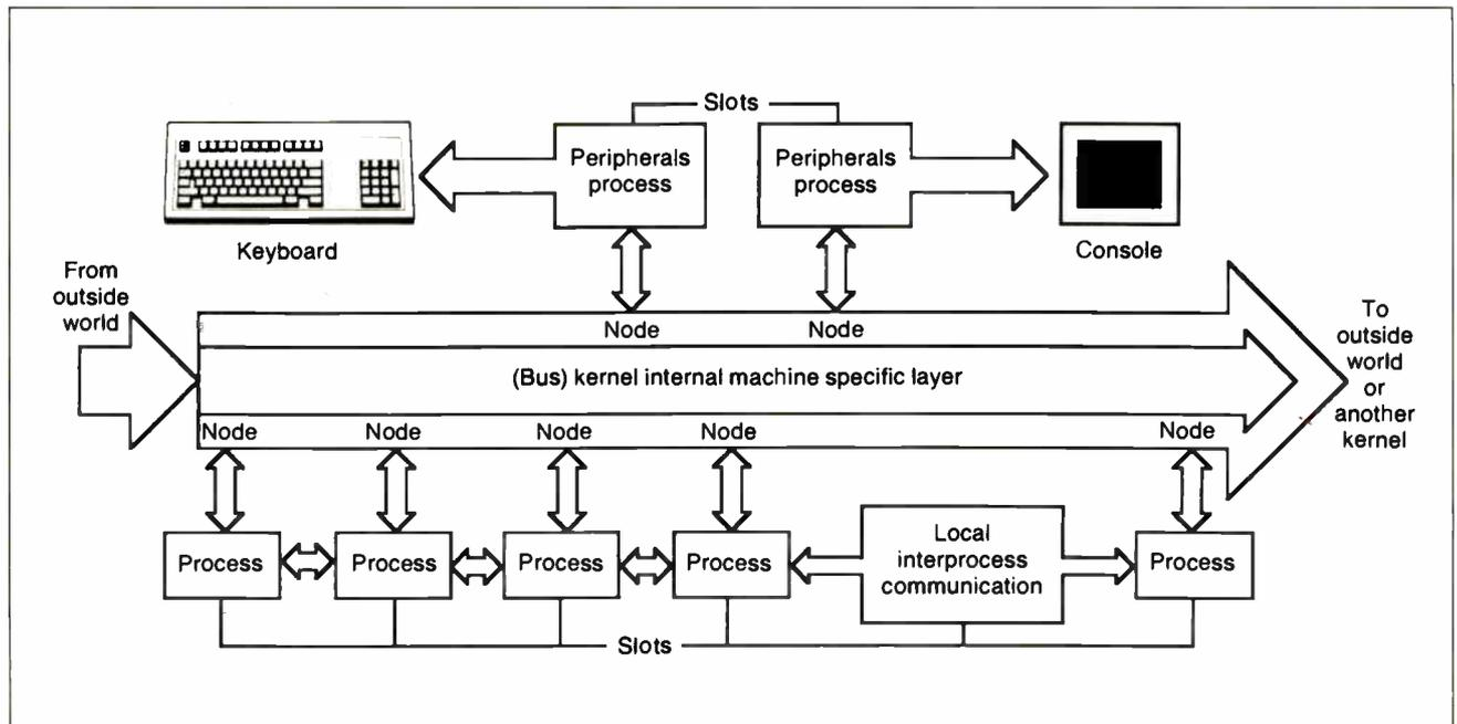
Figure 4: A block diagram of the architecture of the V operating system.
