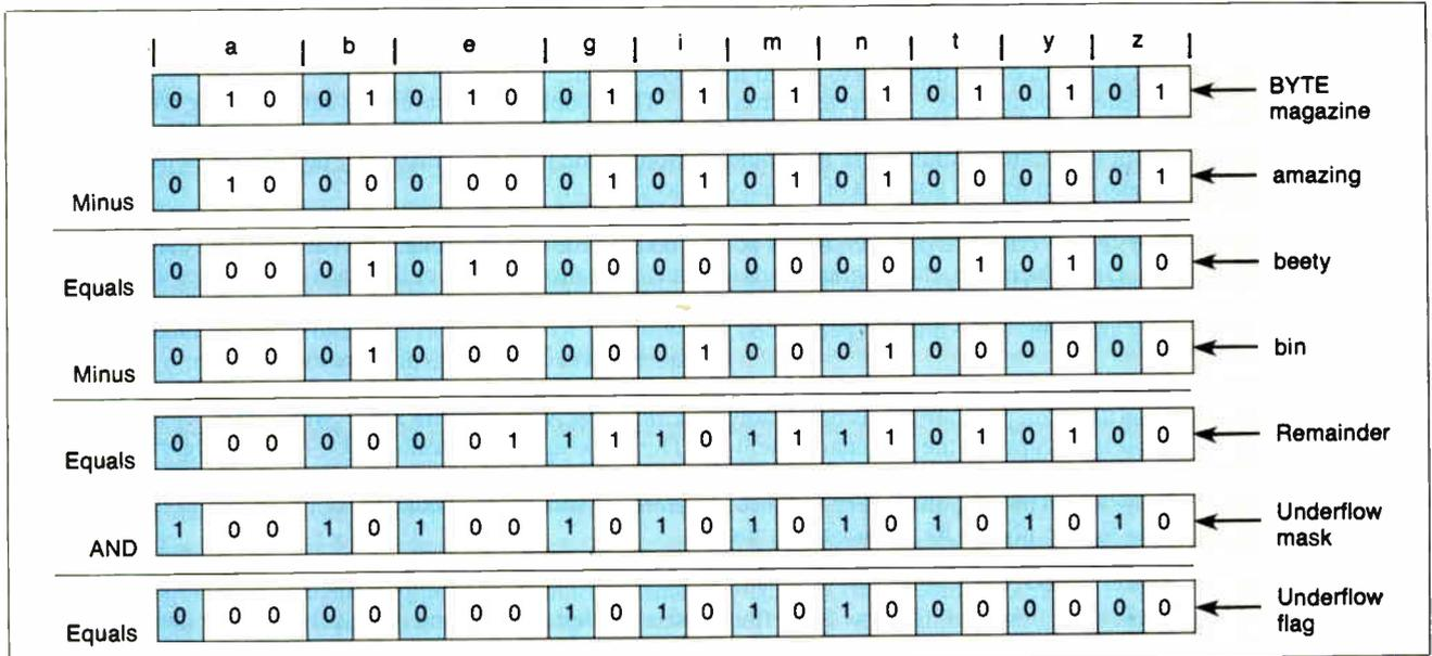
**Figure 1: Subtracting signature bytes to determine if a given word is contained in a given letter set. Rows 1 through 3 show how the word amazing can be subtracted from the letters in the phrase BYTE magazine to give beety. Variable-length fields with an underflow bit at the left end of each one represent the letters in the phrase. We know the subtraction is valid because all the underflow bits (shaded) in the result are zero. Rows 3 through 7 show what happens**
