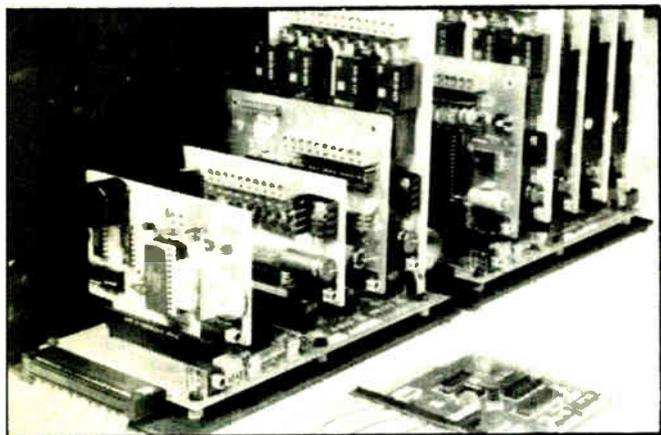
An A-BUS system with two Motherboards
