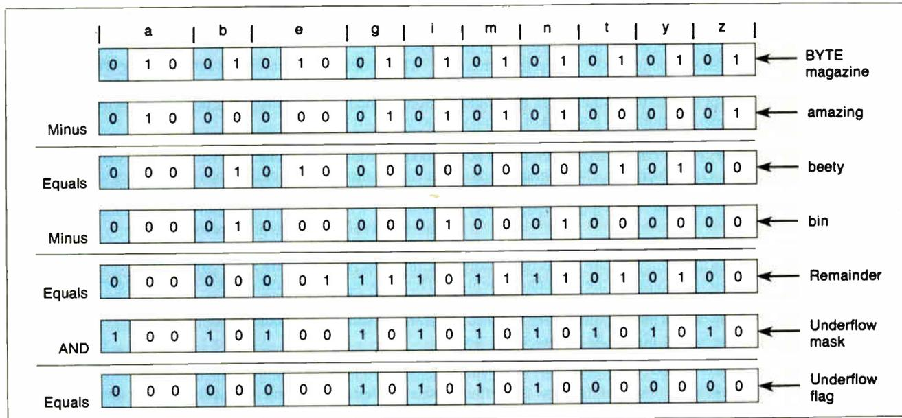
**Figure 1: Subtracting signature bytes to determine if a given word is contained in a given letter set. Rows 1 through 3 show how the word amazing can be subtracted from the letters in the phrase BYTE magazine to give beety. Variable-length fields with an underflow bit at the left end of each one represent the letters in the phrase. We know the subtraction is valid because all the underflow bits (shaded) in the result are zero. Rows 3 through 7 show what happens**
