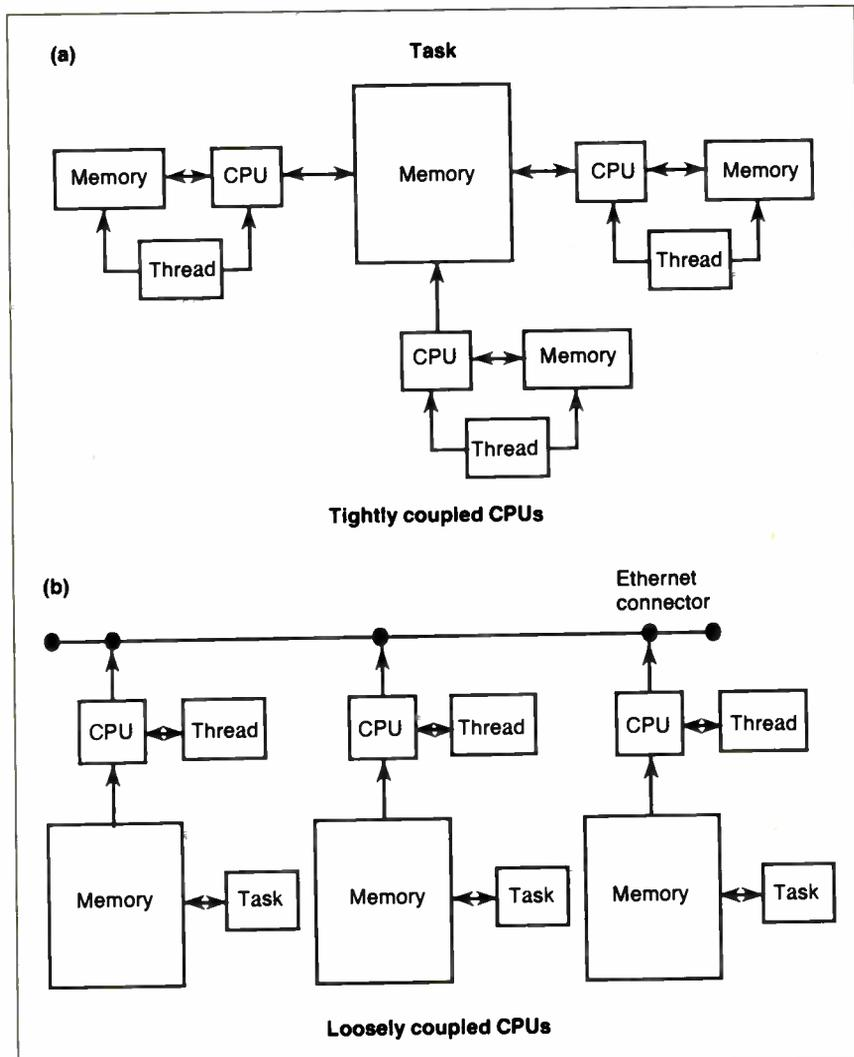
Figure 1: The relationship of tasks, threads, and CPU configurations.
