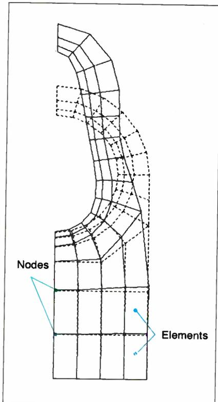
**Figure 1:** A half-symmetry finite-element model of a steel lifting lug, used for lifting pressure vessels and other heavy objects, generated in MSC/pal 2.
