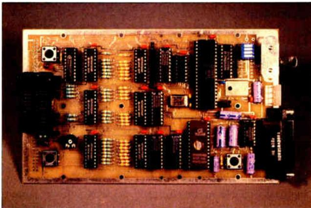
**Photo 1:** The prototype IC tester printed circuit board configured for terminal operation. The IC under test is inserted into a special zero-insertion-force socket on the left side, and test information and menu selections are displayed on a terminal connected through the DB-25 connector on the right side.
