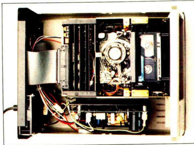
The VAST device uses VCR-like technology to back up data.
