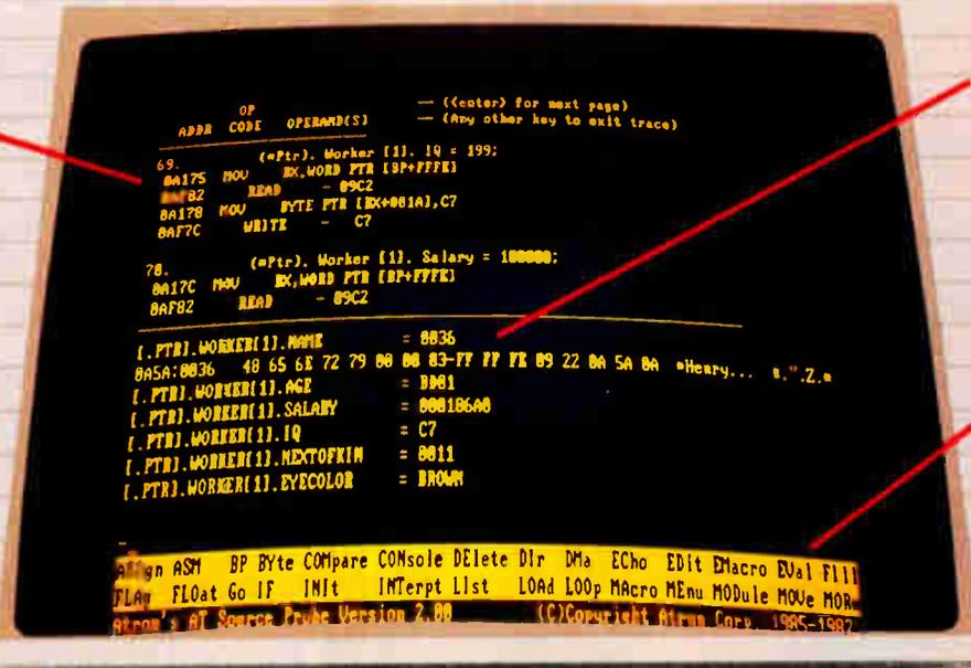
PROBE knows all about your local and complex variables. You can display and change an array of structures as easily as shown in this display.
