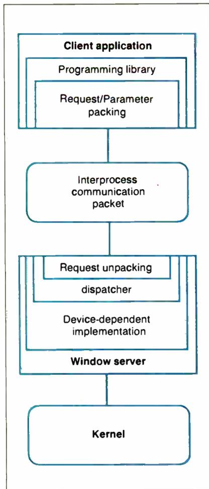
**Figure 2: Client-server relationship.** The window server manages all interaction with the display device and the input devices. Clients are user applications that request services from the server through the window programming library.
