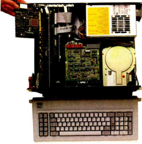
*High-tech. Open your PC and slide the controller board into any expansion slot. Low-tech. Hook up VCR to computer with standard connector cables.*
