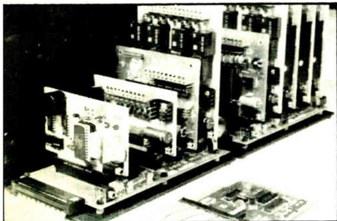
An A-BUS system with two Motherboards
