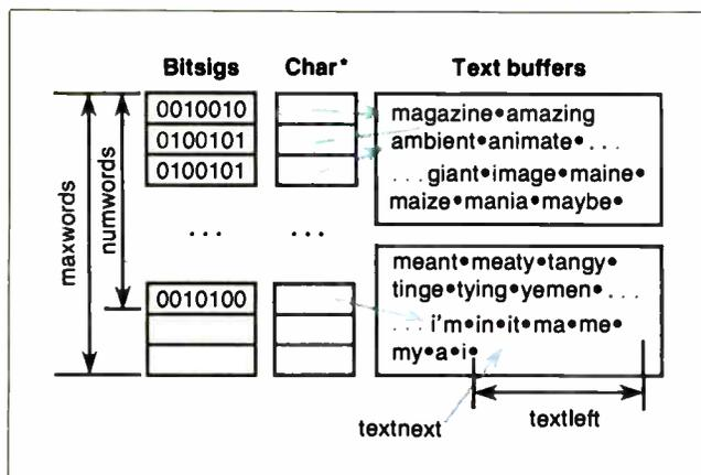
◀ **Figure 3:** Storing candidate words for easy use during the anagram search. The search needs both the bit signature and text for each word. These are kept in parallel arrays; both the maximum length and used length of the arrays are remembered. The variables numwords and maxwords keep track of the number of entries left in the two arrays, while textnext and textleft do the same for the text buffer area.
